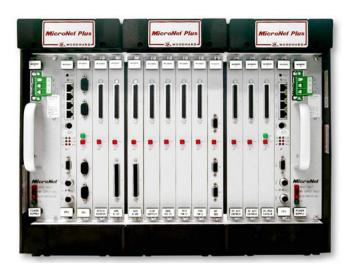
The program will maintain a qualified Micronet Test System that is capable of running final test routines on virtually all Woodward Micronet modules. These will be returned with a test sheet that shows the recorded data and test results. Cleaning of Micronet chassis, cards and replacing ventilators are all part of this service.
