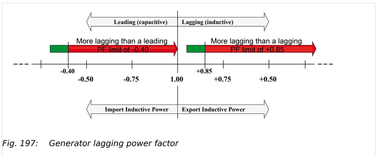
Fig. 197: Generator lagging power factor
