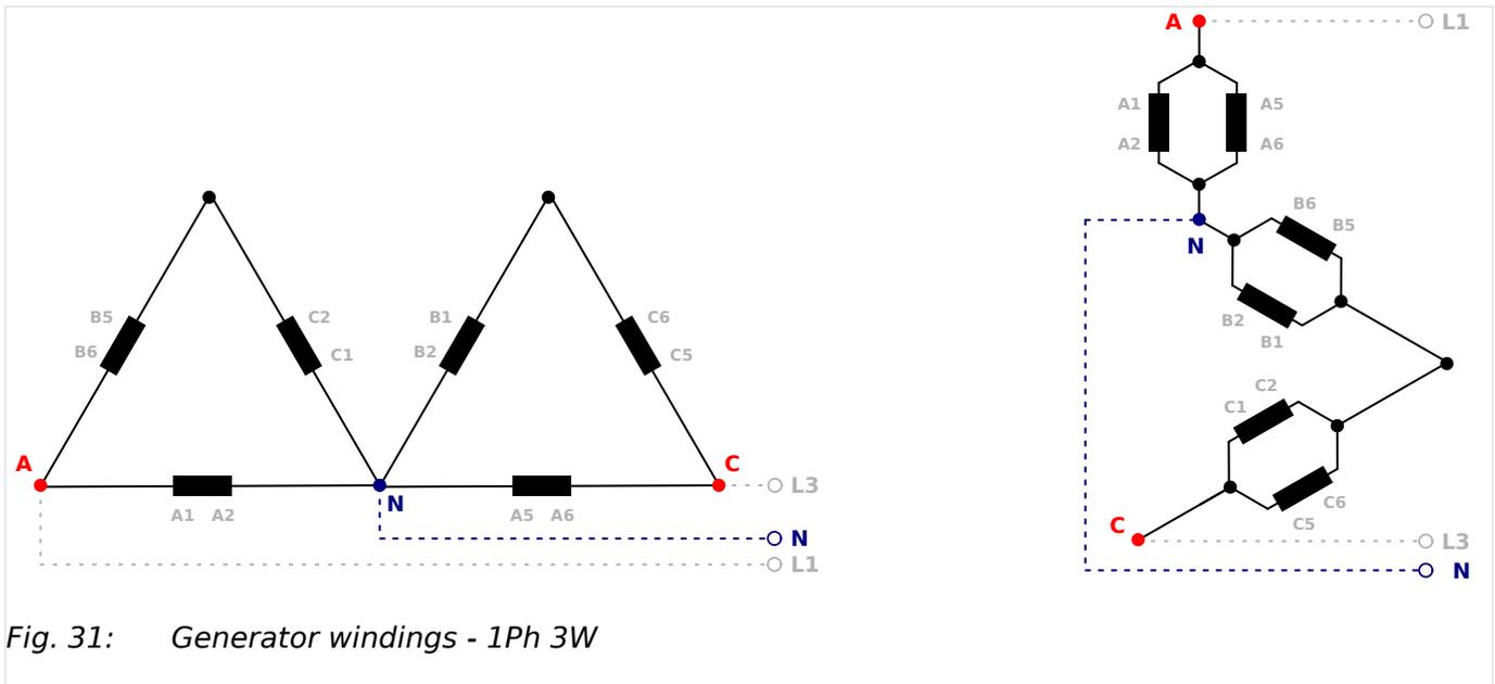
Fig. 31: Generator windings - 1Ph 3W
