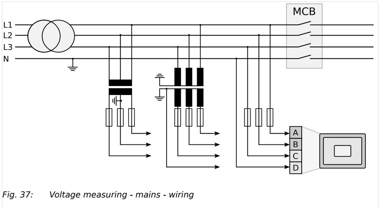
Fig. 37: Voltage measuring - mains - wiring
