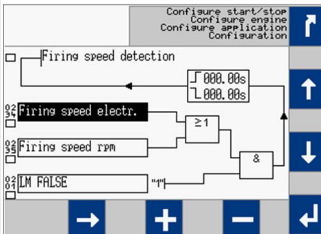
Fig. 151: LogicsManager Firing speed detection
