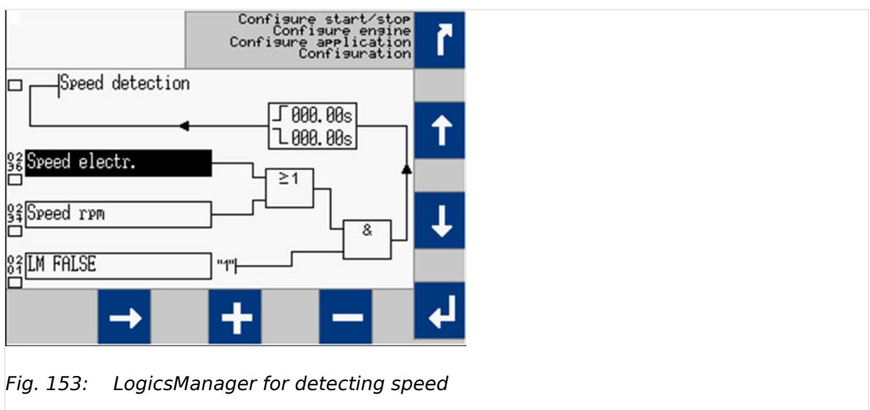
Fig. 153: LogicsManager for detecting speed
