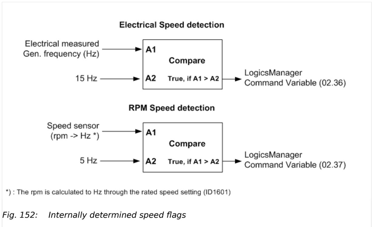
Fig. 152: Internally determined speed flags
