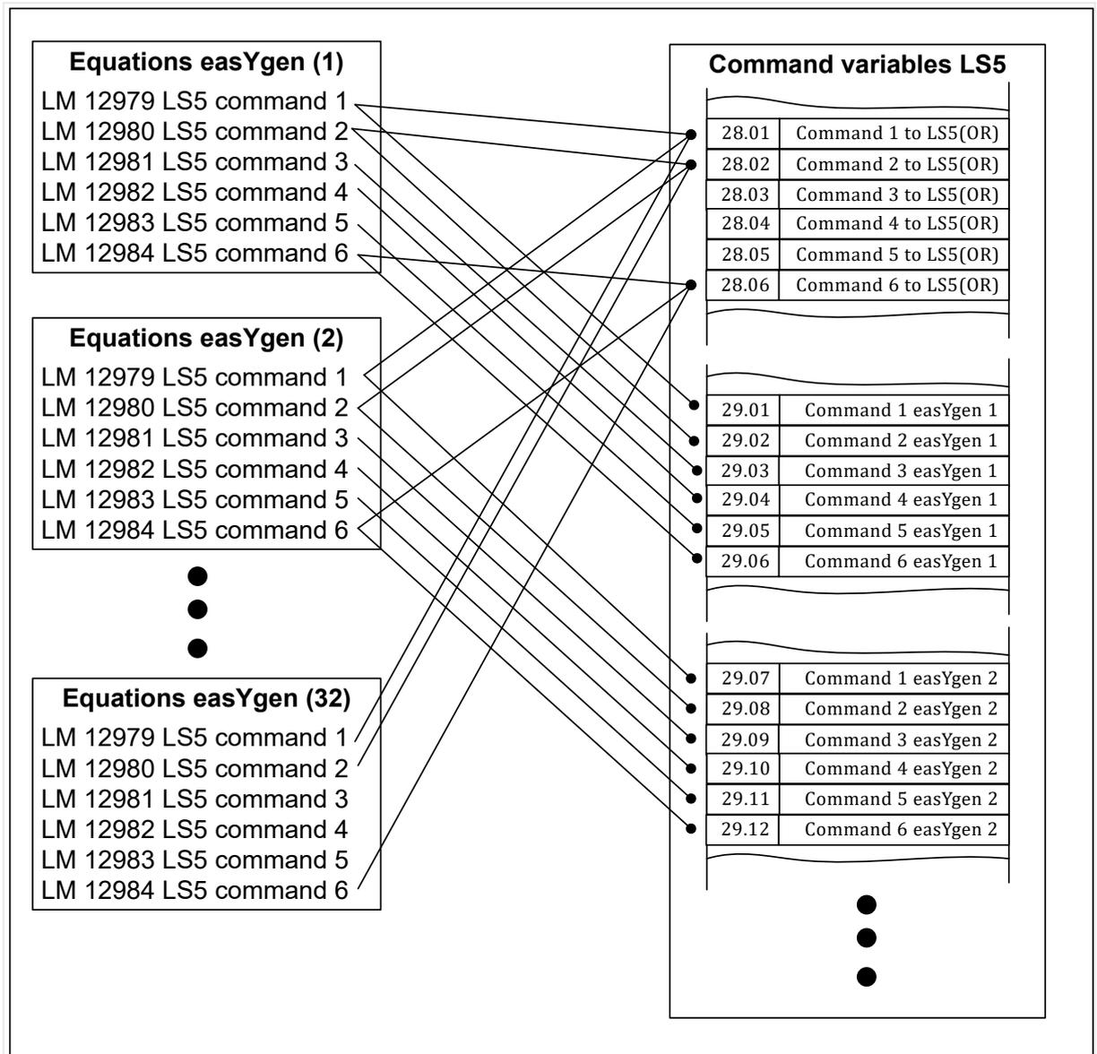
Fig. 221: LM flags of easYgen transferred to LS-5 (LSx)
