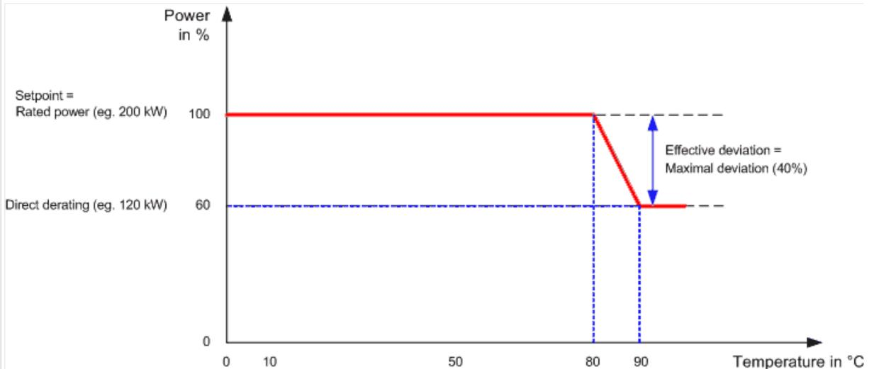
Fig. 313: Derating: Mains parallel operation; setpoint = rated power
