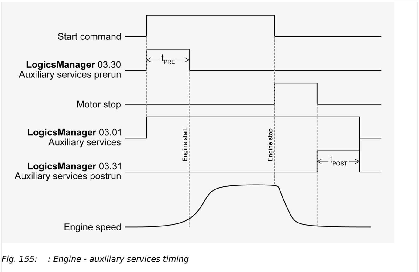
Fig. 155: : Engine - auxiliary services timing
