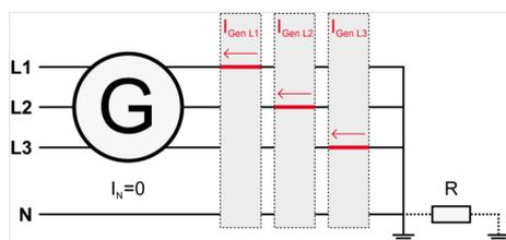
Fig. 199: Generator ground fault - schematic
