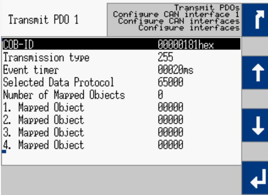
Fig. 266: TPDO configuration for IKD 1 (example HMI)
