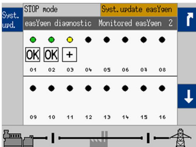
Fig. 245: Diagnostic screen example (HMI)
