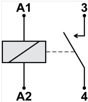
Fig. 163: Normally Open contacts - schematic
