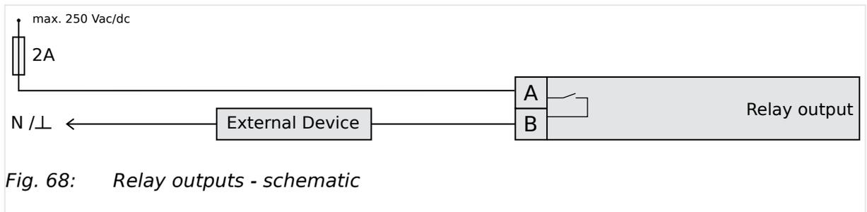
Fig. 68: Relay outputs - schematic
