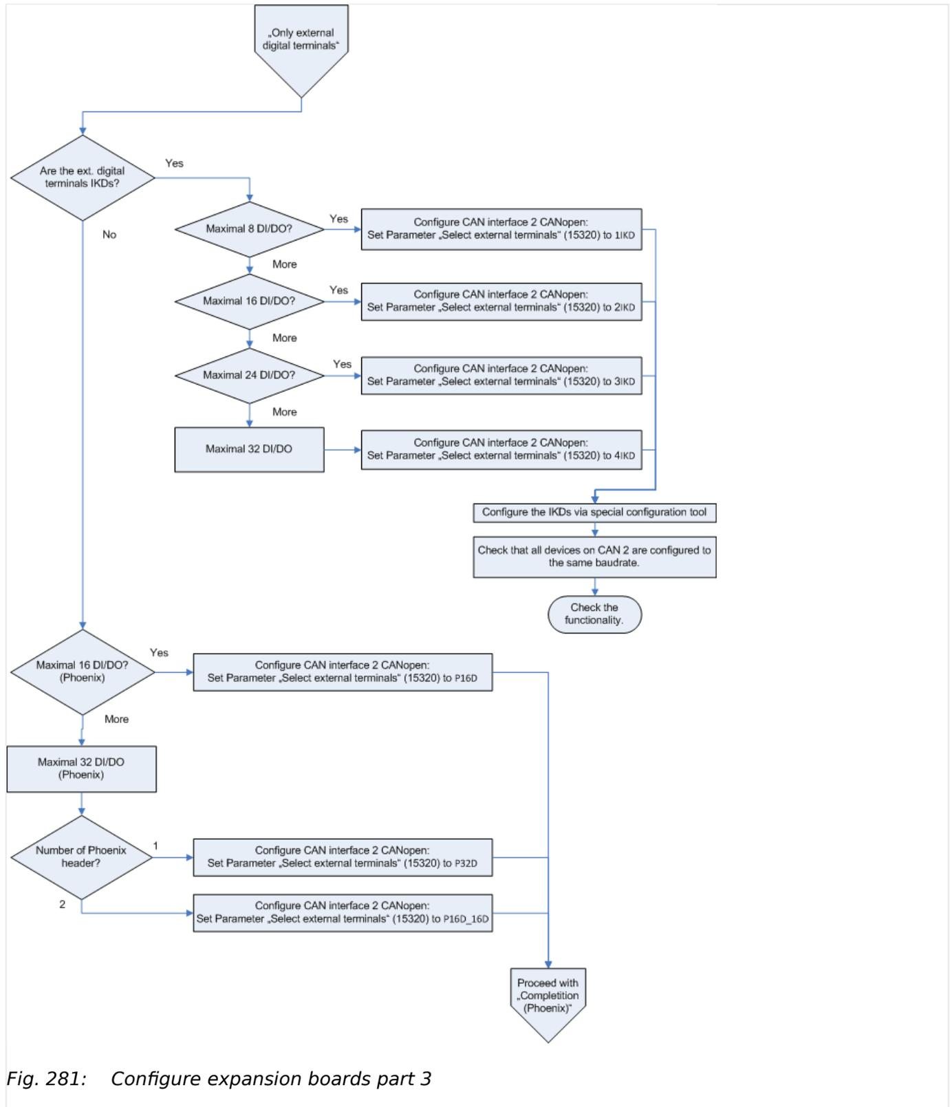
Fig. 281: Configure expansion boards part 3
