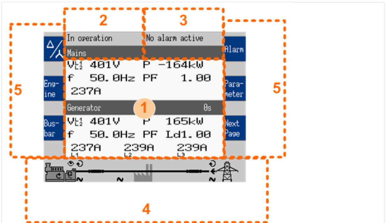
Fig. 86: Main screen (shown with default settings for screen configuration)
