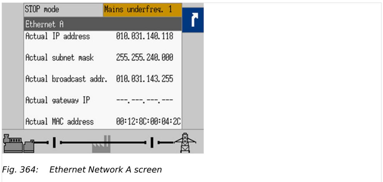
The actual IP address in Network A, subnet mask and gateway IP address can be viewed under Next Page (Status Menu) / Diagnostic / Interfaces / Ethernet / Ethernet A.
