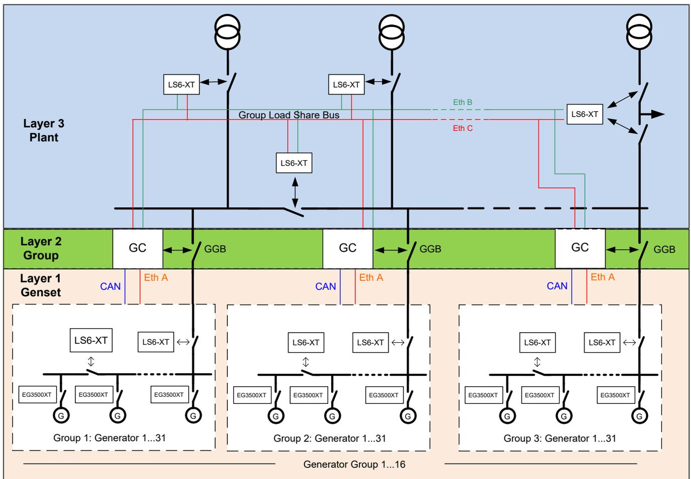
Fig. 240: Example application mode A13 with GC and LS-6XT
