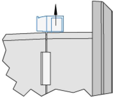
Fig. 11: Remove terminals
