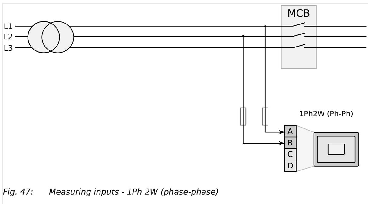
Fig. 47: Measuring inputs - 1Ph 2W (phase-phase)
