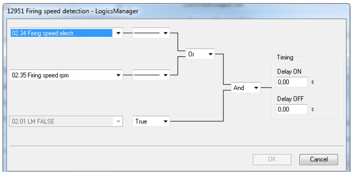
Fig. 286: LogicsManager function "Firing speed detection"
