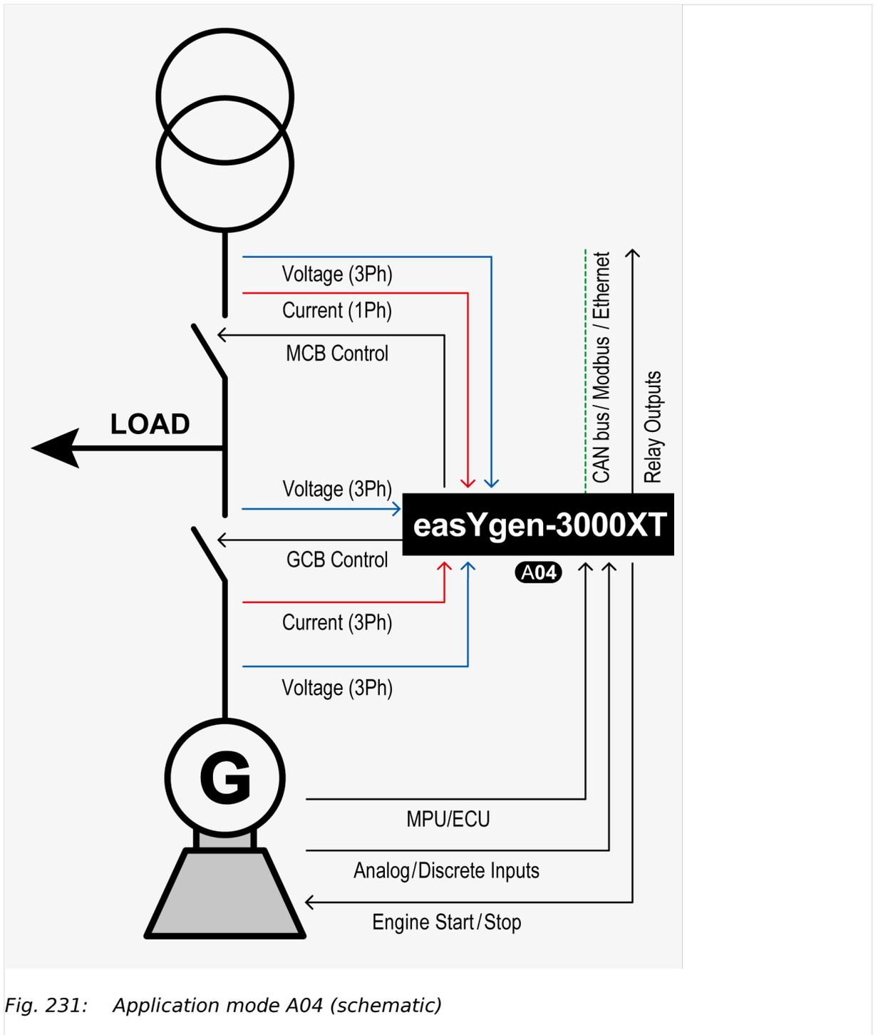
Fig. 231: Application mode A04 (schematic)
