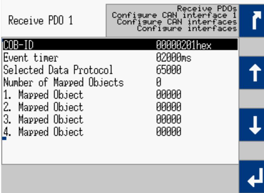
Fig. 268: RPDO configuration for IKD 1 (example HMI)
