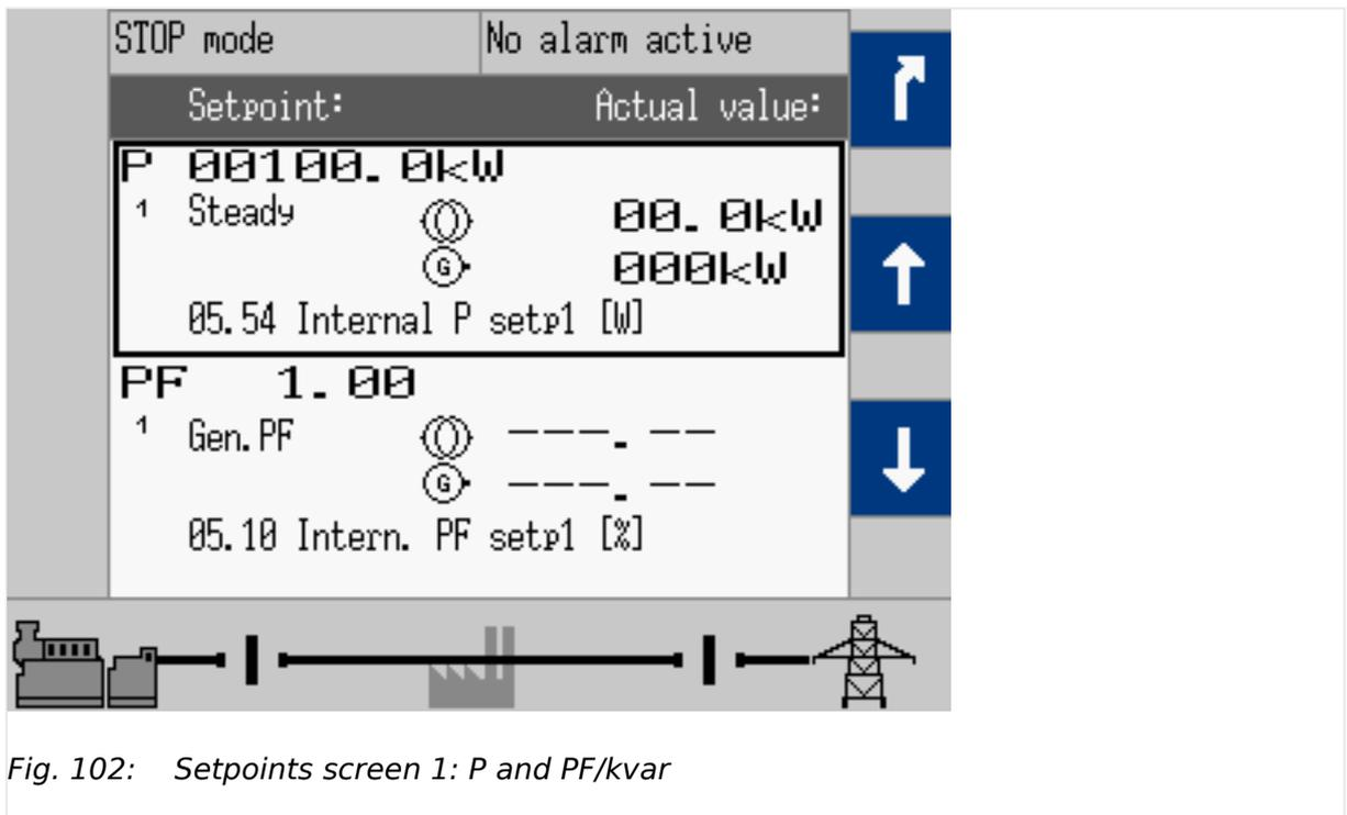
Fig. 102: Setpoints screen 1: P and PF/kvar
