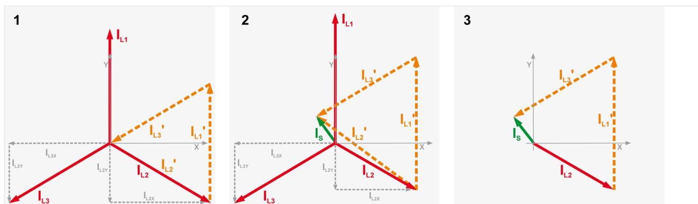
Fig. 200: Generator ground fault - calculation
