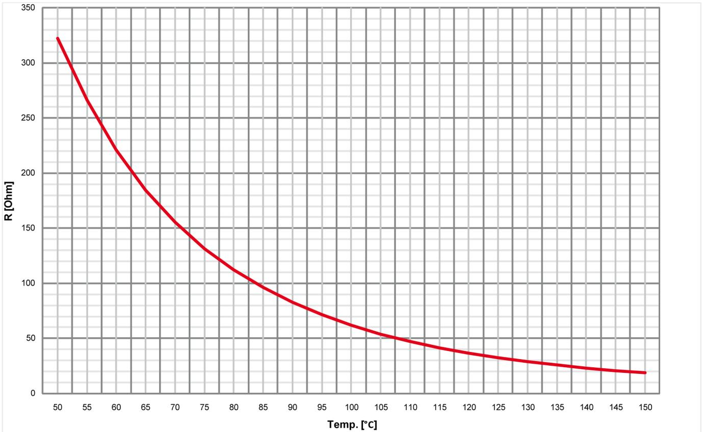
Fig. 383: Characteristics diagram VDO 50 to 150 °C - detail, Index "92-027-006"
