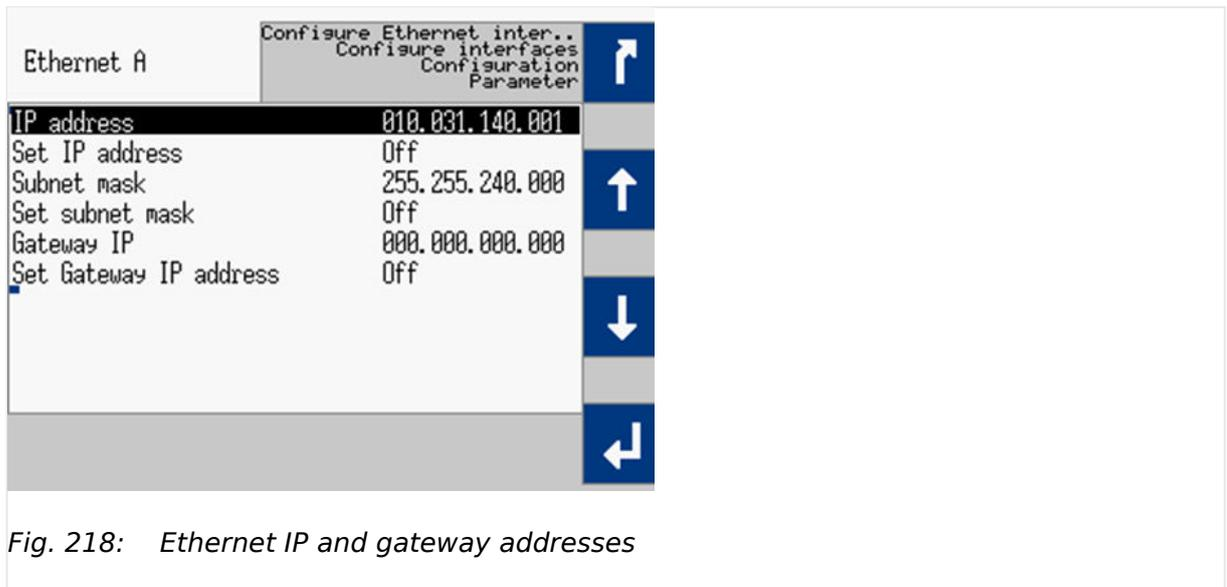
Fig. 218: Ethernet IP and gateway addresses
