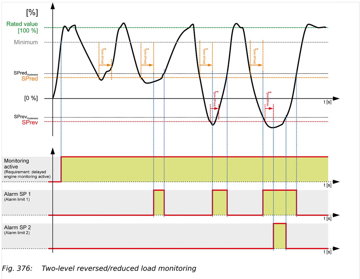
Fig. 376: Two-level reversed/reduced load monitoring
