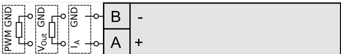
Fig. 71: Analog controller output - two wires
