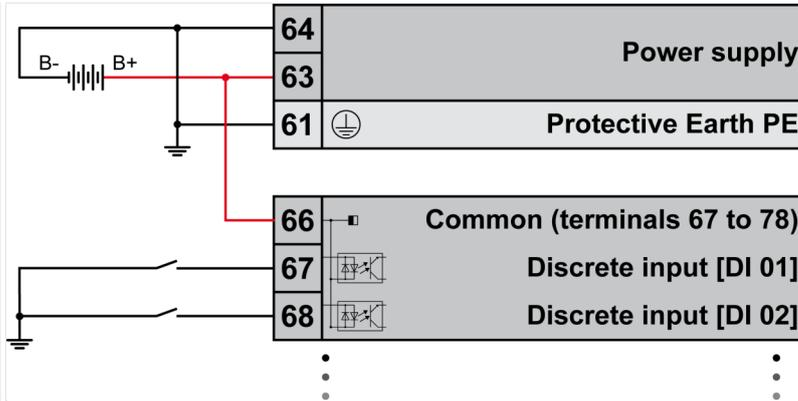
Fig. 276: Wiring self-powered discrete inputs
