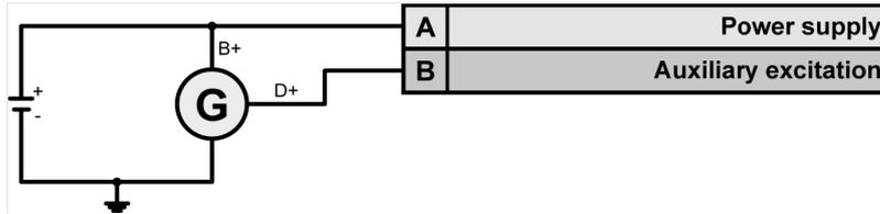
Fig. 23: Charging alternator - wiring
