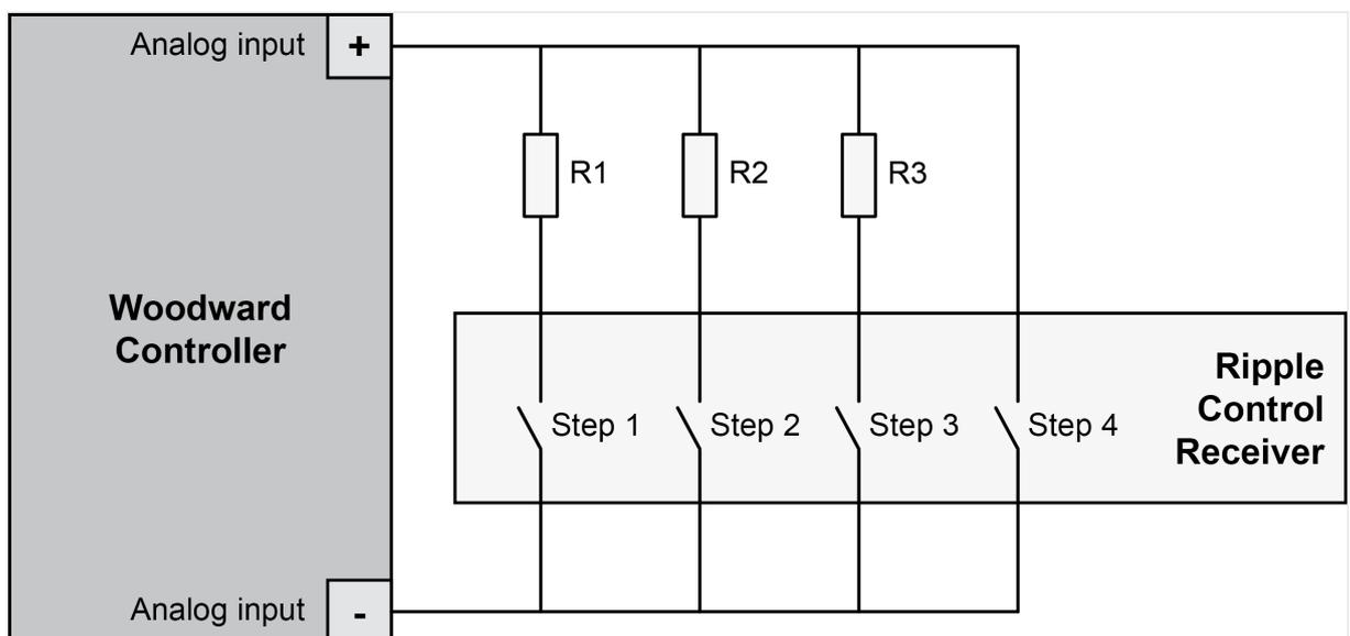
Fig. 291: Ripple control receiver wiring
