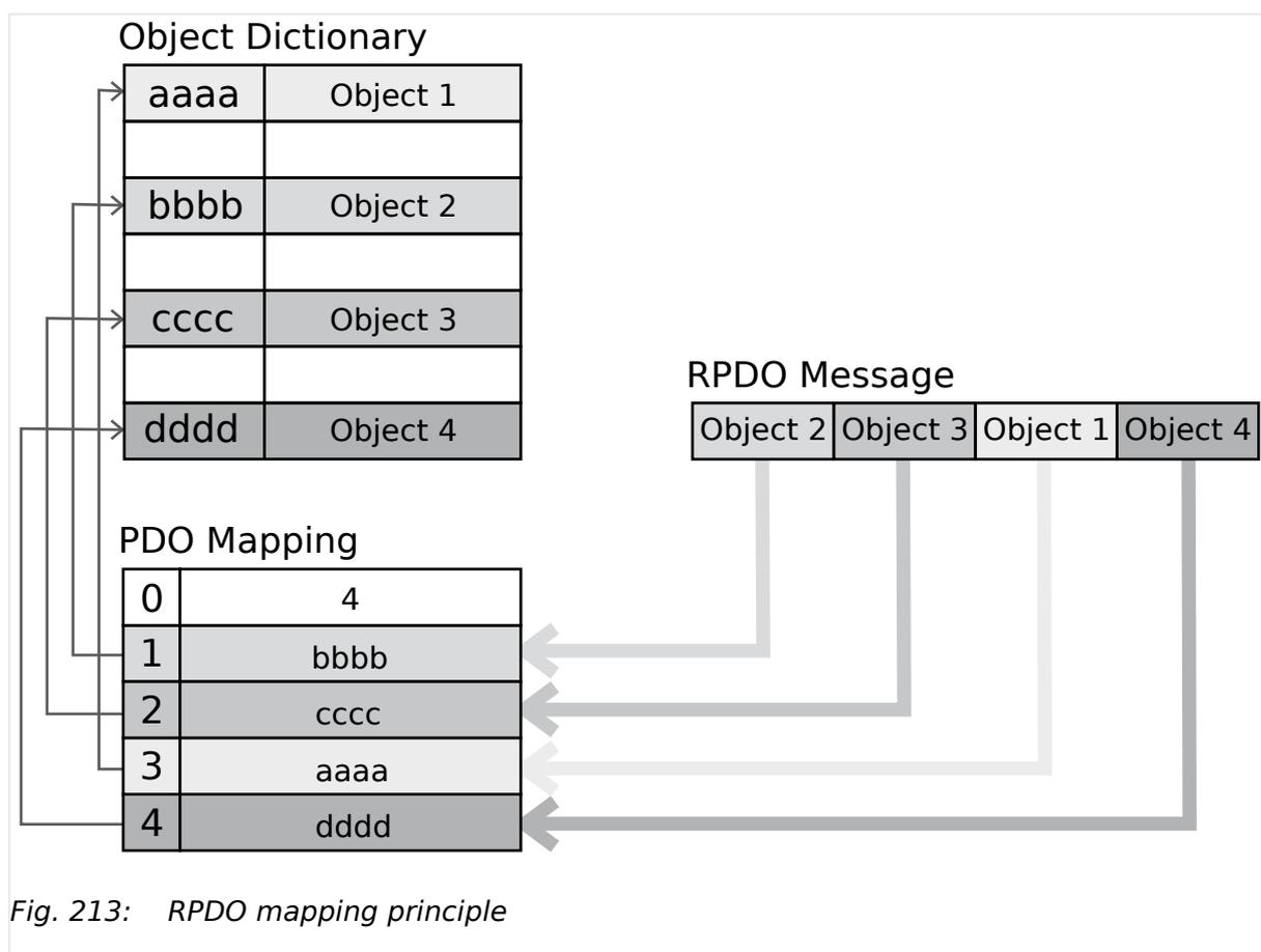
Fig. 213: RPDO mapping principle
