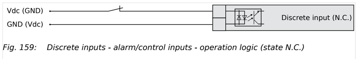
Fig. 159: Discrete inputs - alarm/control inputs - operation logic (state N.C.)
