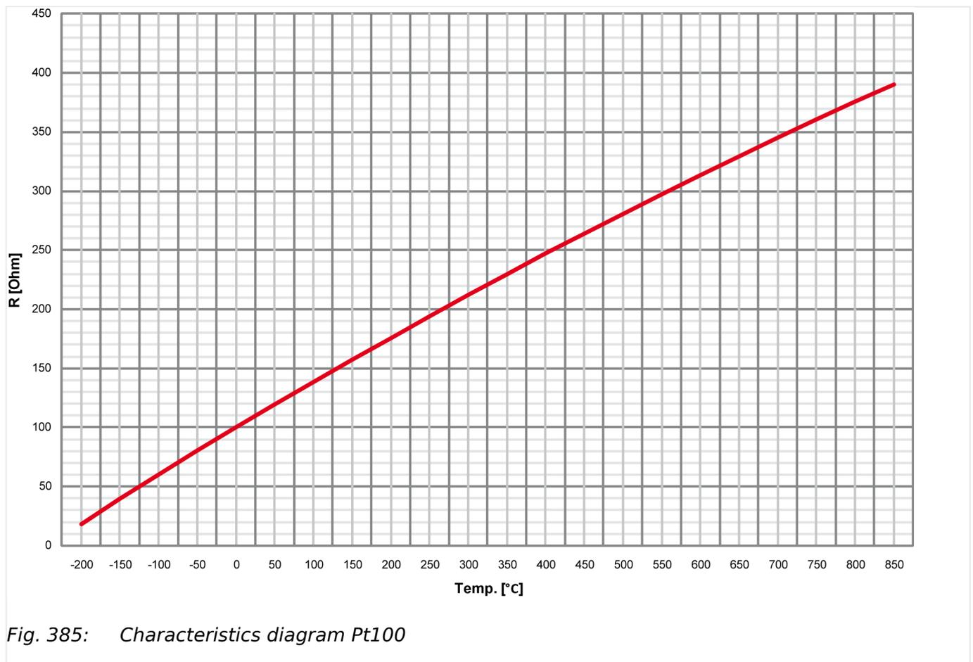
Fig. 385: Characteristics diagram Pt100
