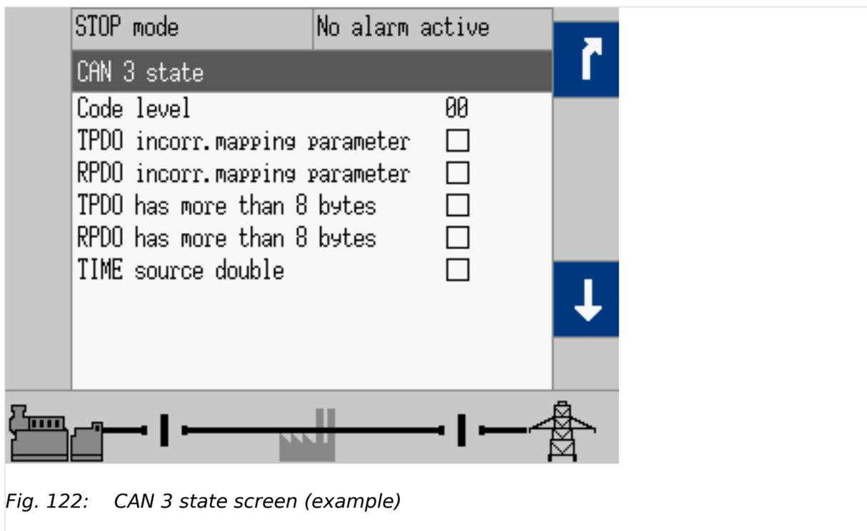
Fig. 122: CAN 3 state screen (example)
