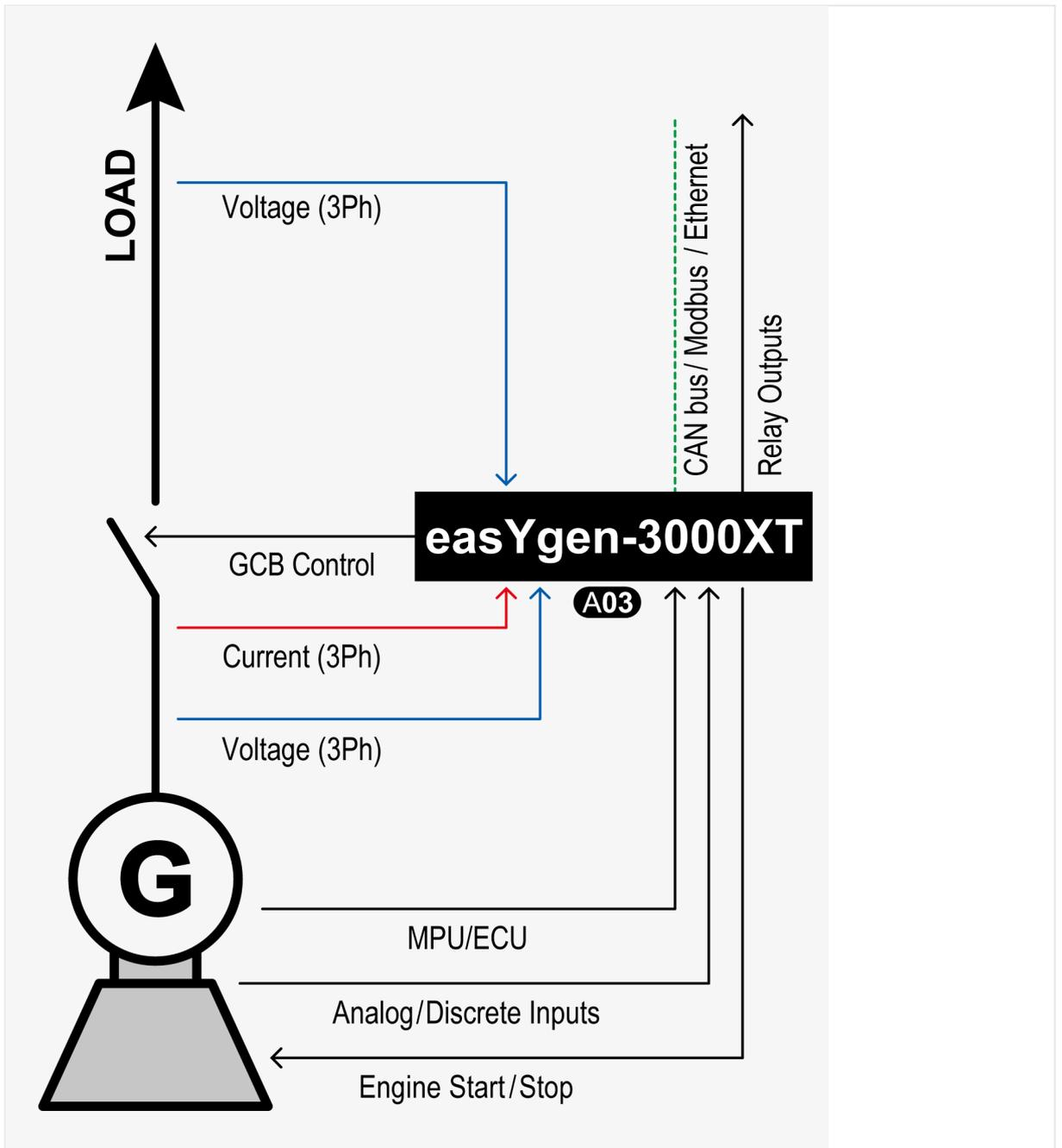
Fig. 230: Application mode (schematic)
