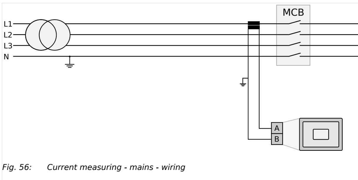
Fig. 56: Current measuring - mains - wiring
