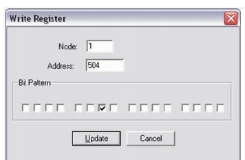
Fig. 319: Modbus - write register - shutdown command
