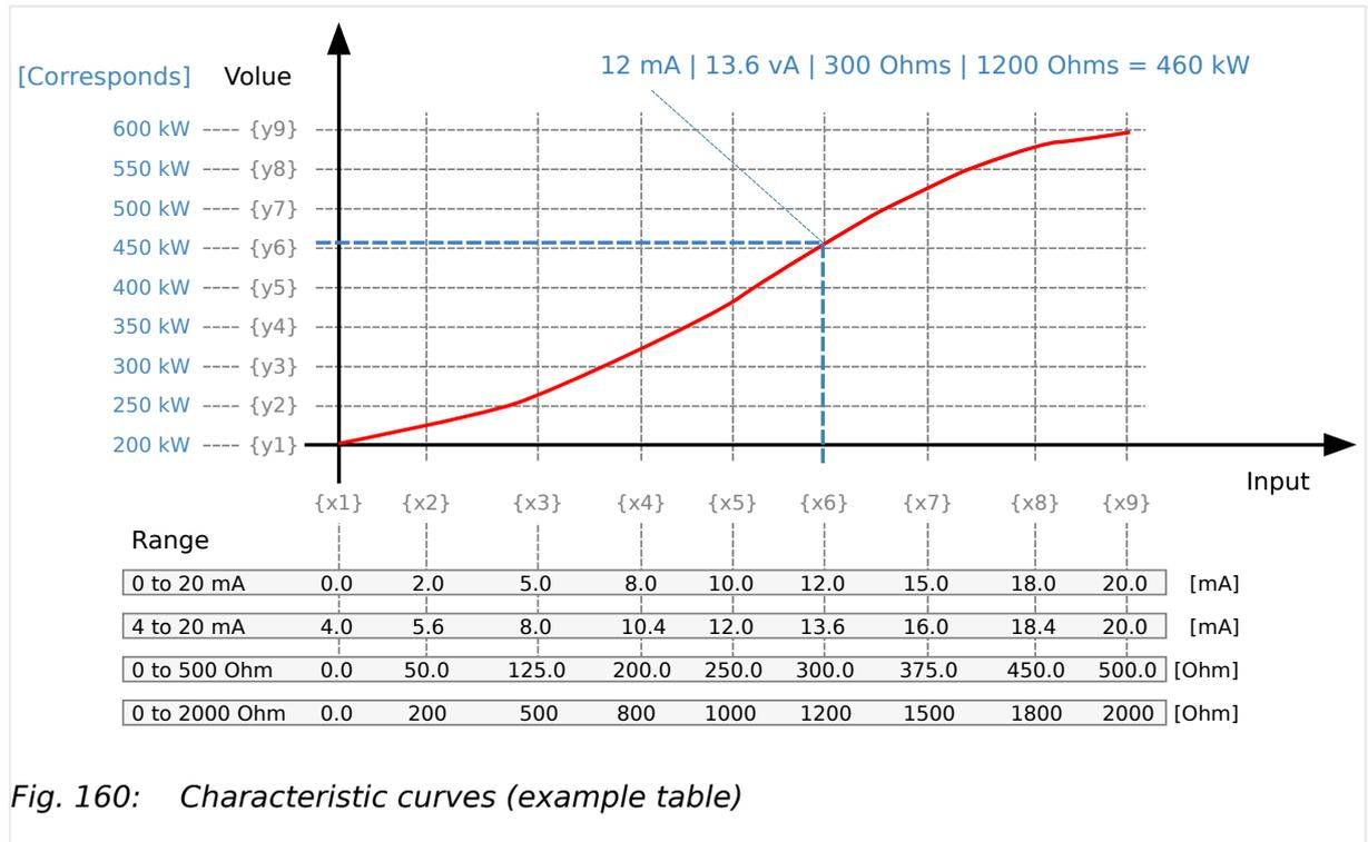
Fig. 160: Characteristic curves (example table)
