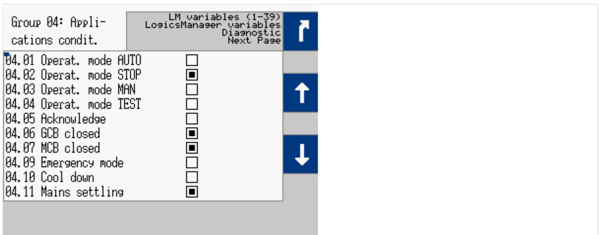
Fig. 109: Command variables screen (example)
