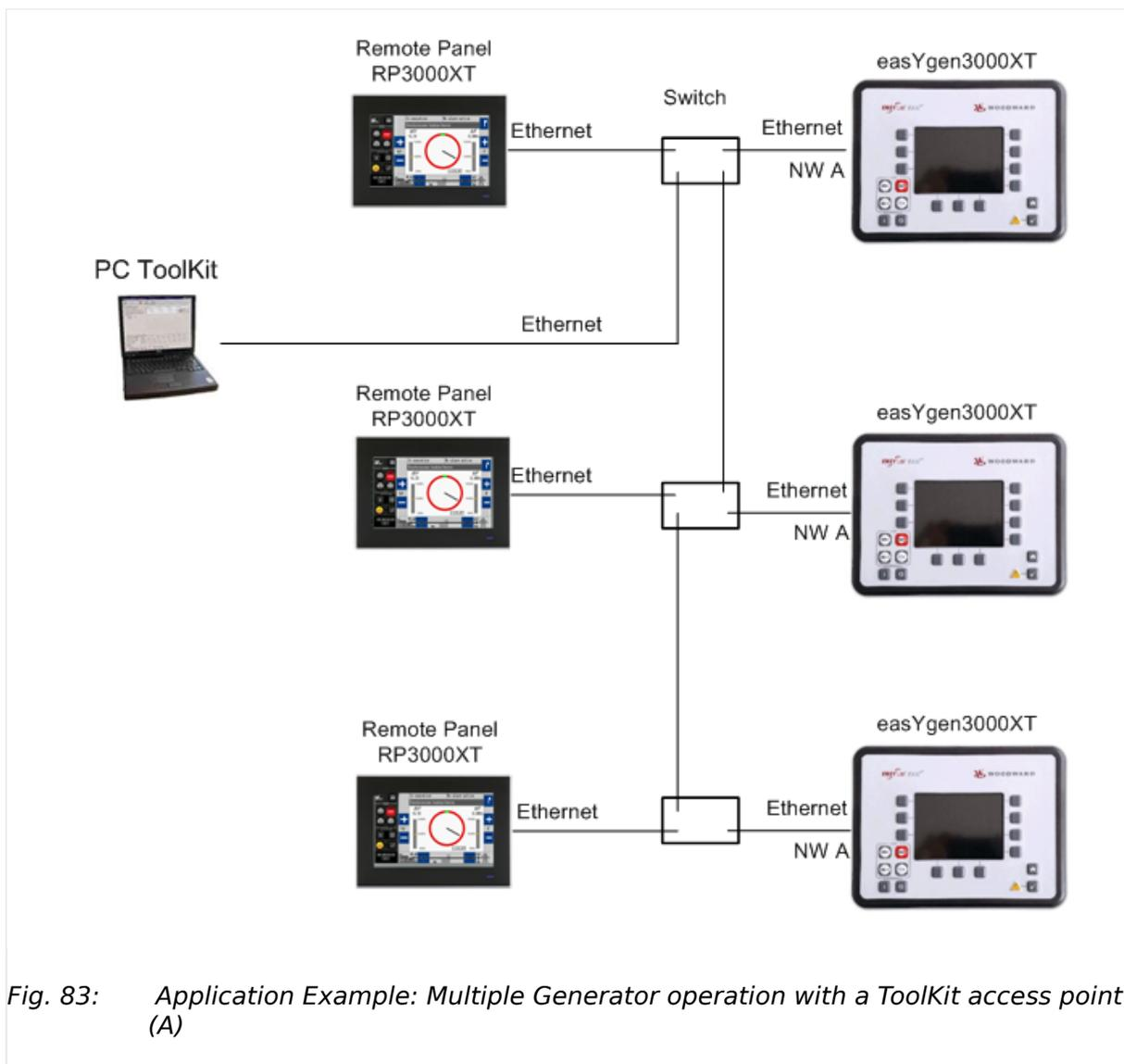
Fig. 83: Application Example: Multiple Generator operation with a ToolKit access point (A)
