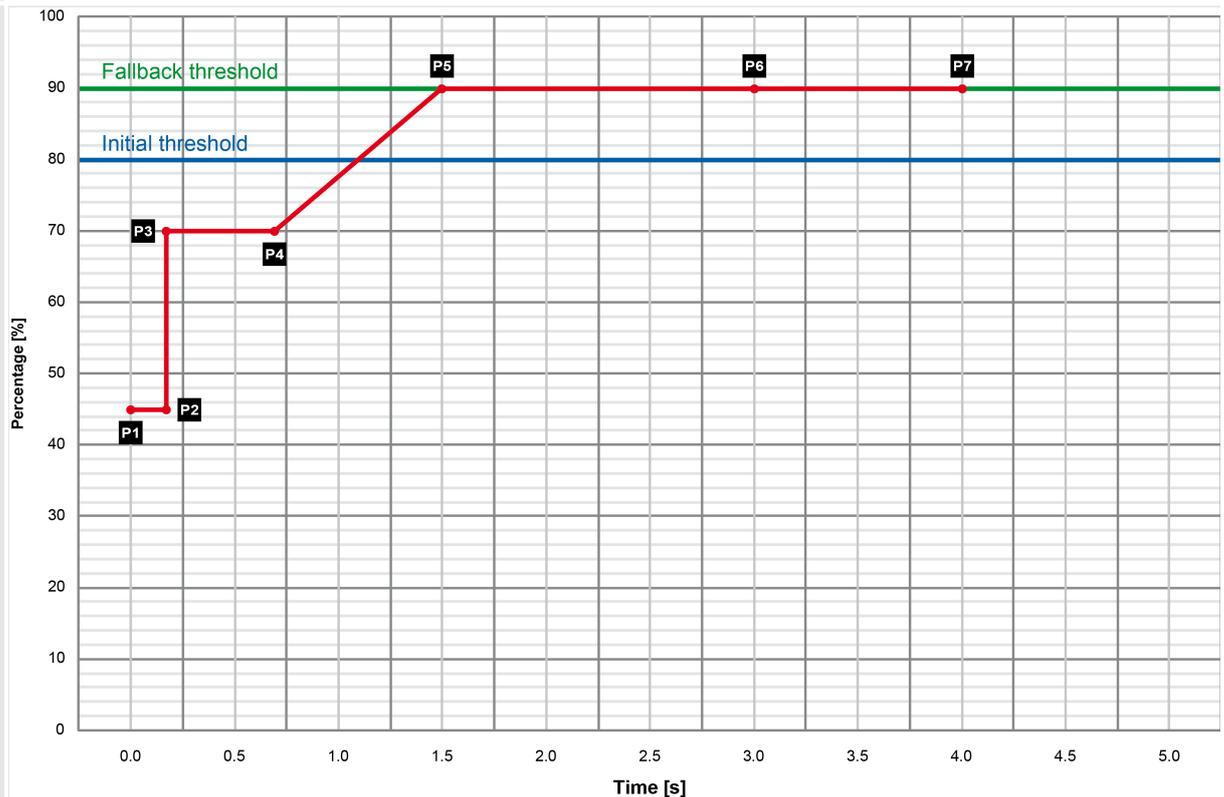
Fig. 205: Time-dependent voltage monitoring curve
