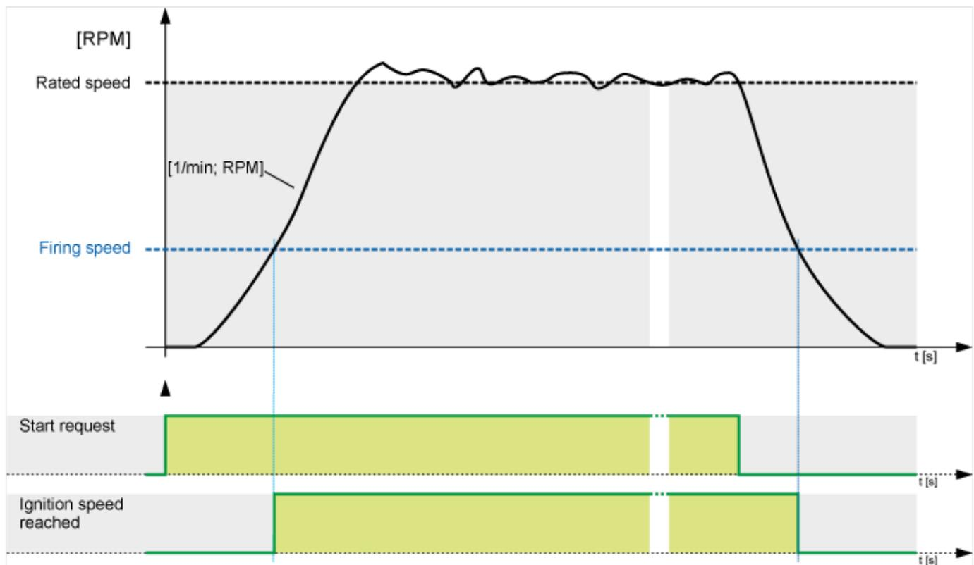
Fig. 154: Engine - firing speed
