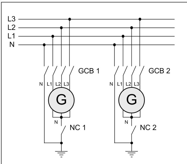
Fig. 295: Wiring neutral Interlocking: GCB 4-pole
