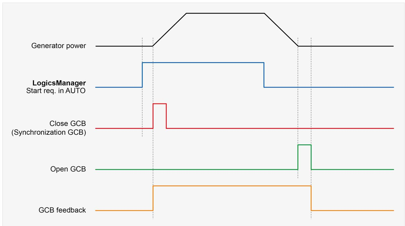
Fig. 290: Start/Stop sequence - LogicsManager Start req. in AUTO
