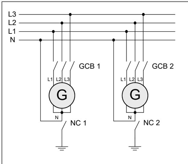
Fig. 294: Wiring neutral Interlocking: GCB 3-pole
