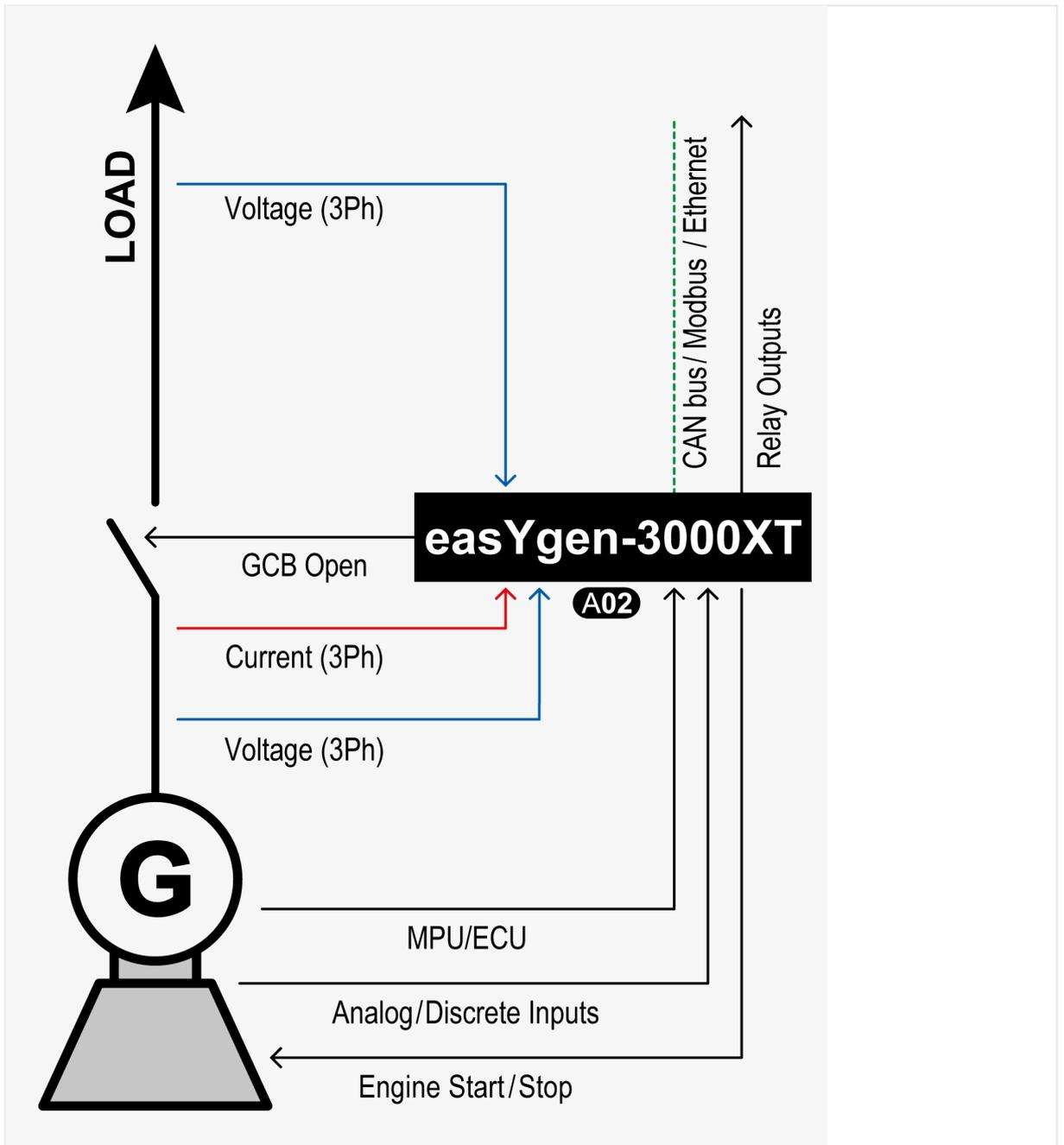
Fig. 229: Application mode A02 (schematic)
