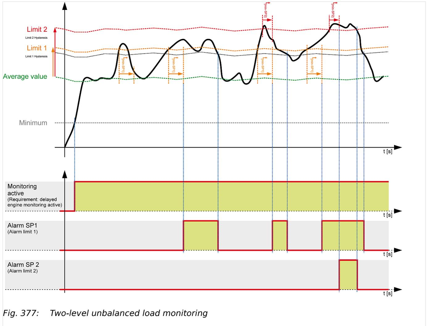
Fig. 377: Two-level unbalanced load monitoring
