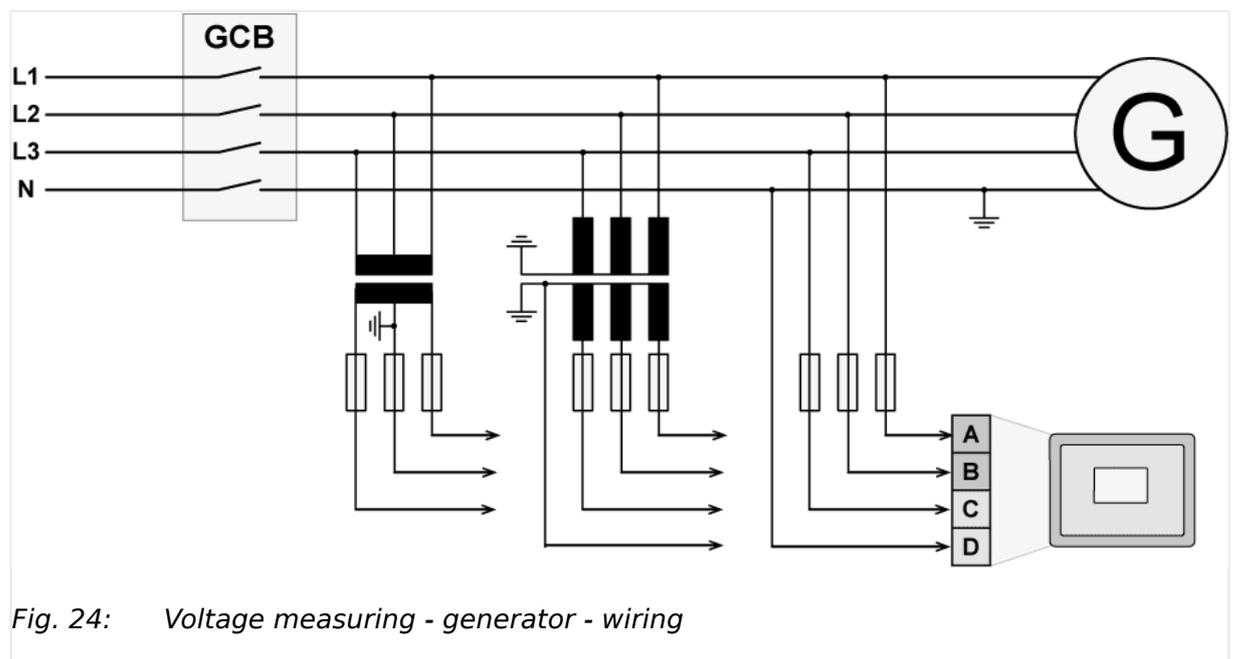
Fig. 24: Voltage measuring - generator - wiring
