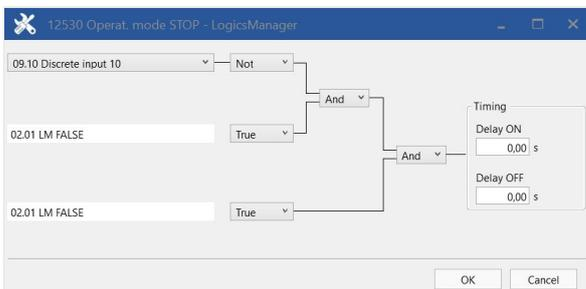
Fig. 260: LogicsManager function "Operat. mode STOP"
