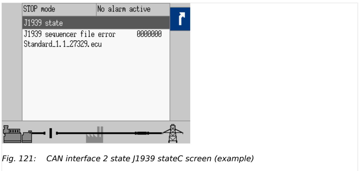
Fig. 121: CAN interface 2 state J1939 stateC screen (example)
