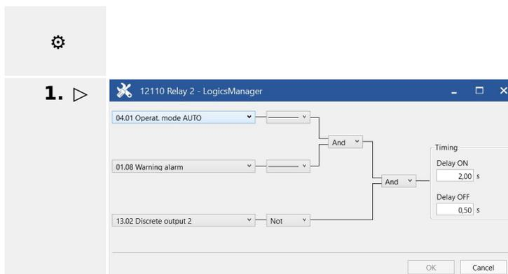
Fig. 251: LogicsManager function "Relay 2"
