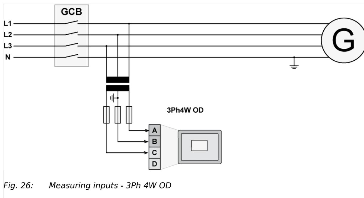
Fig. 26: Measuring inputs - 3Ph 4W OD
