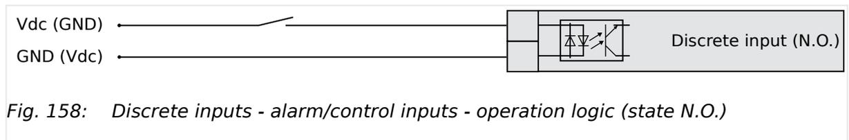
Fig. 158: Discrete inputs - alarm/control inputs - operation logic (state N.O.)
