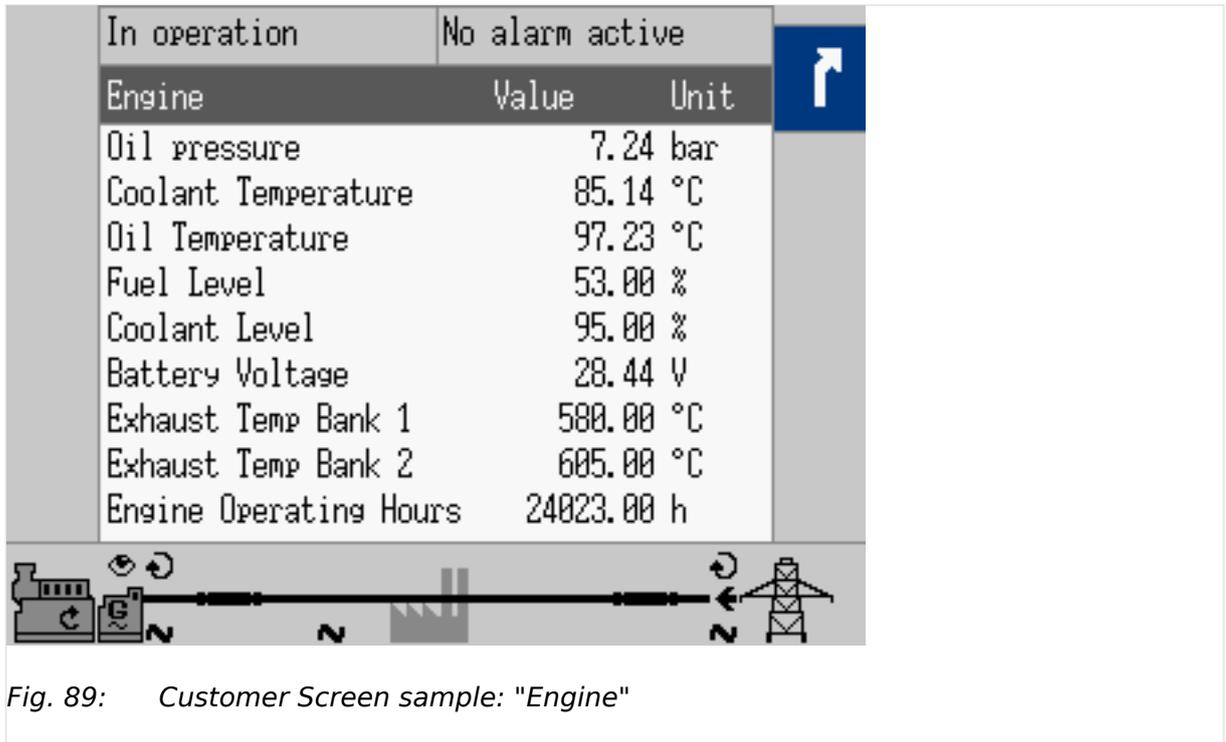
Fig. 89: Customer Screen sample: "Engine"
