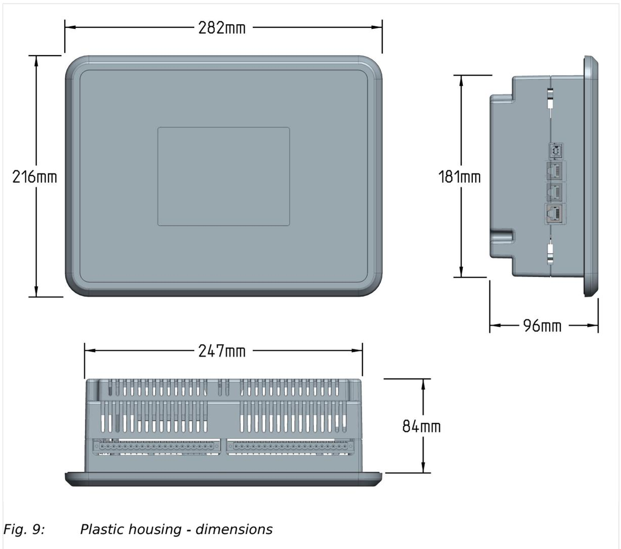
Fig. 9: Plastic housing - dimensions
