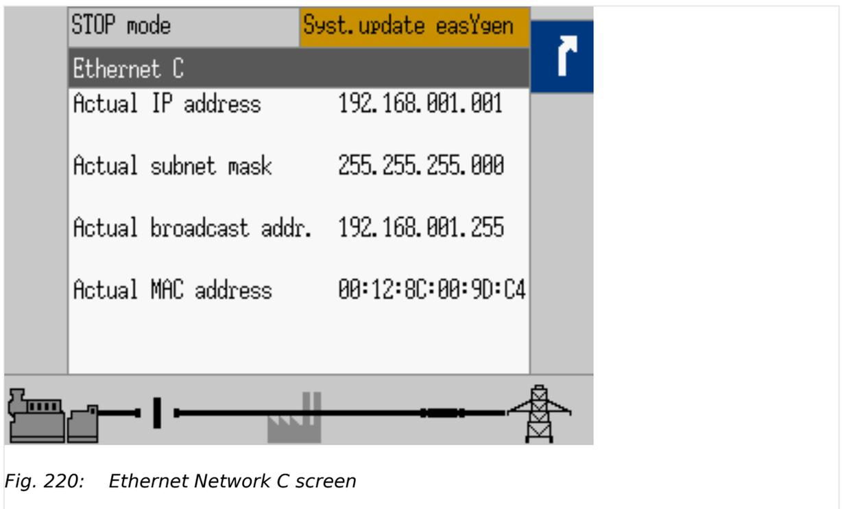
Fig. 220: Ethernet Network C screen
