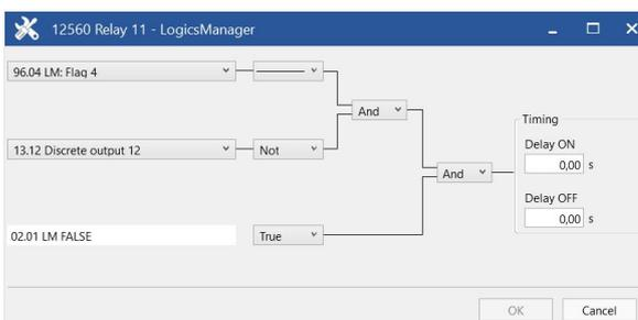
Fig. 252: LogicsManager function "Relay 11"
