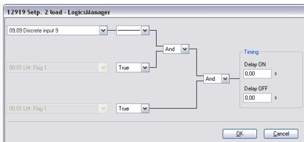
Fig. 248: LogicsManager function "Setp. 2 load"
