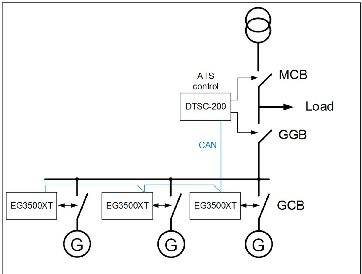
Fig. 311: Example of an application with parameter 9066 "Predicted load source" is configured as "External". Additionally, there is a hardwired inhibit signal from easYgens to the ATS".
