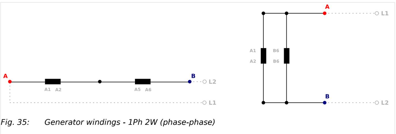
Fig. 35: Generator windings - 1Ph 2W (phase-phase)
