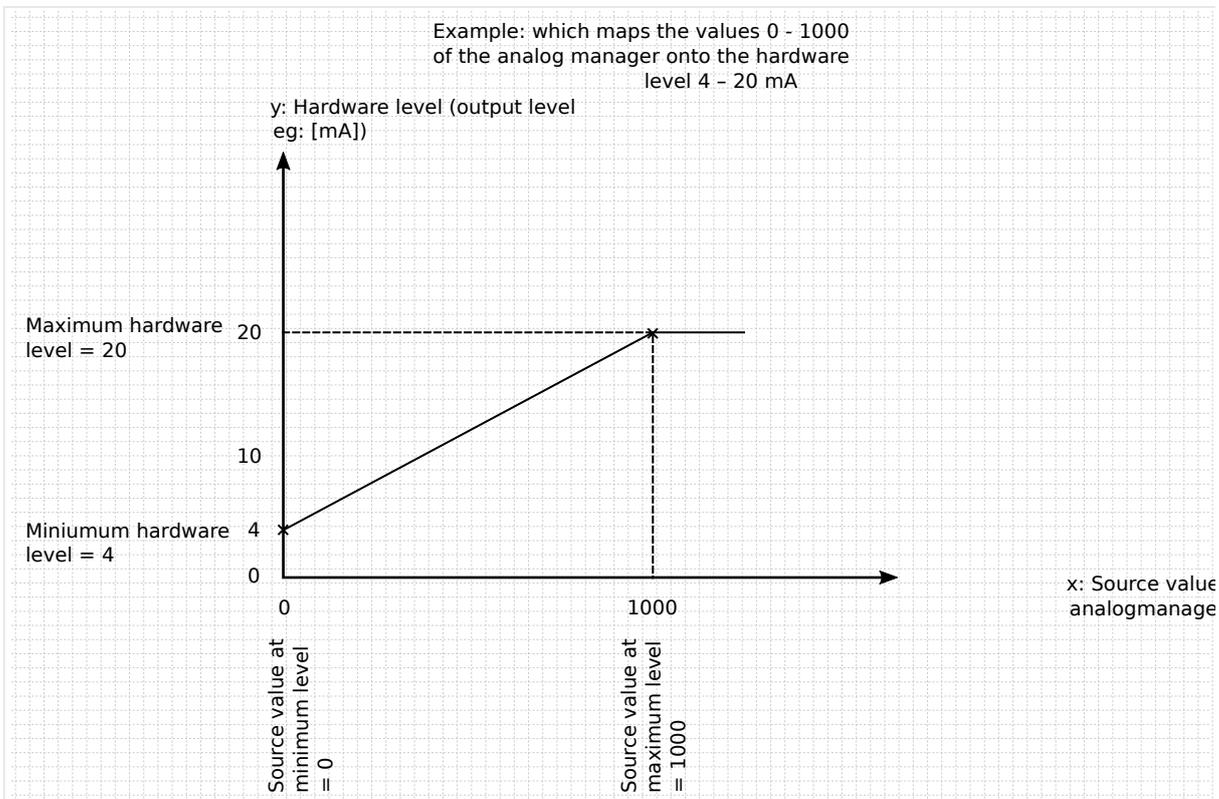
Fig. 162: Example to setup AO for 0 to 1000 IN becomes OUT 4 to 20 mA
