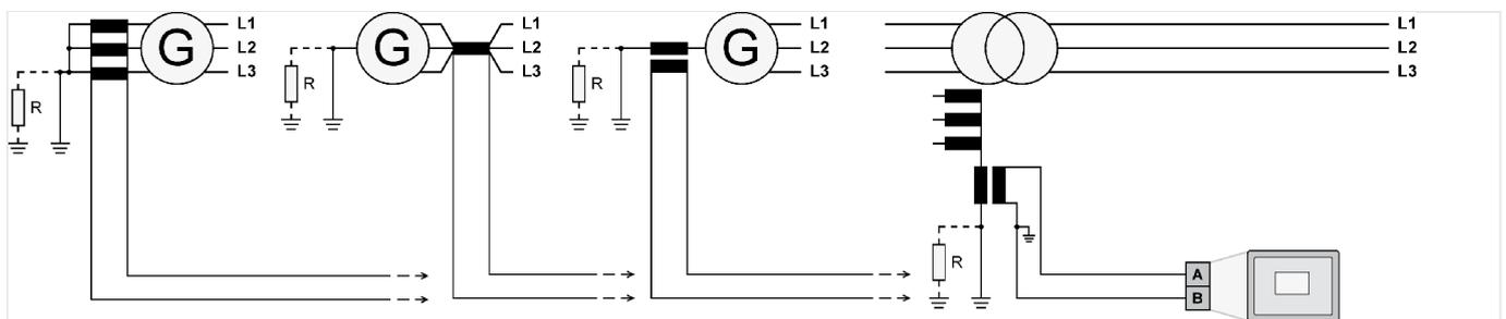
Fig. 58: Current measuring - ground current - wiring
