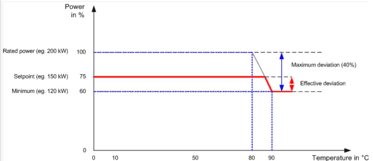
Fig. 312: Derating: Mains parallel operation; setpoint below rated power
