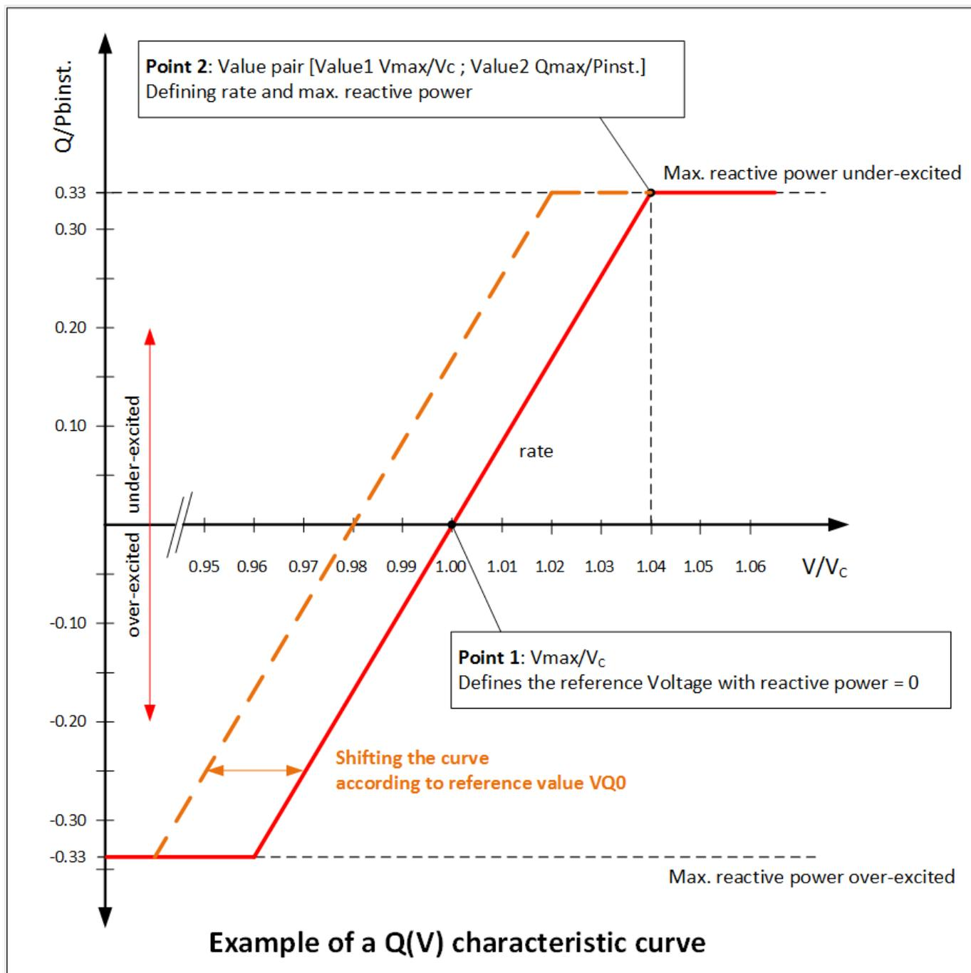
Fig. 175: EGXT\_Example\_of\_a\_Q(V)\_characteristic
