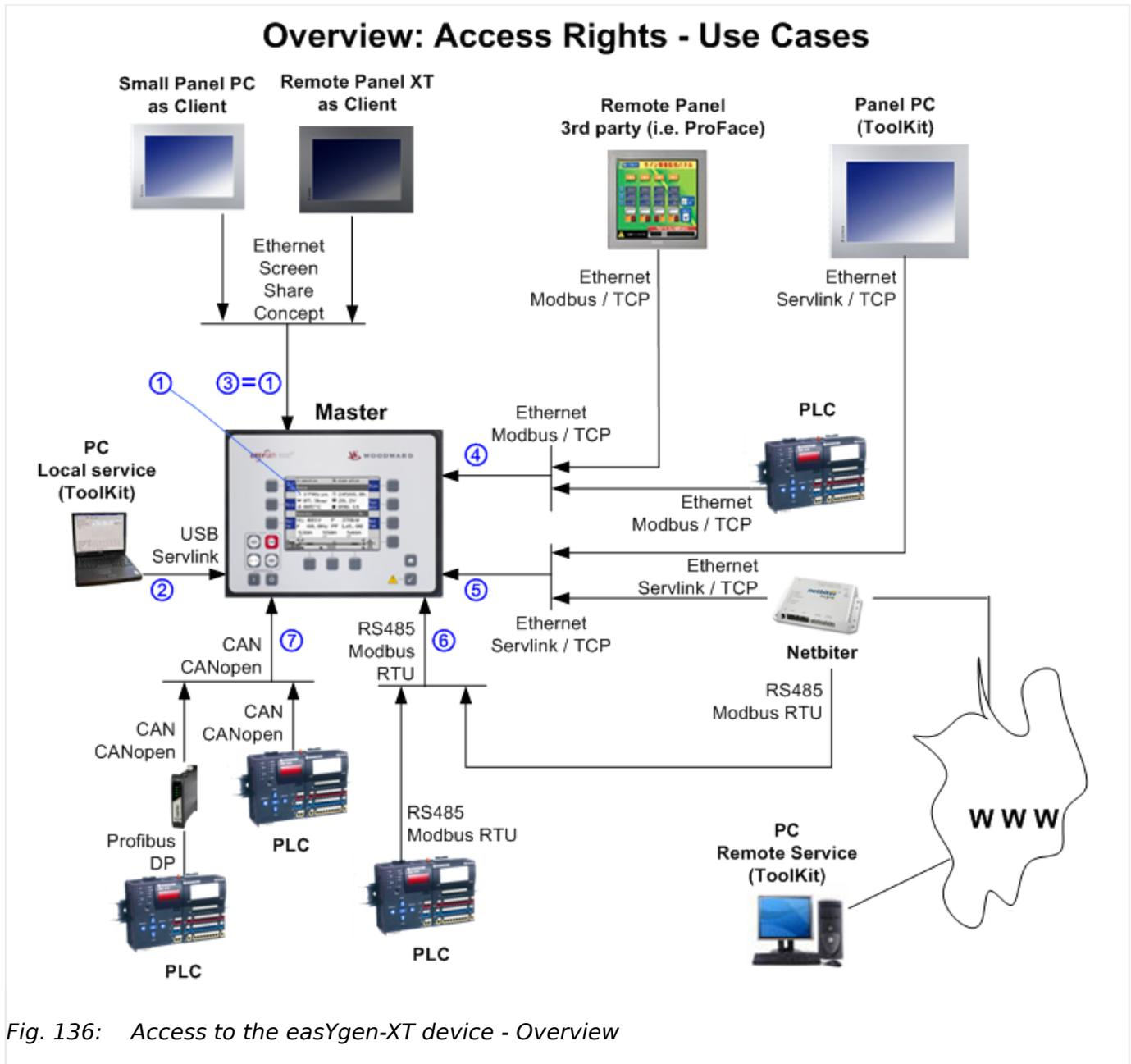
Fig. 136: Access to the easYgen-XT device - Overview
