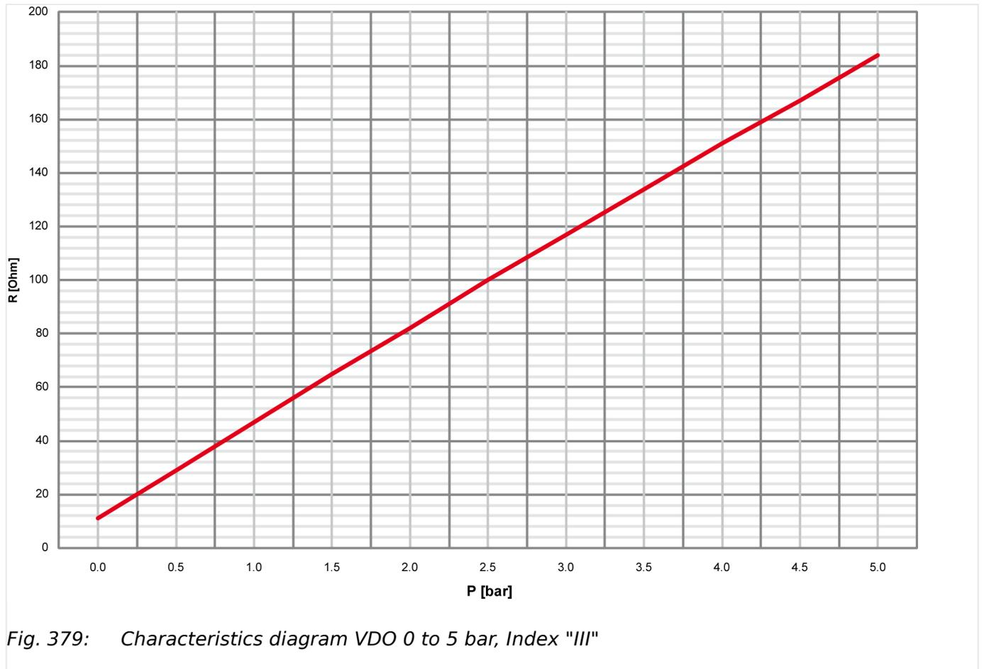
Fig. 379: Characteristics diagram VDO 0 to 5 bar, Index "III"
