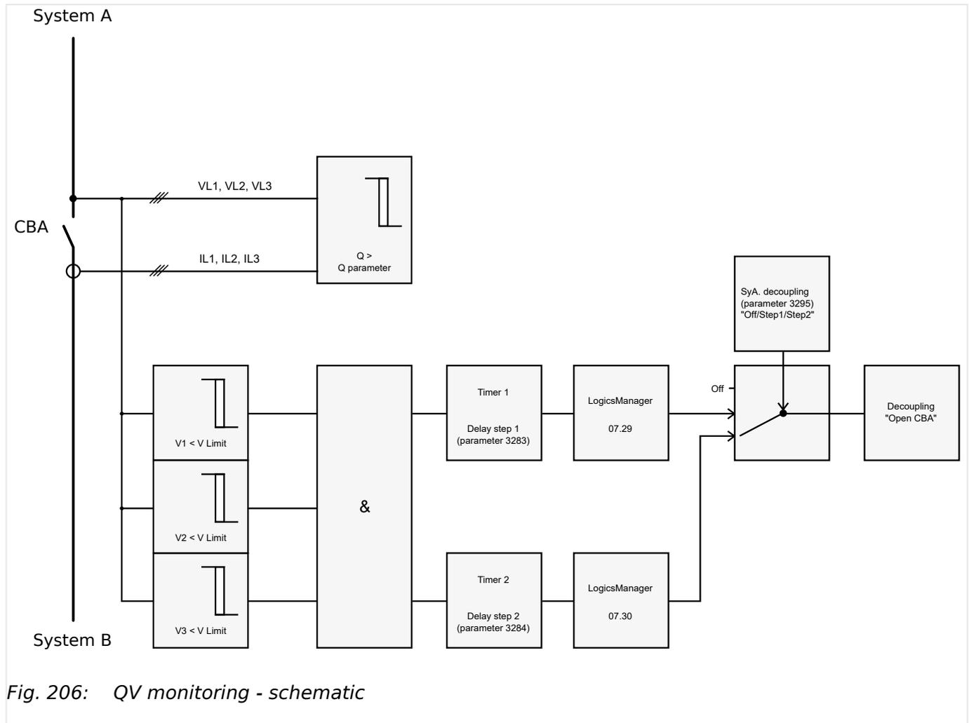
Fig. 206: QV monitoring - schematic
