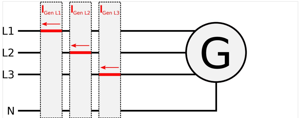
Fig. 54: Current measuring - generator, L1 L2 L3
