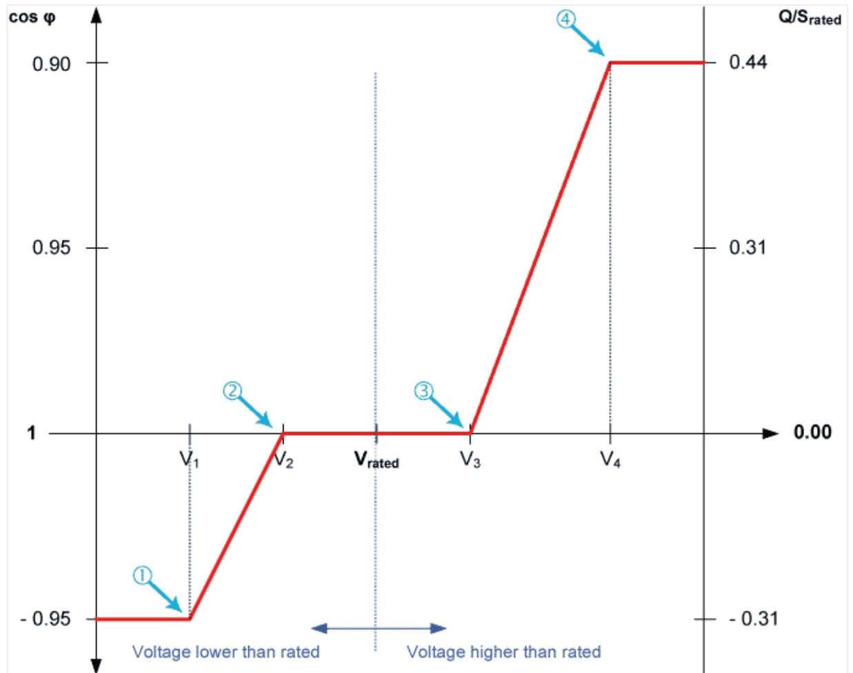
Fig. 172: Power factor characteristic according to the relation  $Q/S$  rated over rated voltage
