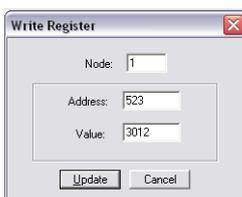
Fig. 352: Write register - acknowledge alarm message
