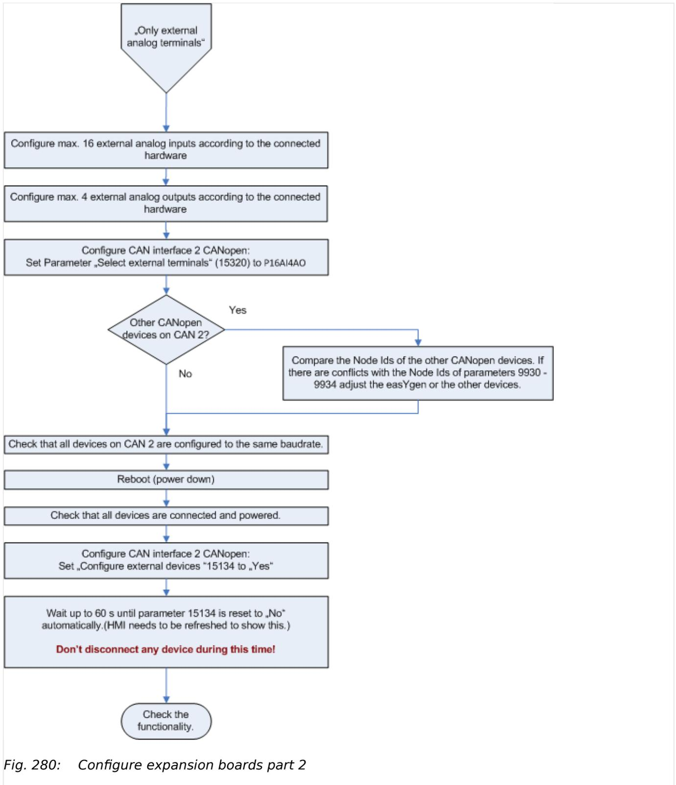
Fig. 280: Configure expansion boards part 2
