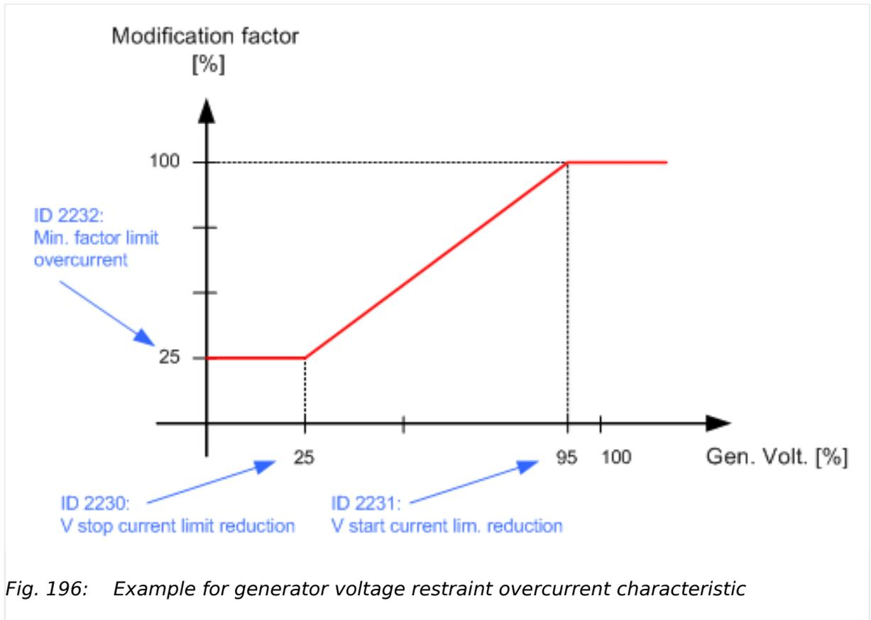
Fig. 196: Example for generator voltage restraint overcurrent characteristic
