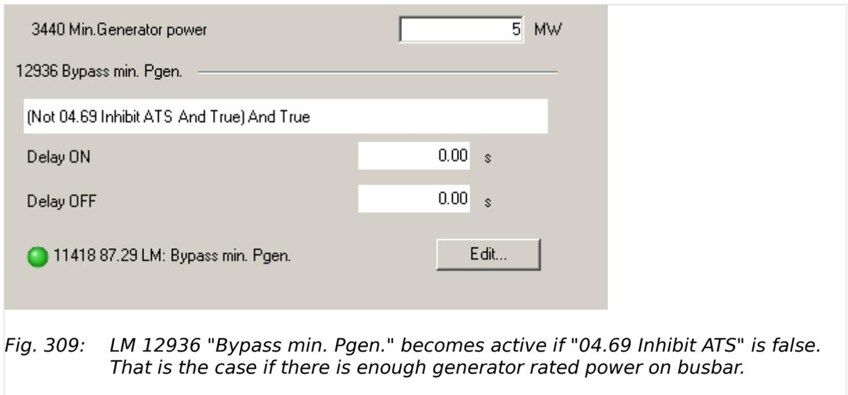
Fig. 309: LM 12936 "Bypass min. Pgen." becomes active if "04.69 Inhibit ATS" is false. That is the case if there is enough generator rated power on busbar.
