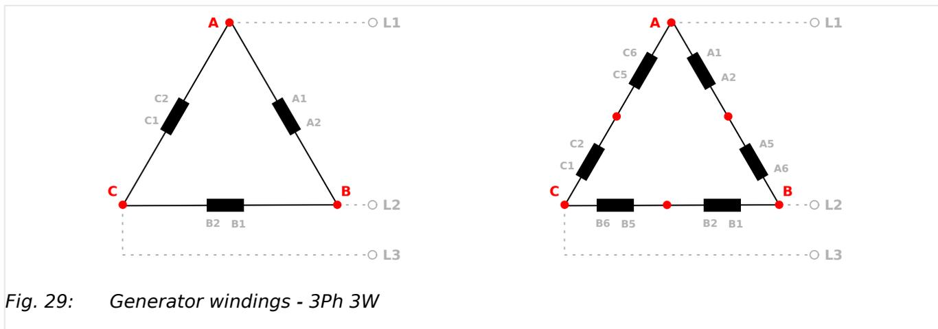
Fig. 29: Generator windings - 3Ph 3W
