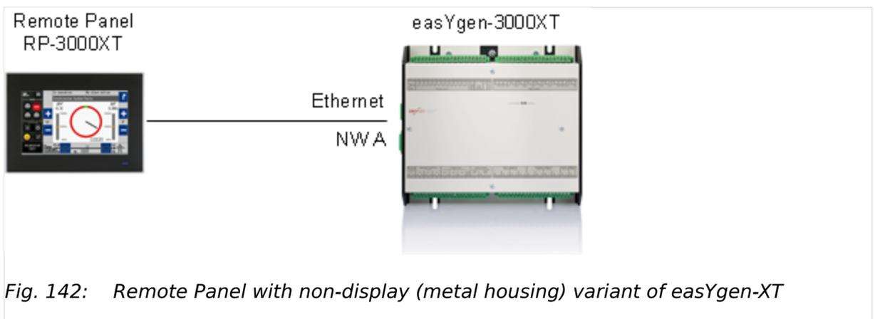
Fig. 142: Remote Panel with non-display (metal housing) variant of easYgen-XT
