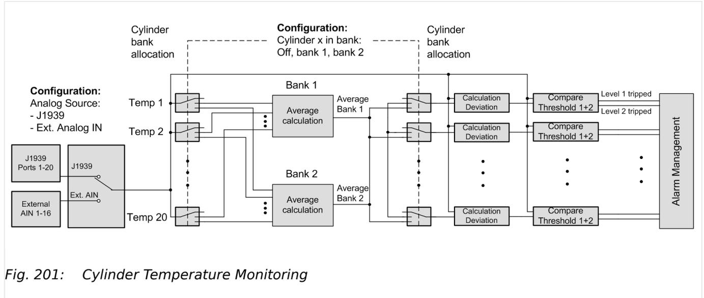
Fig. 201: Cylinder Temperature Monitoring
