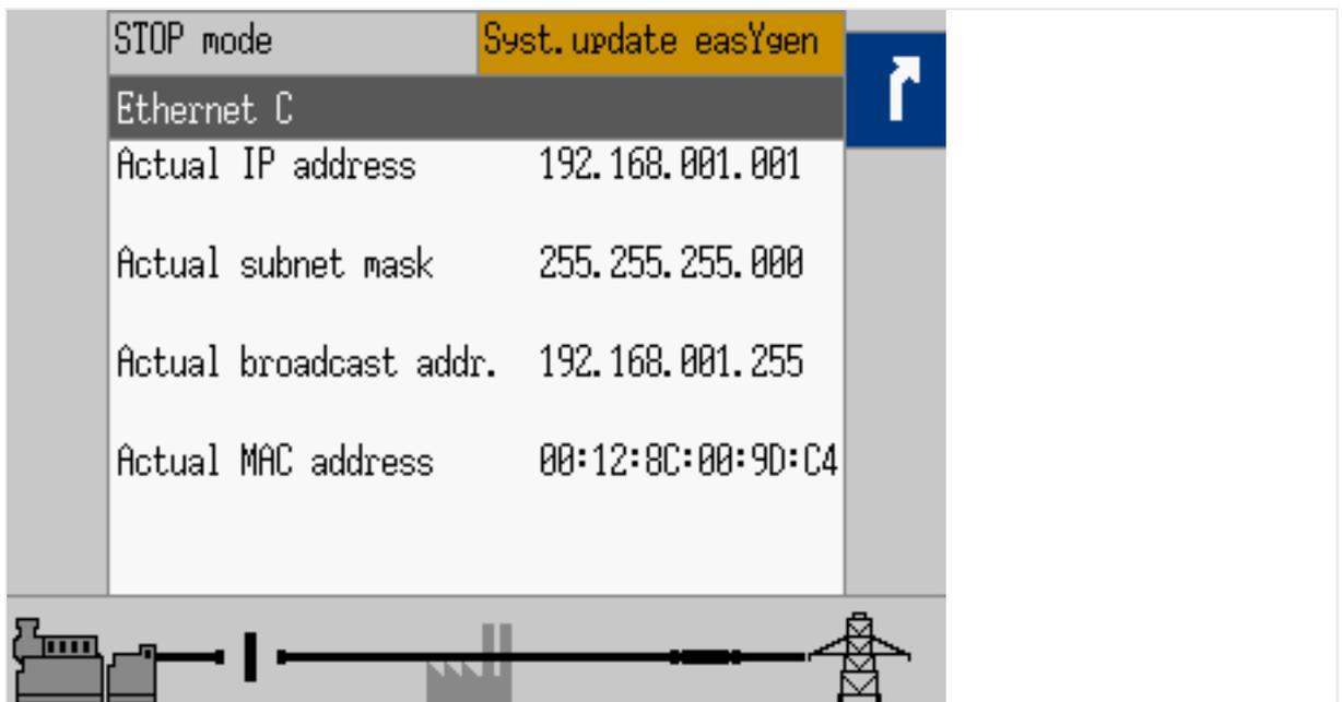
Fig. 366: Ethernet Network C screen
