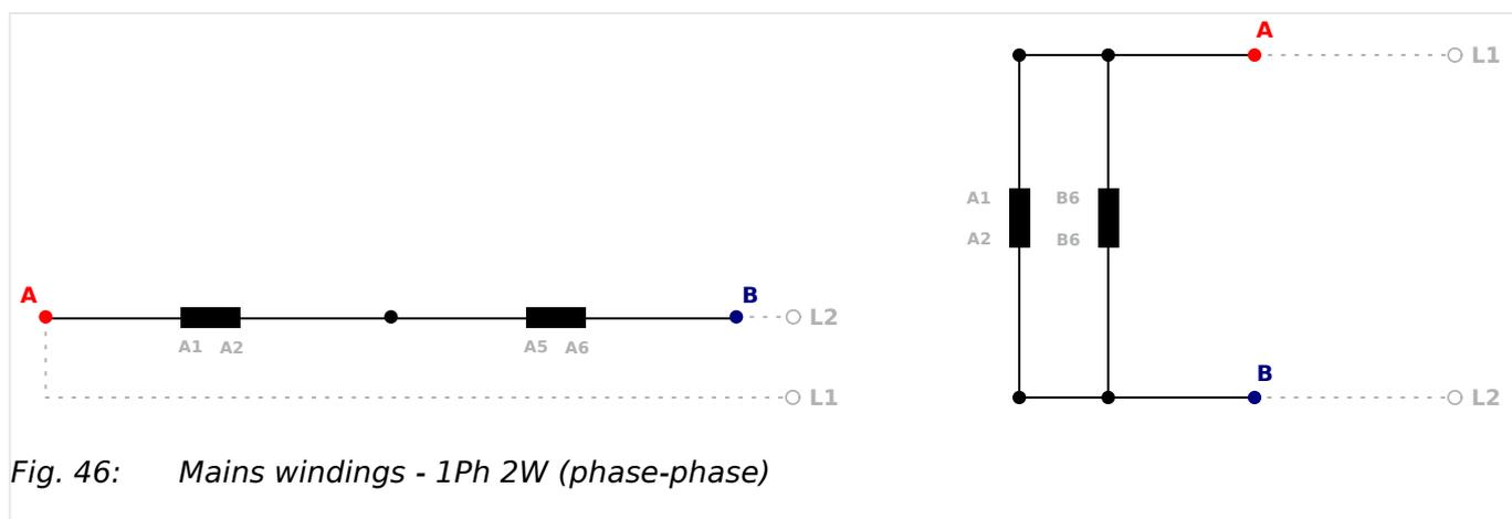
Fig. 46: Mains windings - 1Ph 2W (phase-phase)
