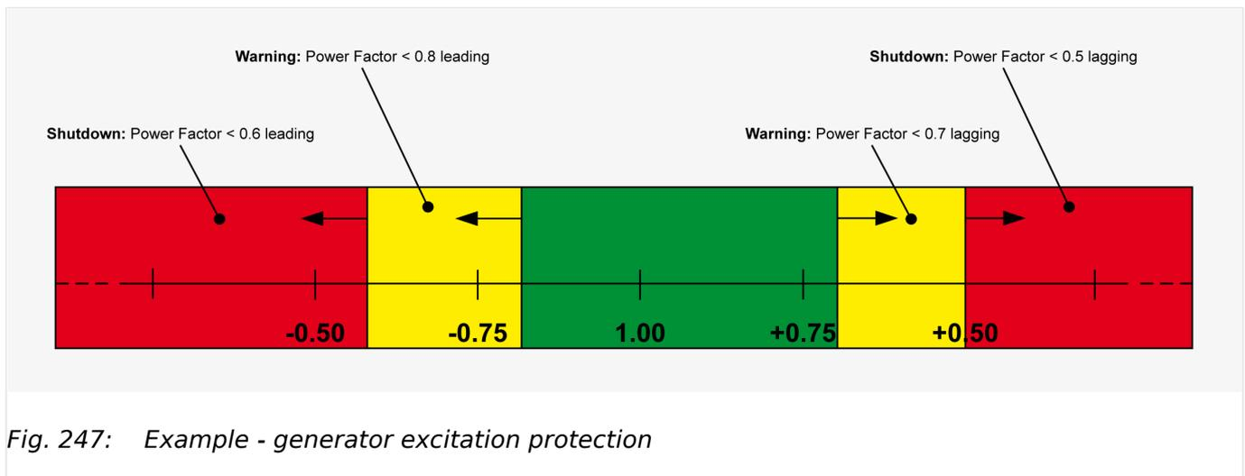
Fig. 247: Example - generator excitation protection
