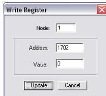
Fig. 358: Write register - resetting the default values
