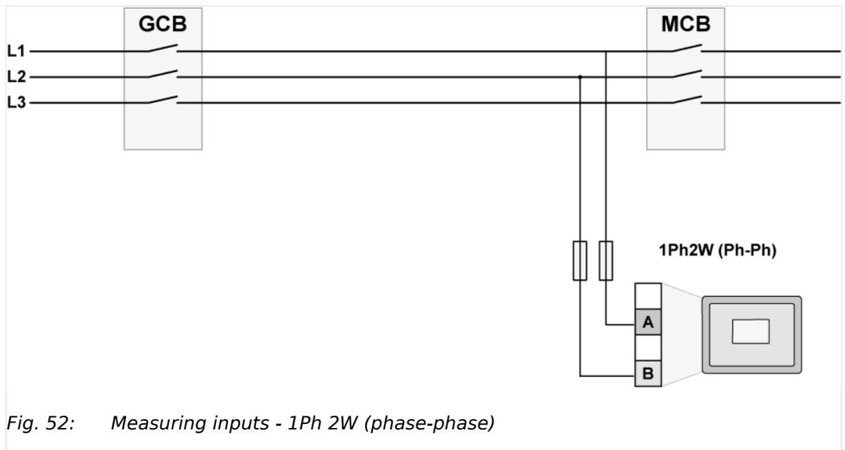
Fig. 52: Measuring inputs - 1Ph 2W (phase-phase)
