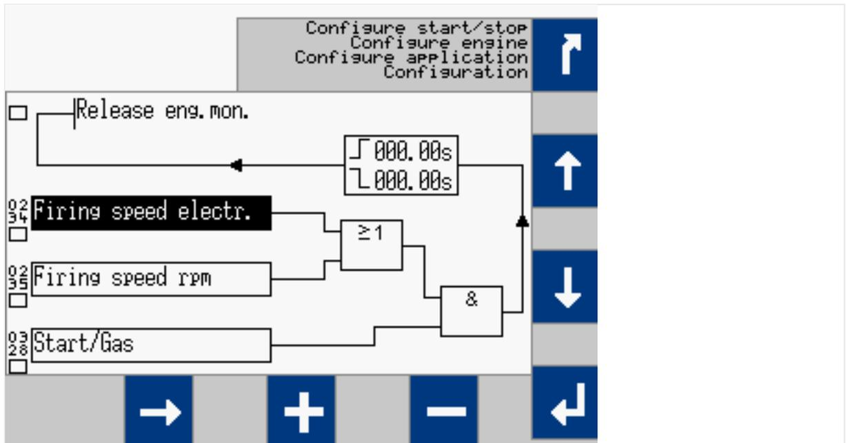
Fig. 157: Release Engine Monitoring screen
