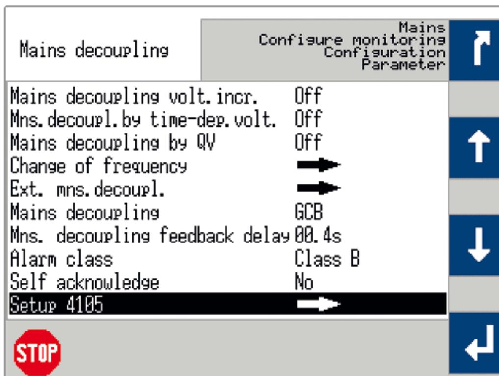
Fig. 204: Select mains decoupling 4105
