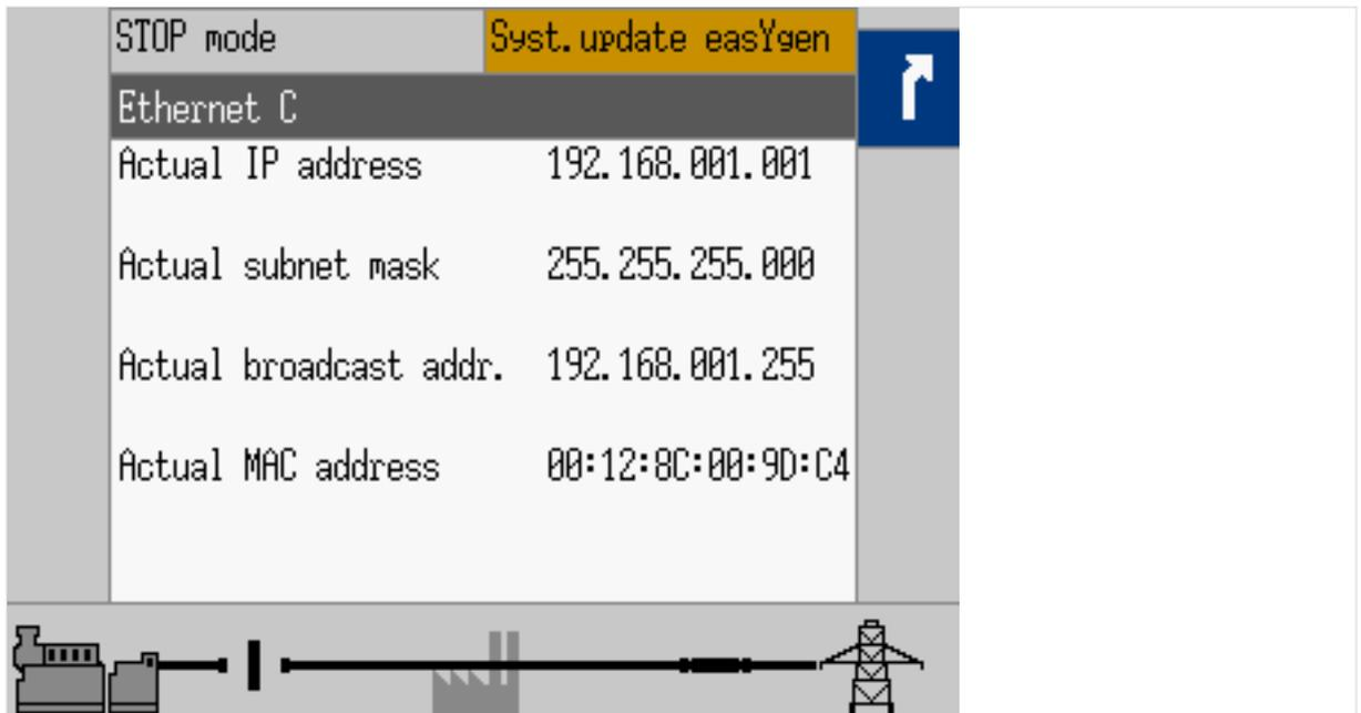
Fig. 126: Ethernet C state screen (example)
