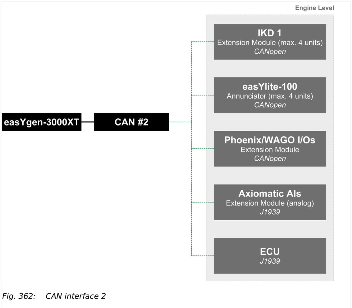
CAN interface 2 is pre-configured for several expansion units. These include the I/O expansion boards Woodward IKD 1, several combinations of the expansion boards of the Phoenix Inline Modular (IL) series, and the support of Wago terminals.
