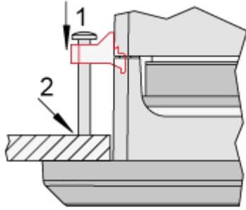
Fig. 14: Tighten clamping screws
