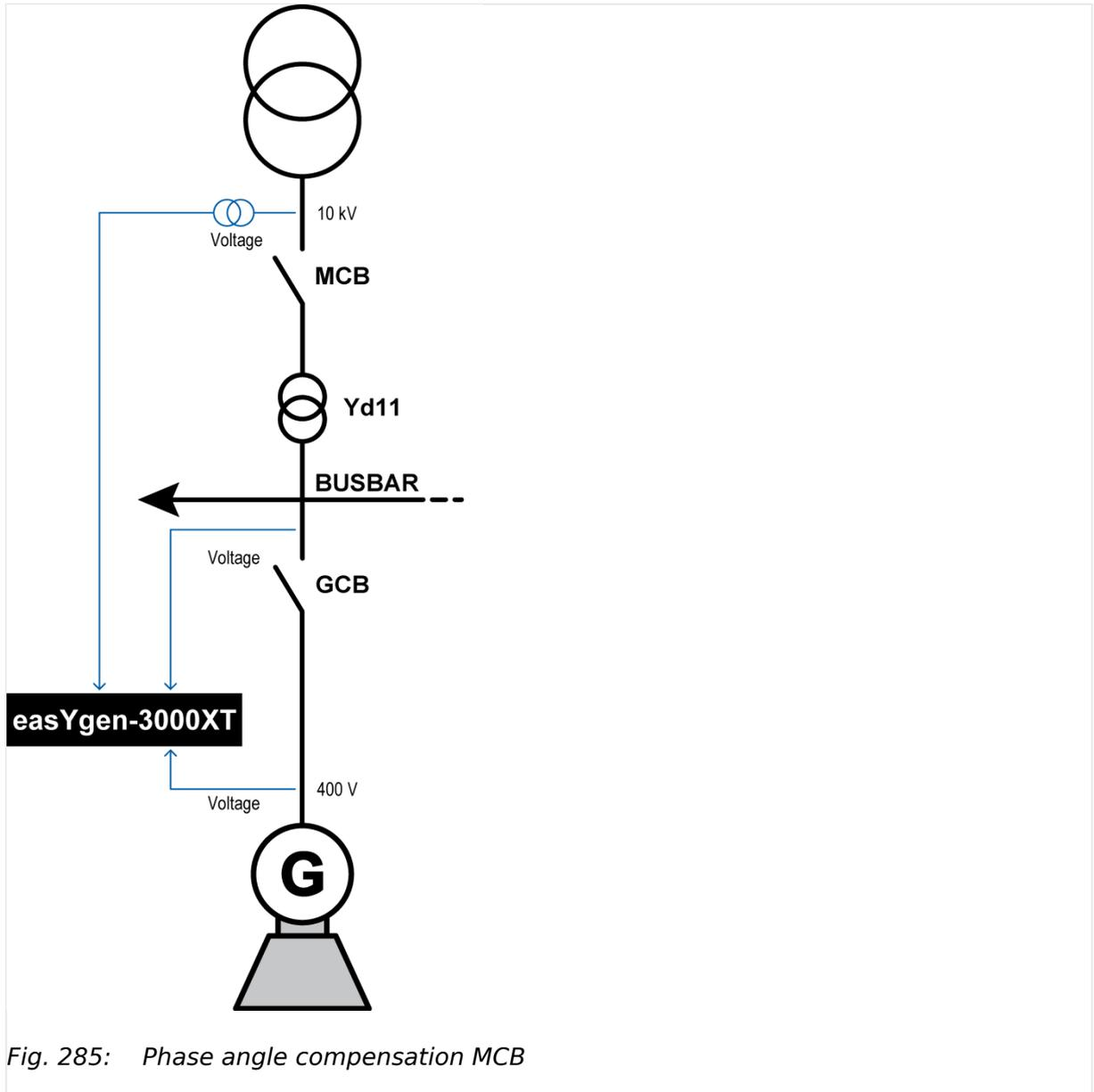
Fig. 285: Phase angle compensation MCB
