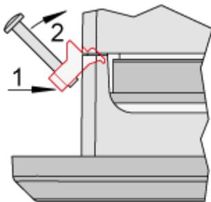
Fig. 13: Attach clamp inserts
