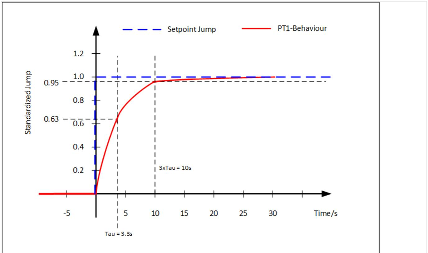
Fig. 173: Setpoint Jump (standardized with height 1) and the resulting PT1 setpoint
