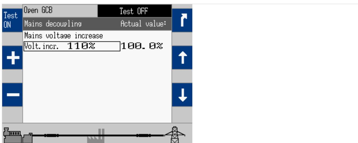
Fig. 114: Mains decoupling screen 4
