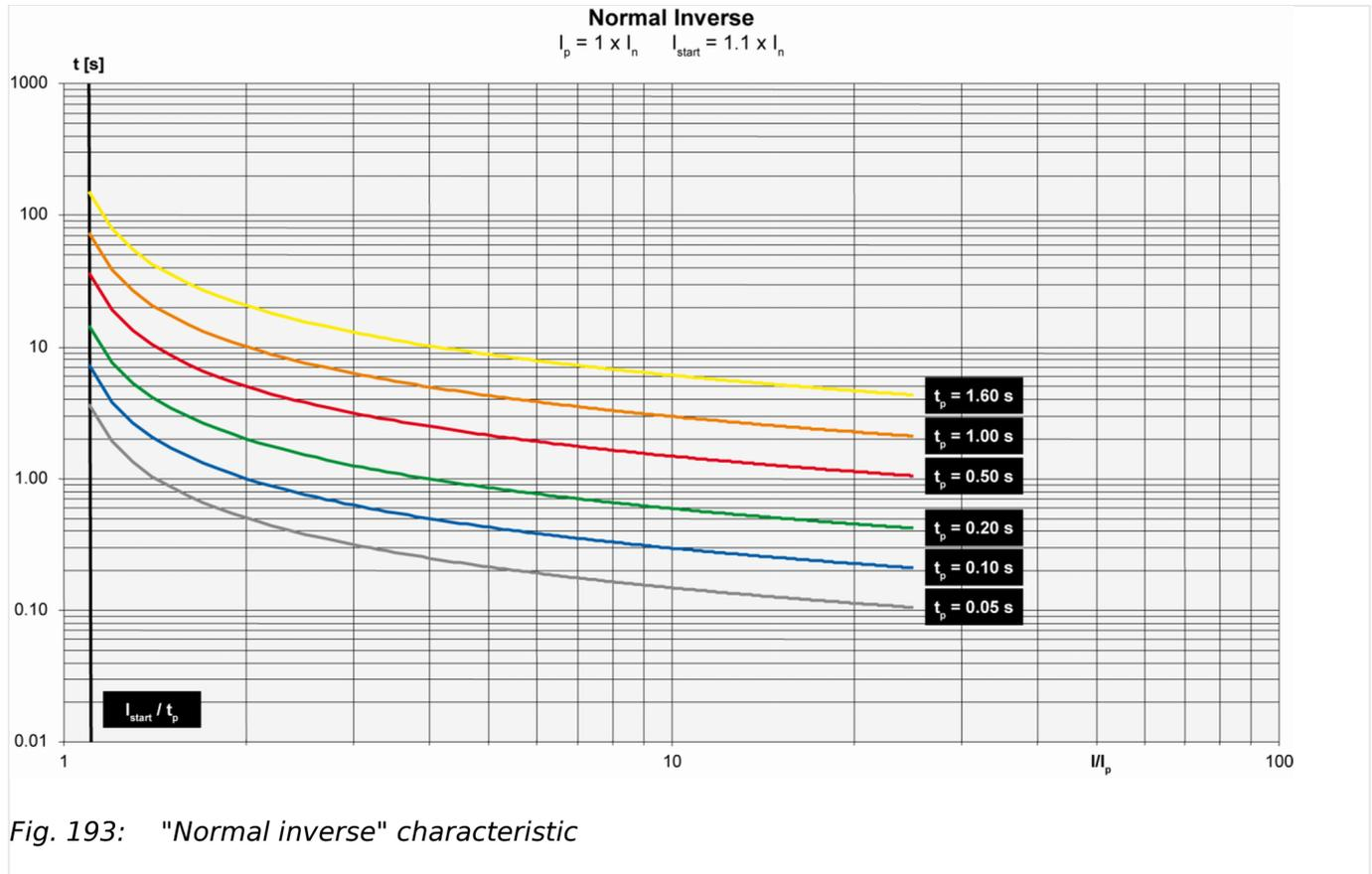
Fig. 193: "Normal inverse" characteristic
