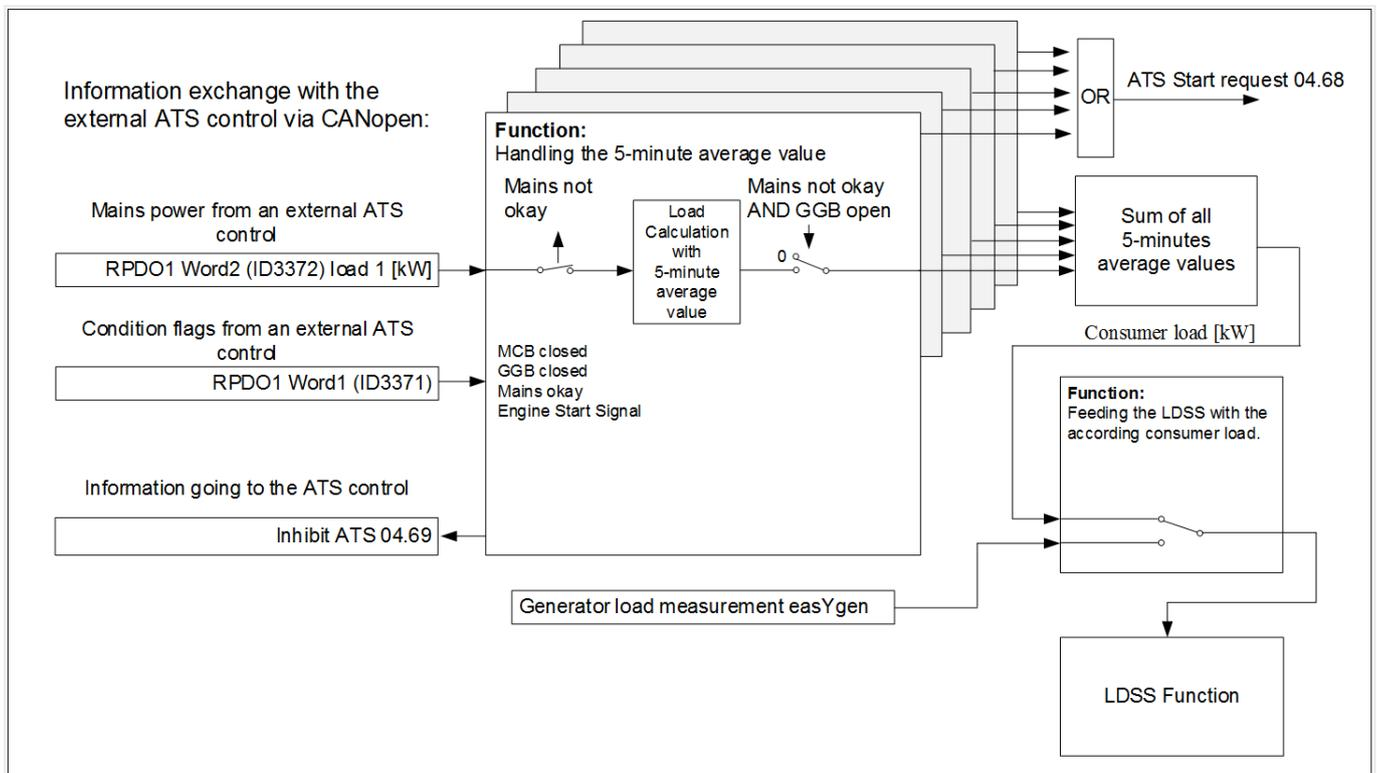
Fig. 310: The principle of the LDSS PL in external source mode
