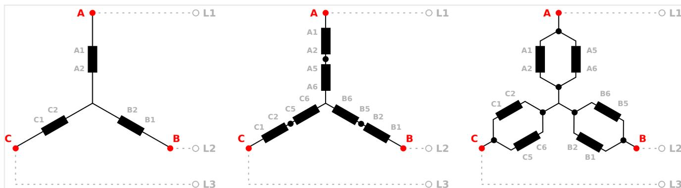
Fig. 25: Generator windings - 3Ph 4W OD
