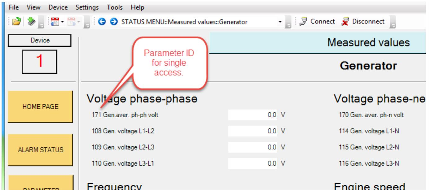
Fig. 391: ToolKit page with generator visualization data
