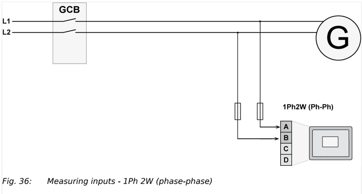
Fig. 36: Measuring inputs - 1Ph 2W (phase-phase)
