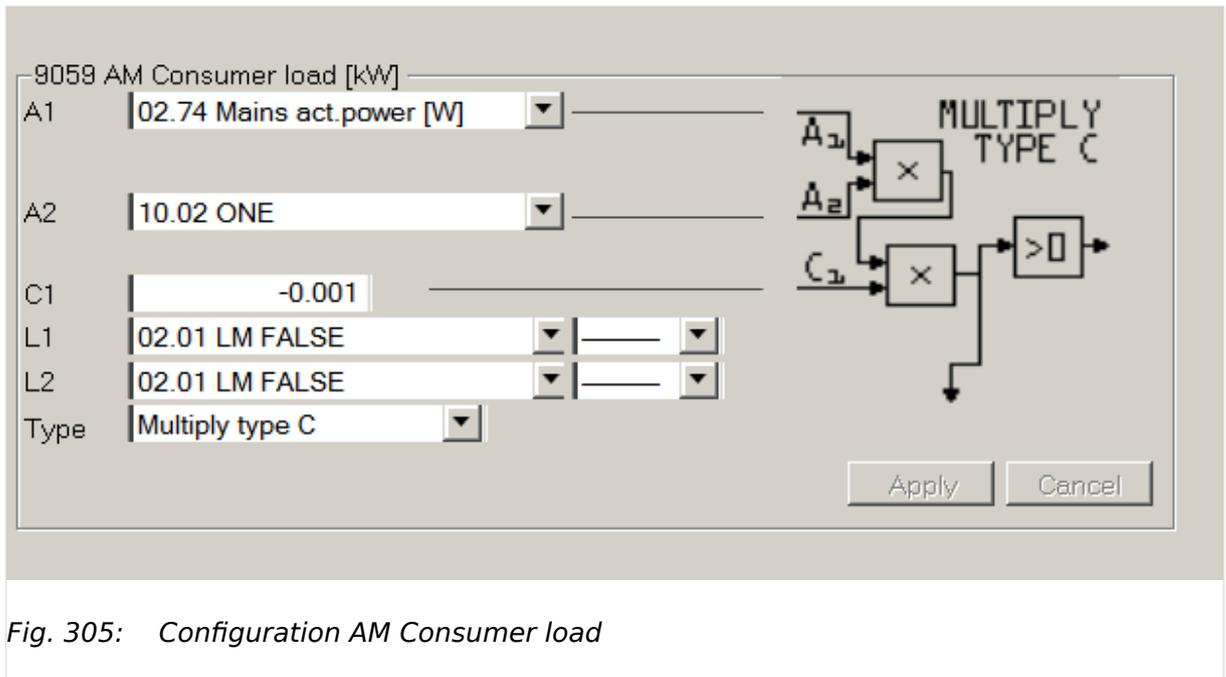
Fig. 305: Configuration AM Consumer load
