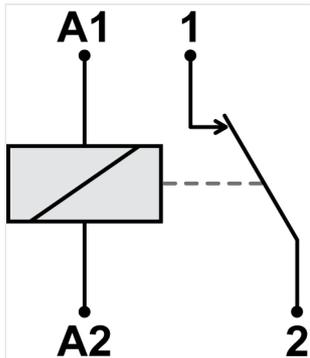
Fig. 164: Normally Closed contacts - schematic
