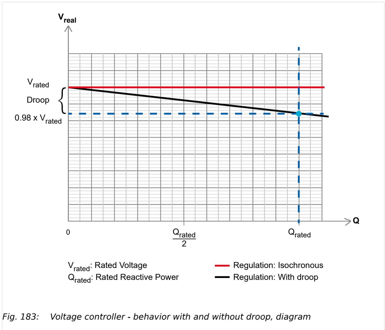
Fig. 183: Voltage controller - behavior with and without droop, diagram
