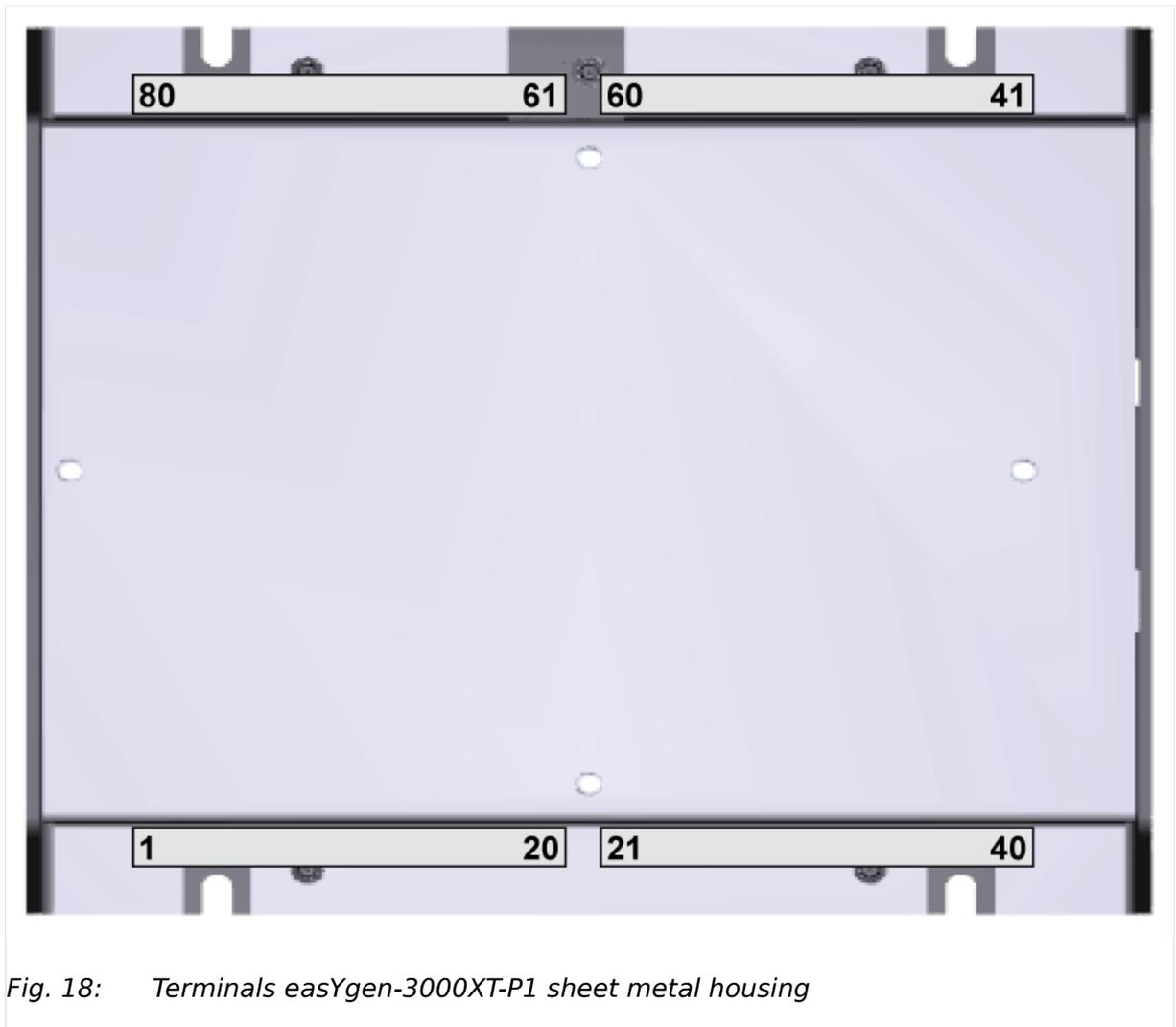
Fig. 18: Terminals easYgen-3000XT-P1 sheet metal housing
