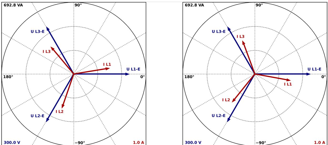
Fig. 60: Phasor diagram: capacitive load (left) and inductive load (right)
