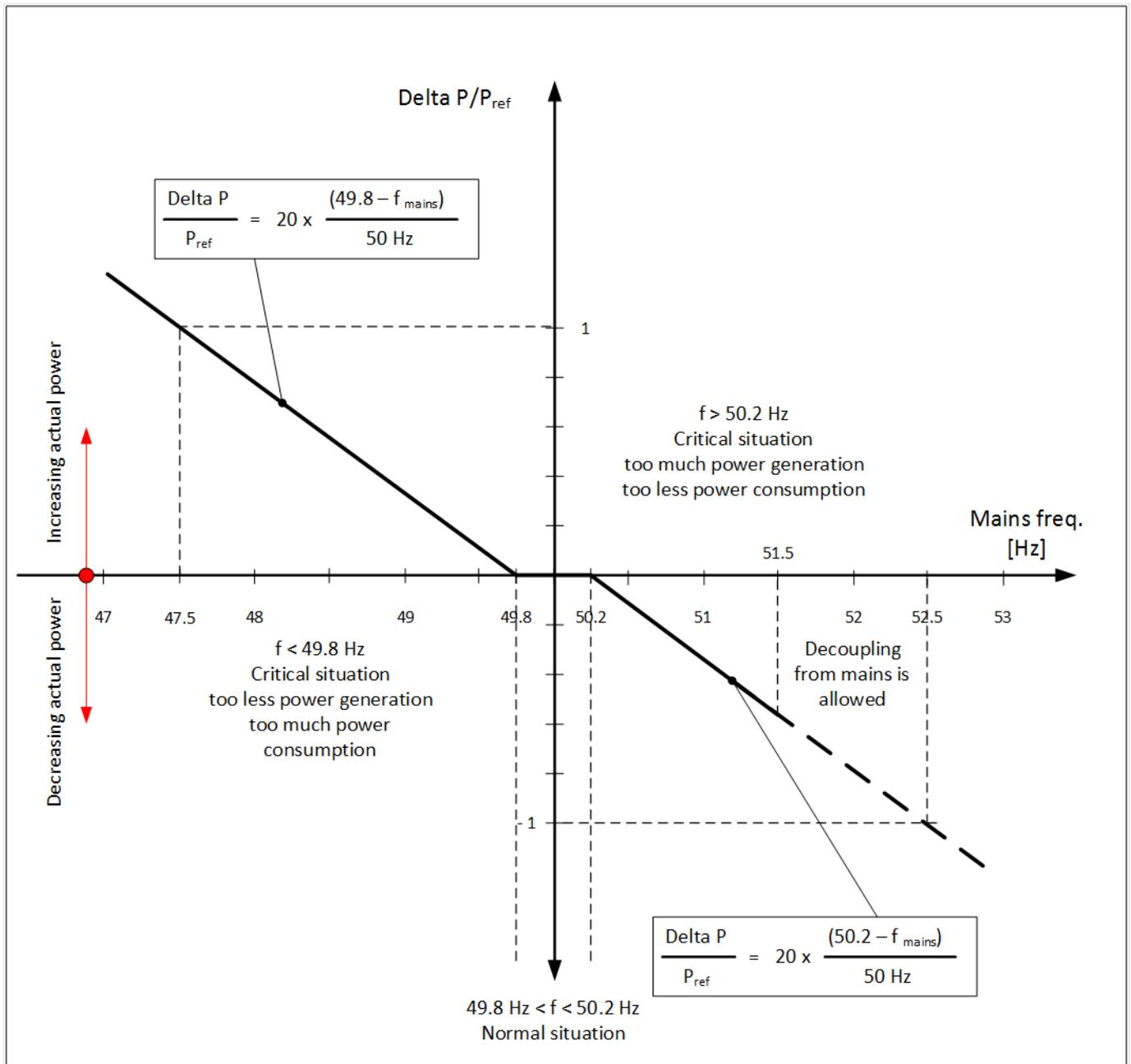
Fig. 185: De/Up-rating of active power setpoint due mains stabilization
