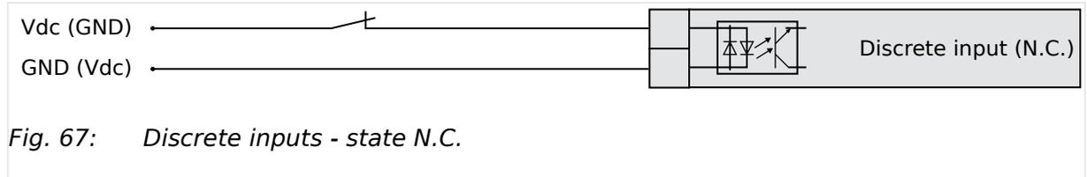
Fig. 67: Discrete inputs - state N.C.
