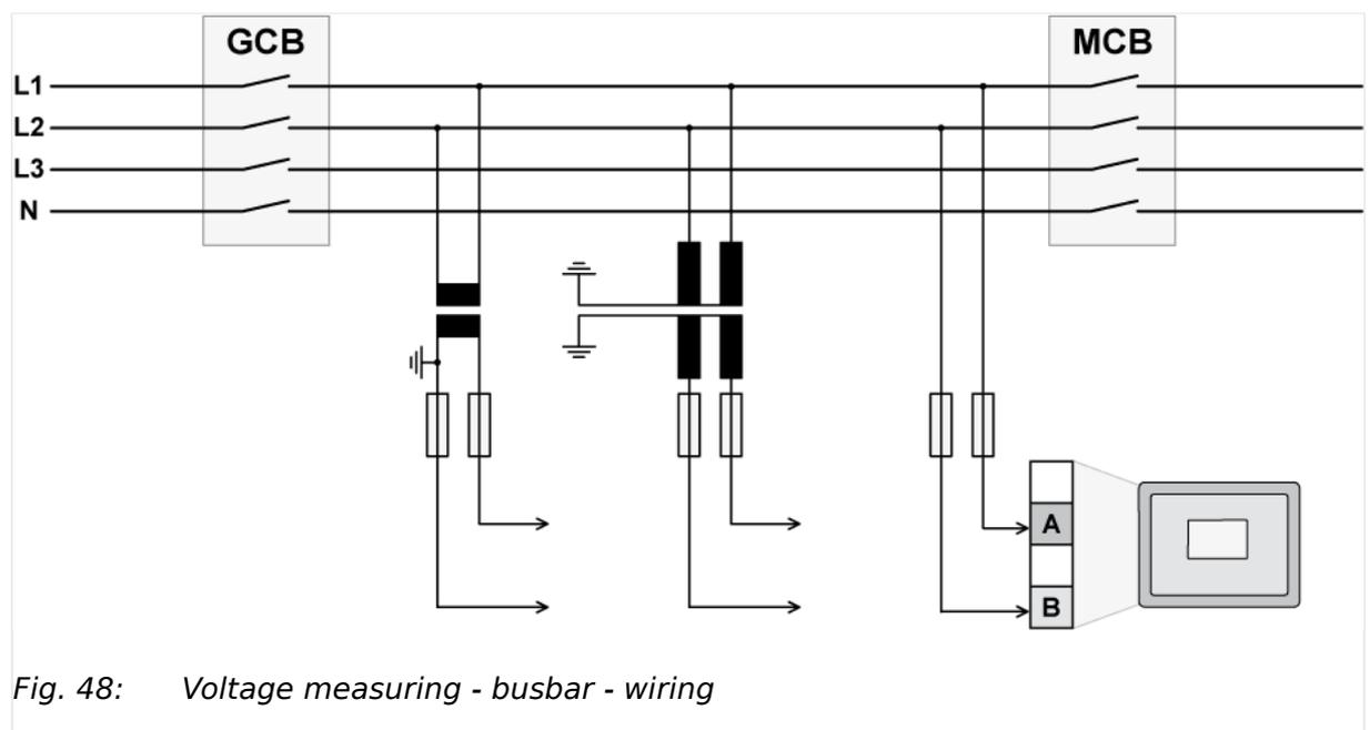
Fig. 48: Voltage measuring - busbar - wiring
