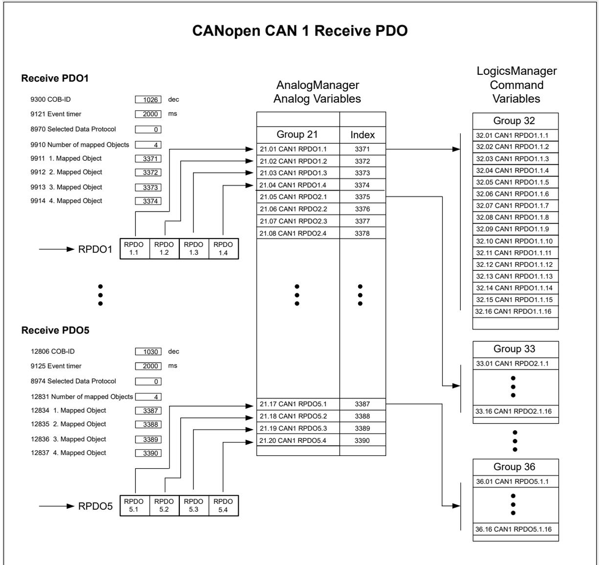
Fig. 389: Example of a CAN 1 RPDO configuration for interconnectivity.
