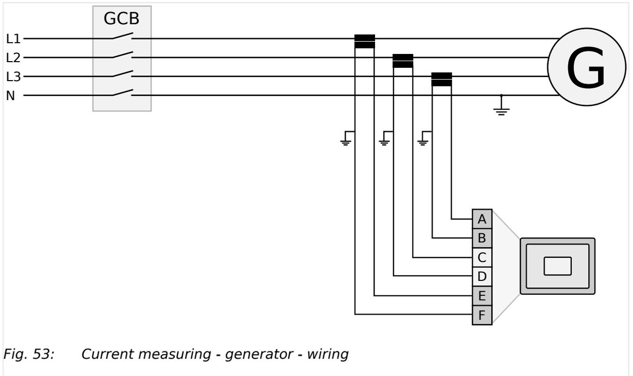
Fig. 53: Current measuring - generator - wiring
