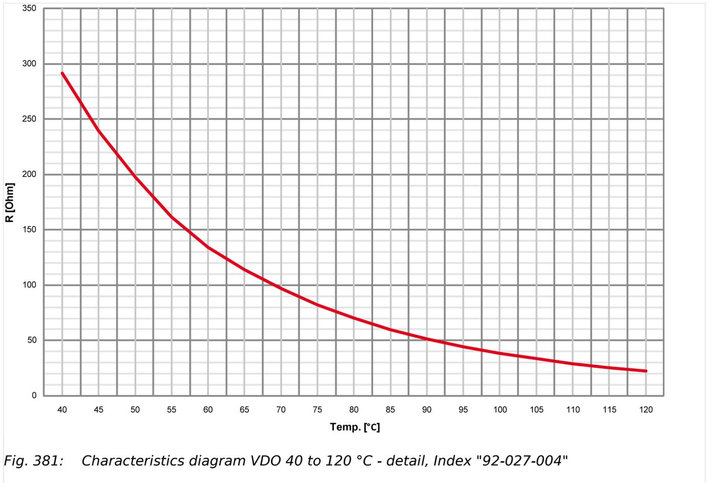
Fig. 381: Characteristics diagram VDO 40 to 120 °C - detail, Index "92-027-004"
