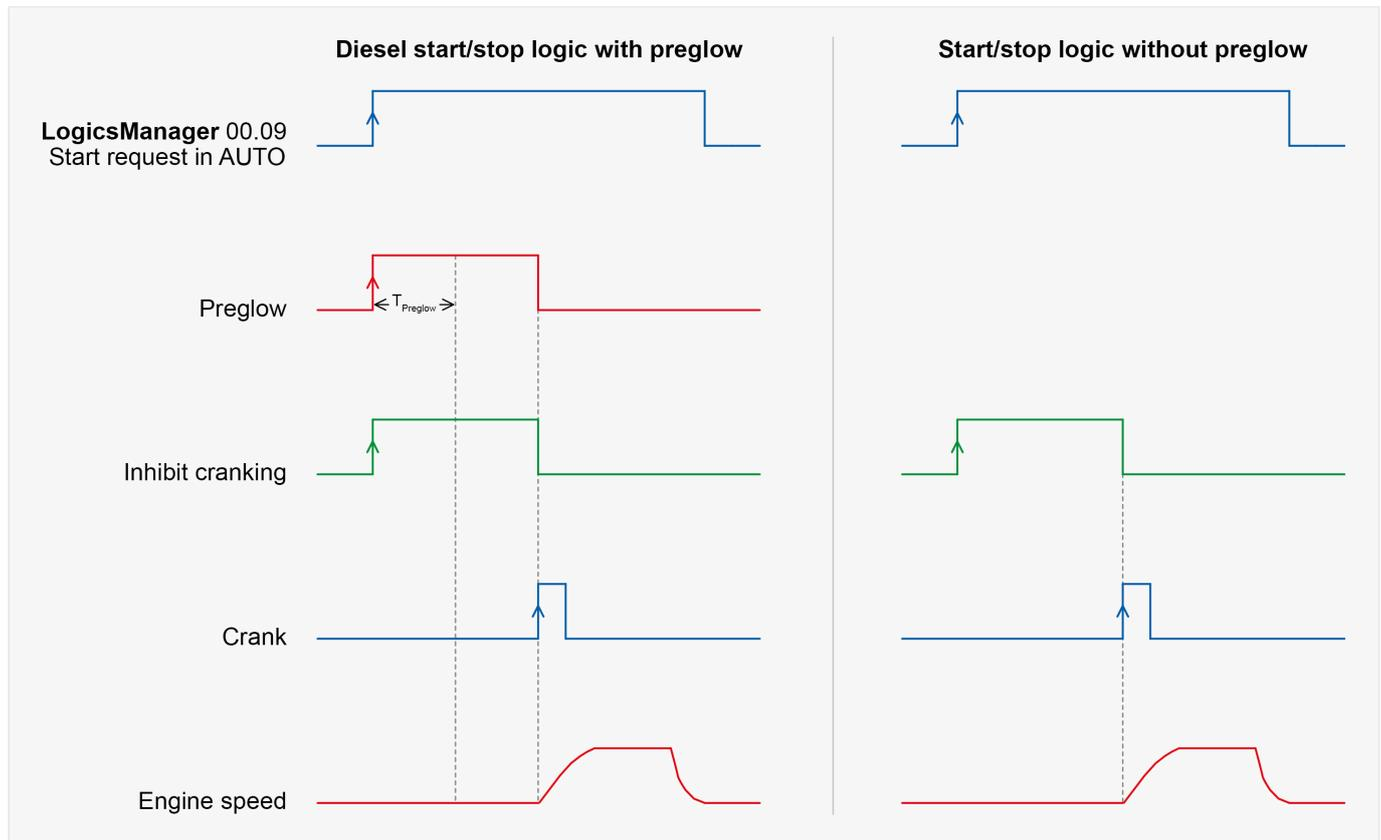
Fig. 156: Engine - start/stop logic (inhibit cranking)
