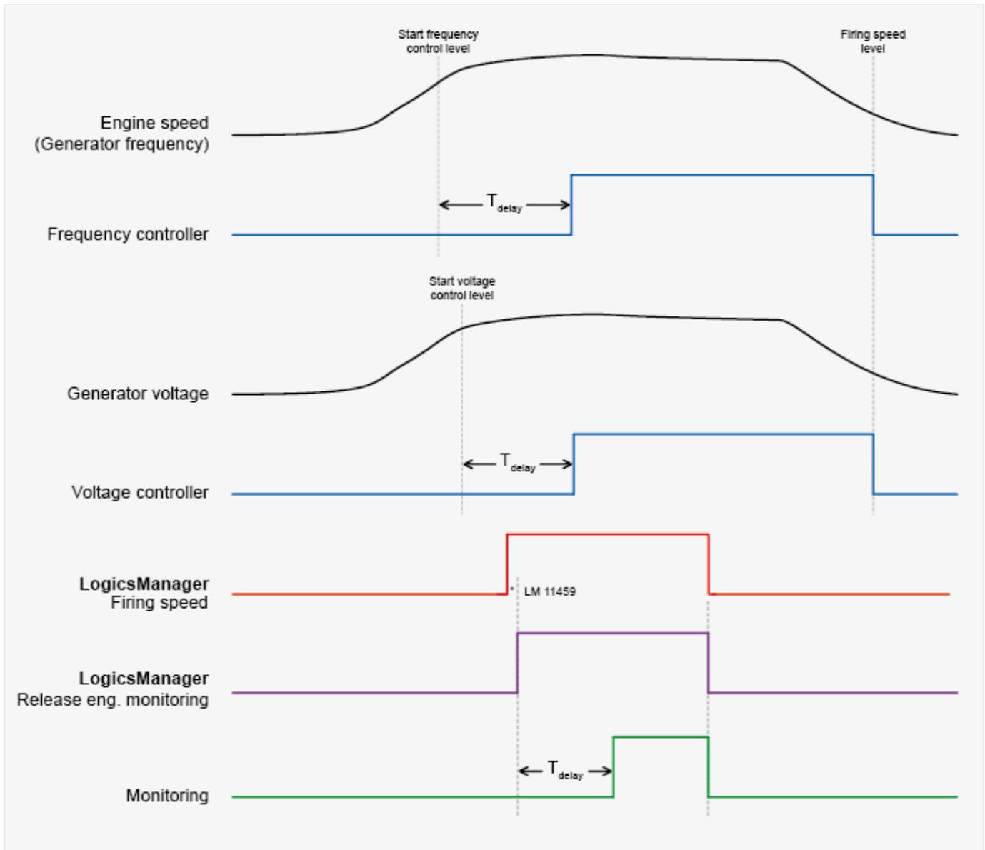
Fig. 288: Start/Stop sequence - LogicsManager "Firing speed detection"
