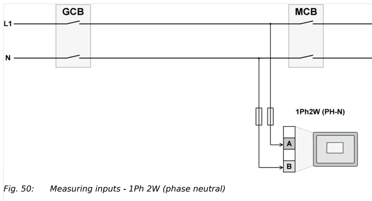
Fig. 50: Measuring inputs - 1Ph 2W (phase neutral)
