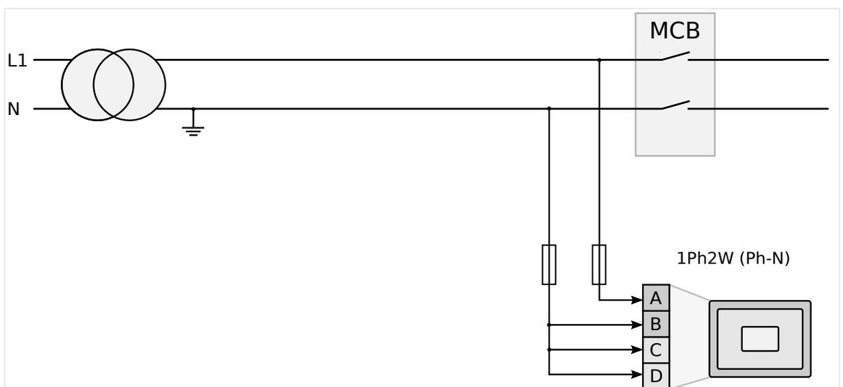
Fig. 45: Measuring inputs - 1Ph 2W (phase neutral)
