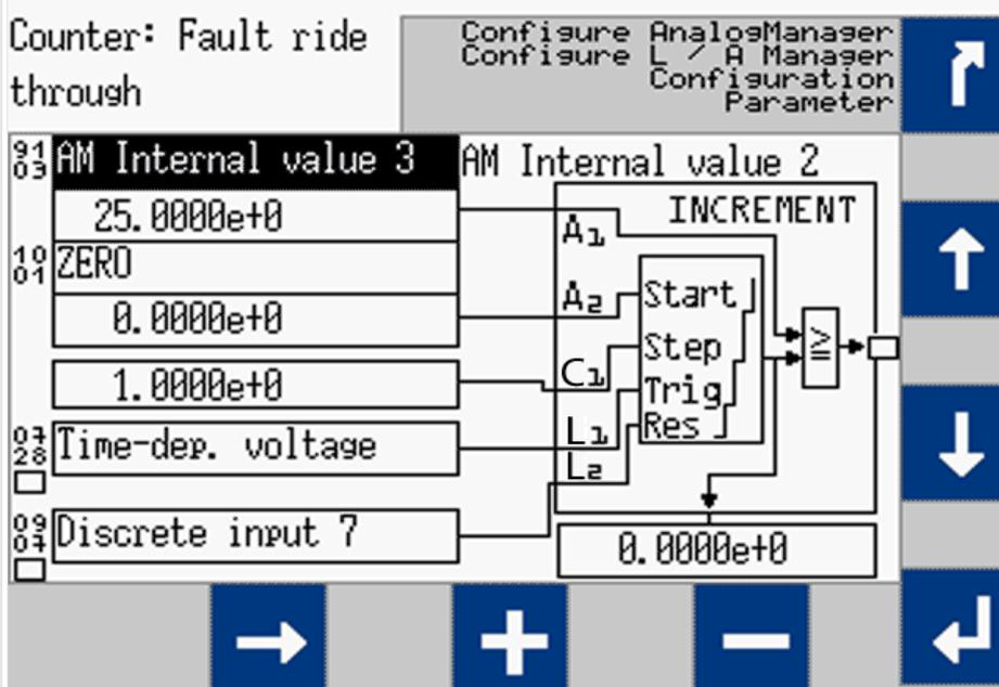
Fig. 225: screen shot HMI: AM increment sample
