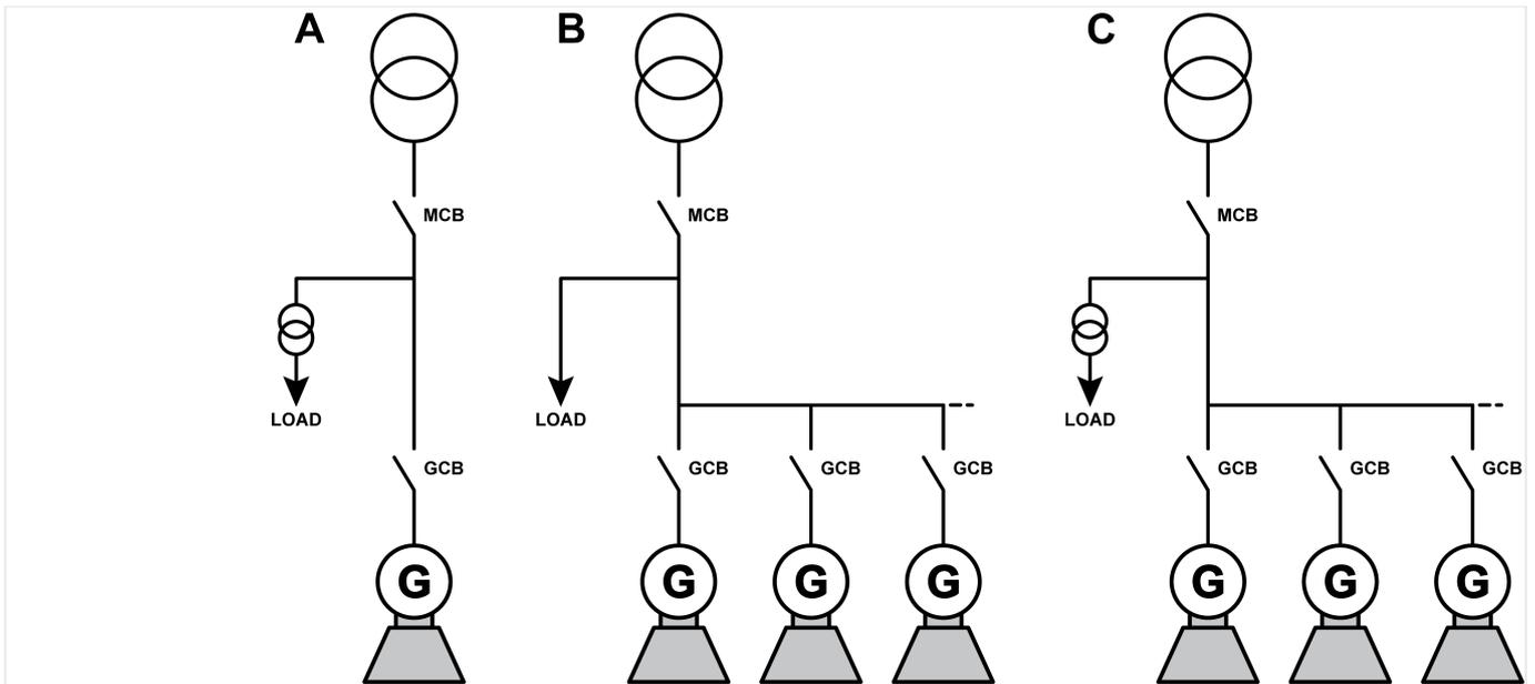
Fig. 297: Run-up synchronization examples
