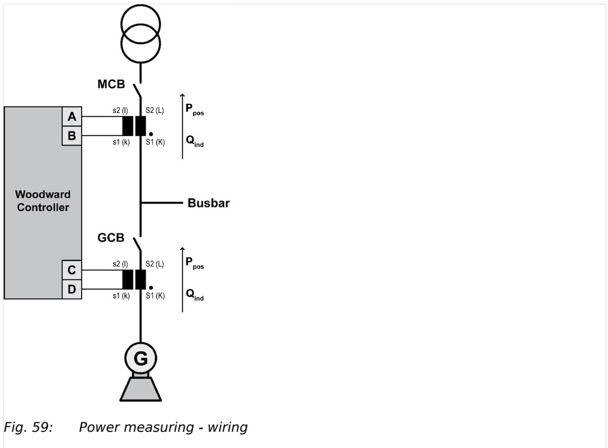
Fig. 59: Power measuring - wiring
