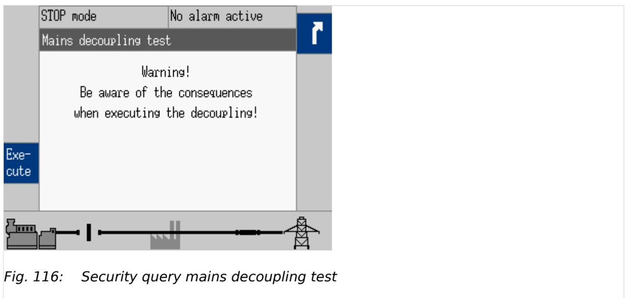
Fig. 116: Security query mains decoupling test
