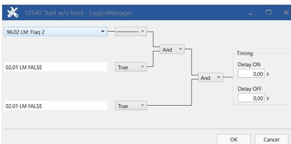
Fig. 262: LogicsManager function "Start without load"
