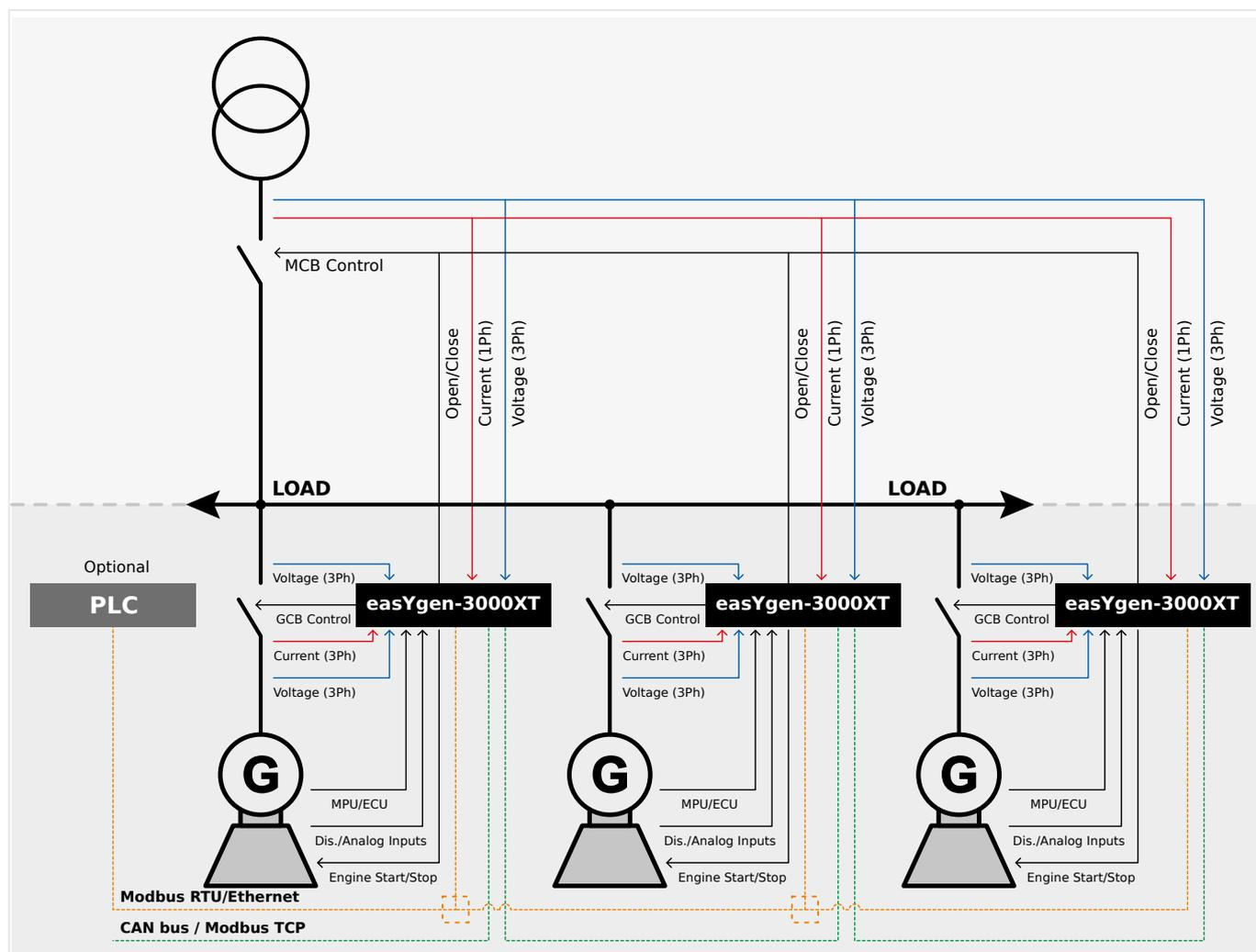
Fig. 242: Multiple genset application (schematic)
