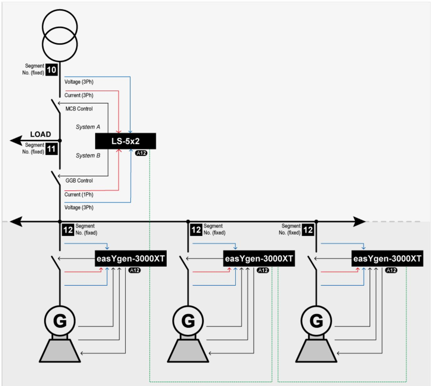
Fig. 239: Application mode A12 (schematic)
