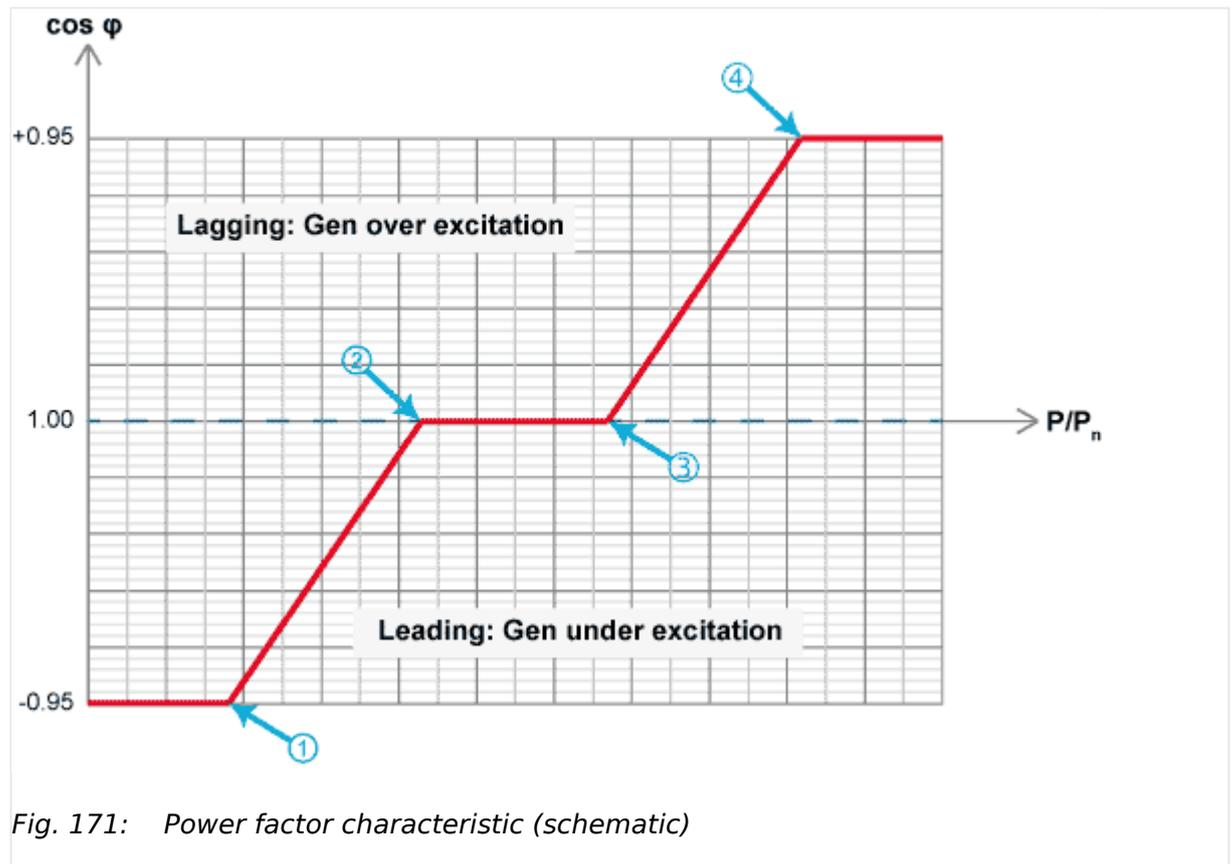
The characteristic is defined by four points (① .. ④). The power factor corresponding to this characteristic is available as data source 05.29 in the AnalogManager.
