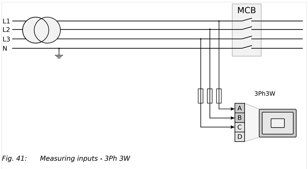
Fig. 41: Measuring inputs - 3Ph 3W
