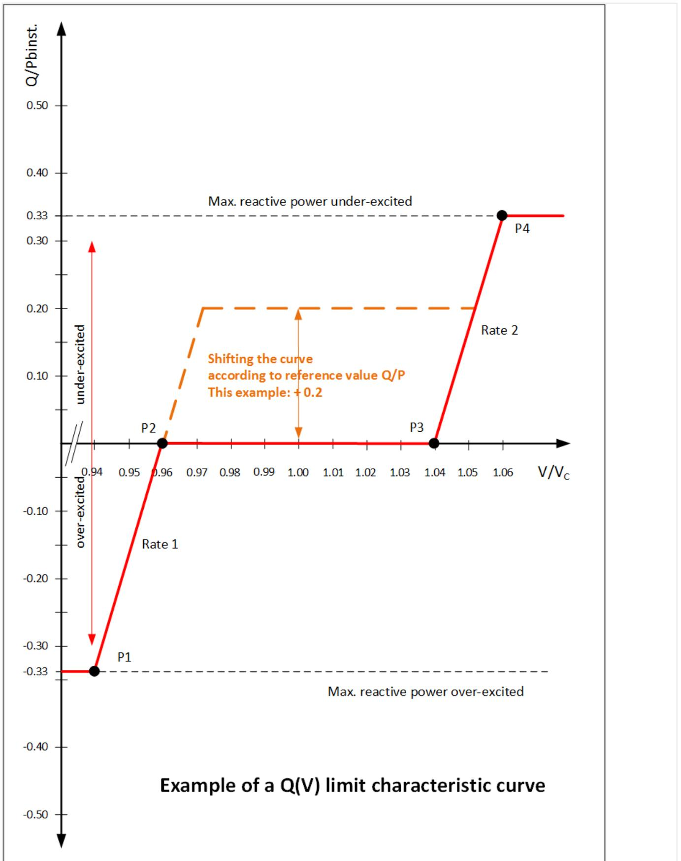
Fig. 177: Example of a Q(V) limit characteristic
