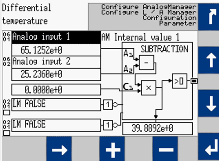
Fig. 224: screen shot HMI: AM subtraction sample
