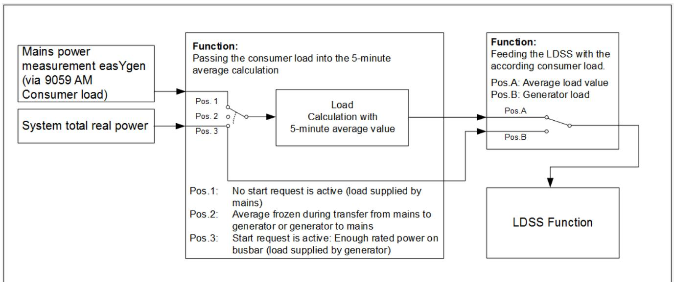
Fig. 306: Schematic of a predicted load with „internal“ source handling
