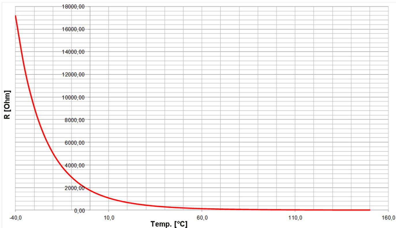
Fig. 382: Characteristics diagram VDO -40 to 120 °C - full range, Index "92-027-004"
