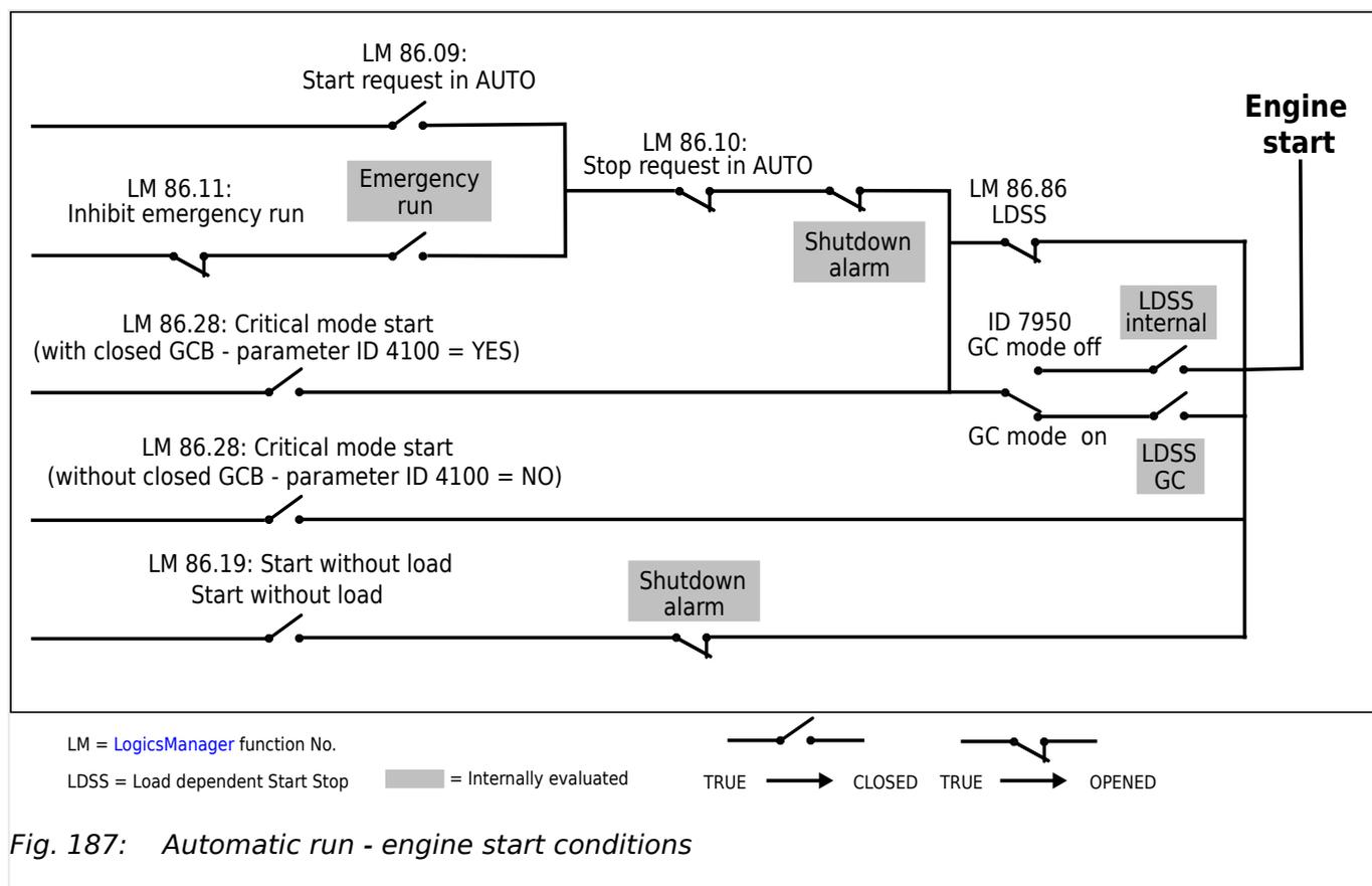
Fig. 187: Automatic run - engine start conditions
