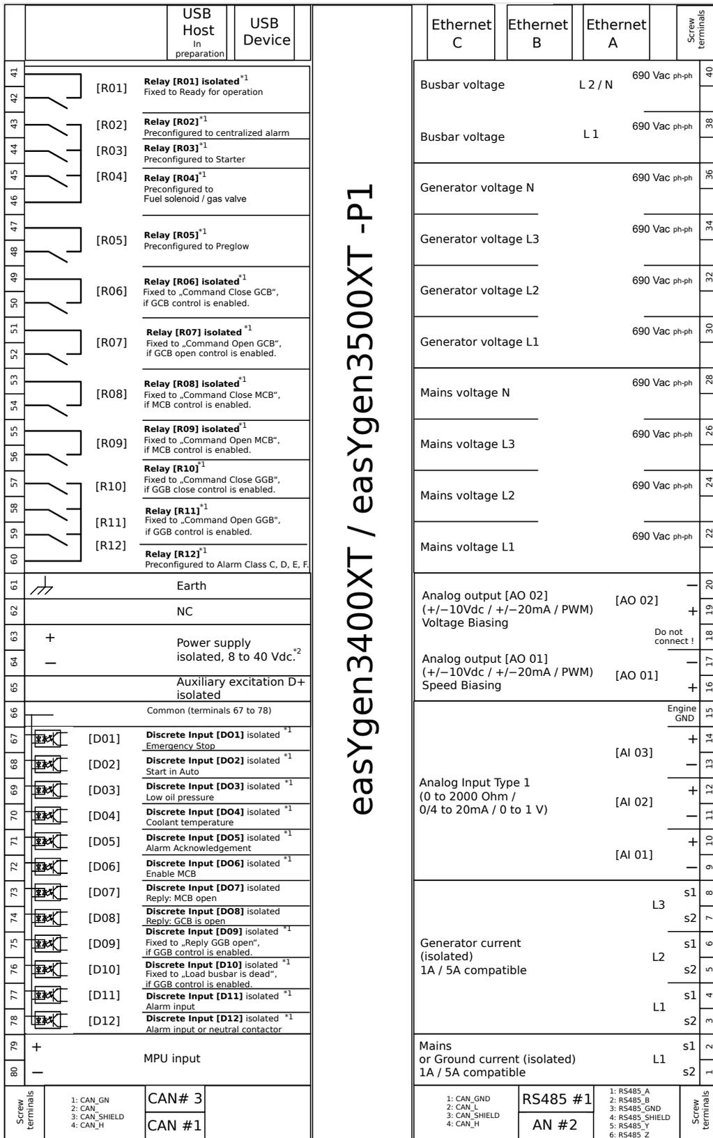
Subject to technical modifications configurable via Logics Manager<sup>\*1</sup> easYgen-3000XT Series Wiring Diagram PCB 1
