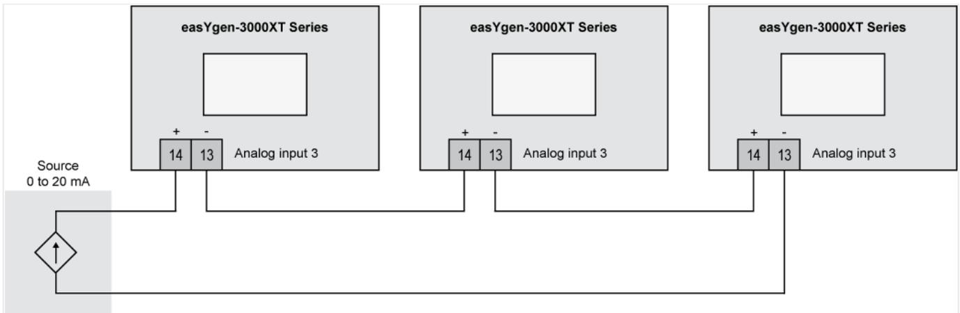
Fig. 277: Connecting analog inputs in series
