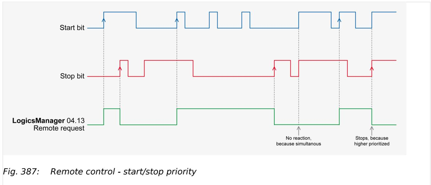
Fig. 387: Remote control - start/stop priority
