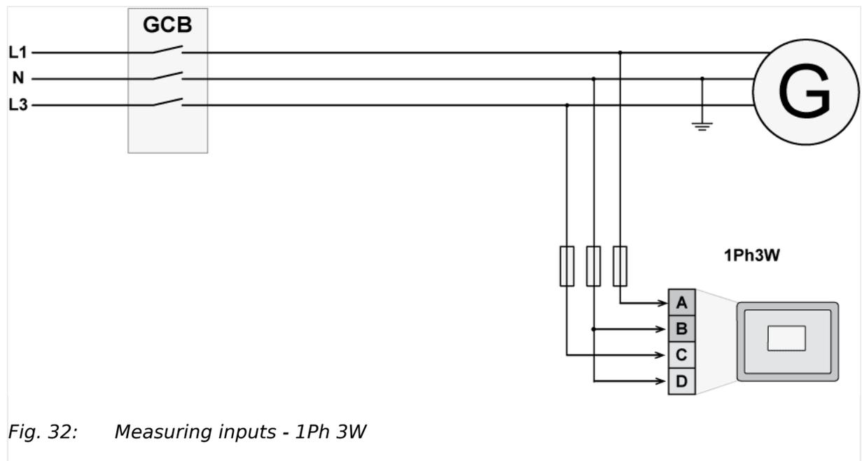
Fig. 32: Measuring inputs - 1Ph 3W
