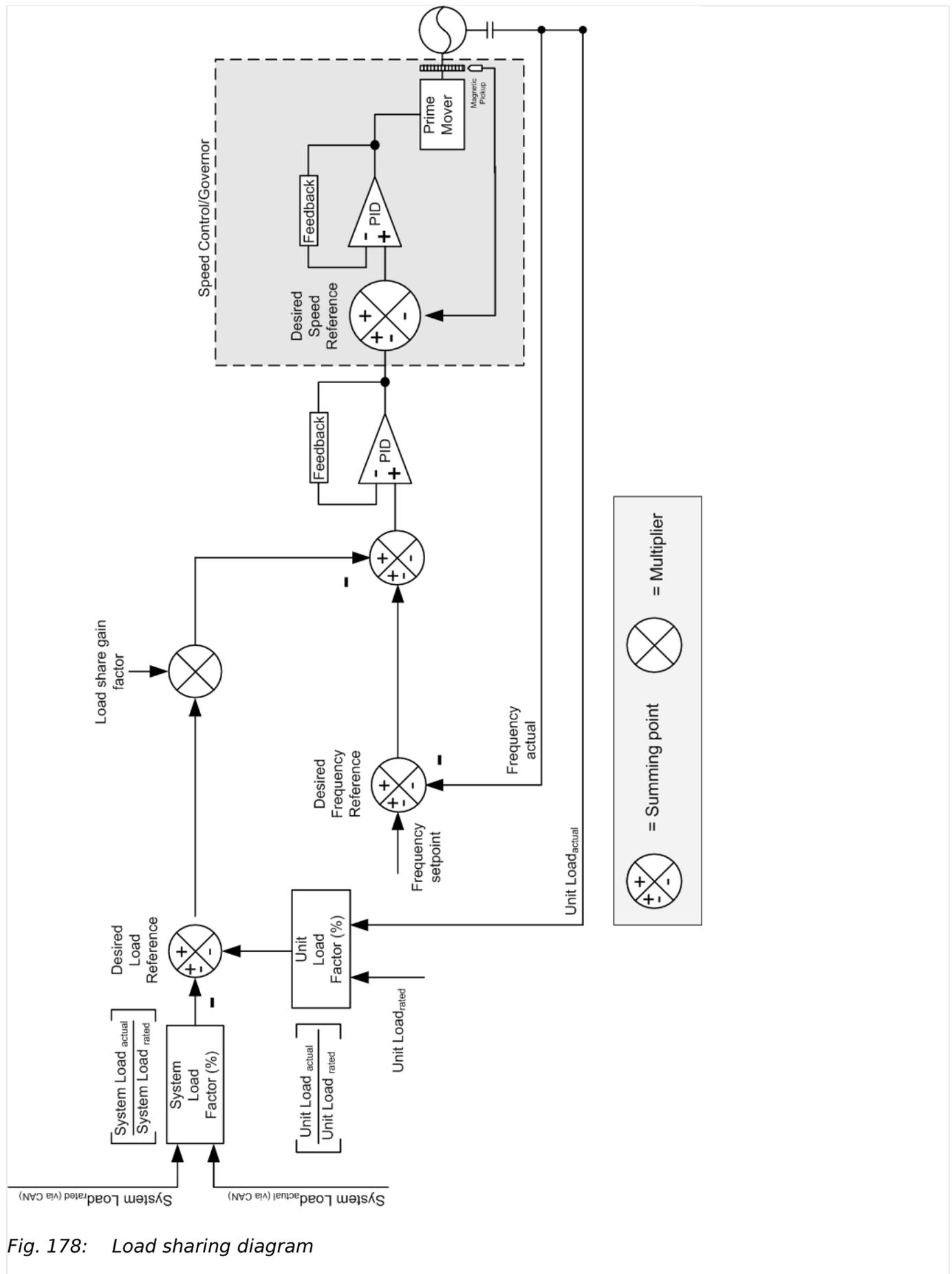
Fig. 178: Load sharing diagram
