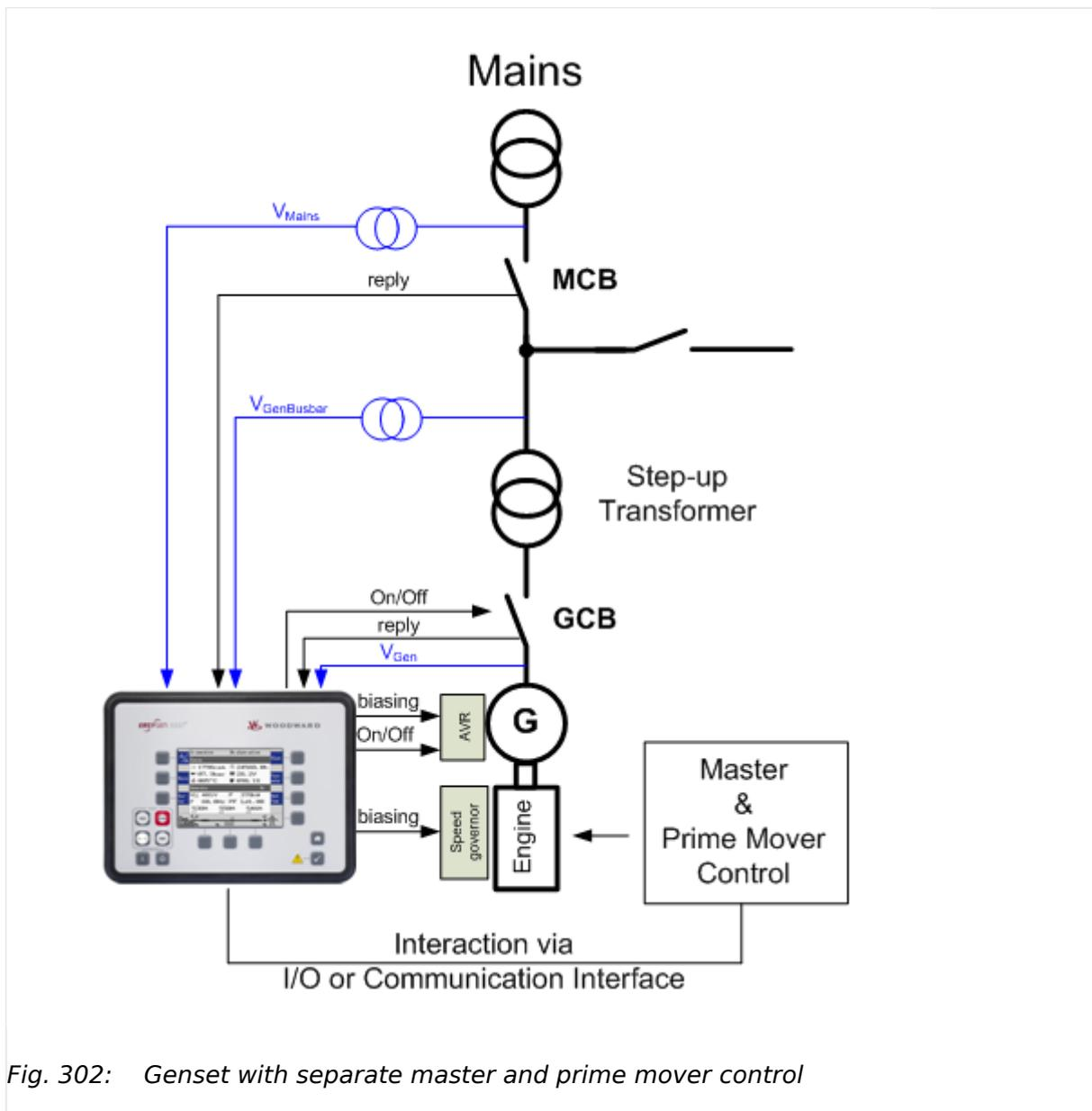
In this application the run up synchronization supports a GCB closure for magnetizing a power transformer. The engine is initiated for start and controlled by an independent control device. The easYgen can support this feature without any speed sensor input as long the Start/Stop mode logic (ID3321) is configured on "Off".
