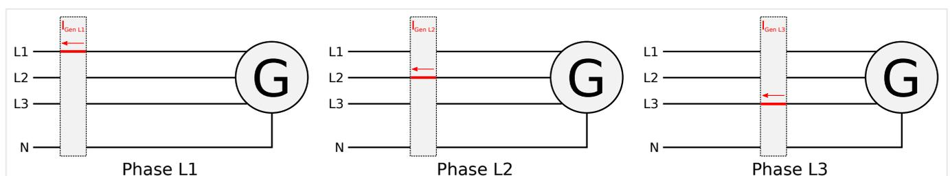
Fig. 55: Current measuring - generator, 'Phase L1' 'Phase L2' 'Phase L3'
