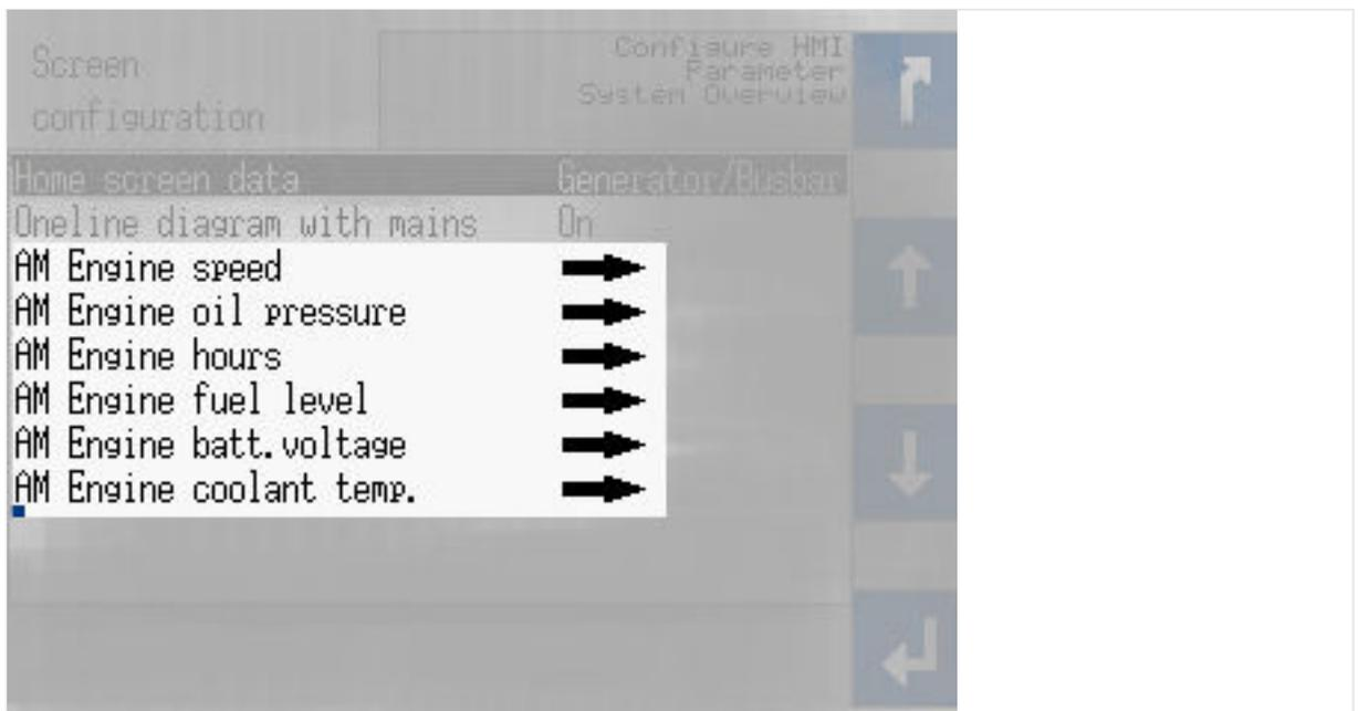
Fig. 88: AnalogManagers for "Engine" values at Home Screen
