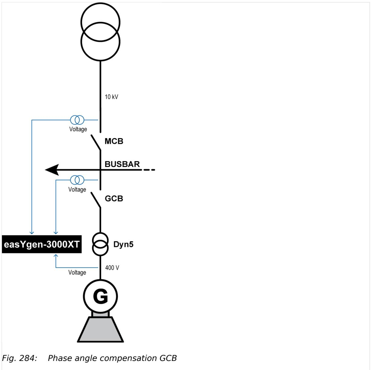
Fig. 284: Phase angle compensation GCB
