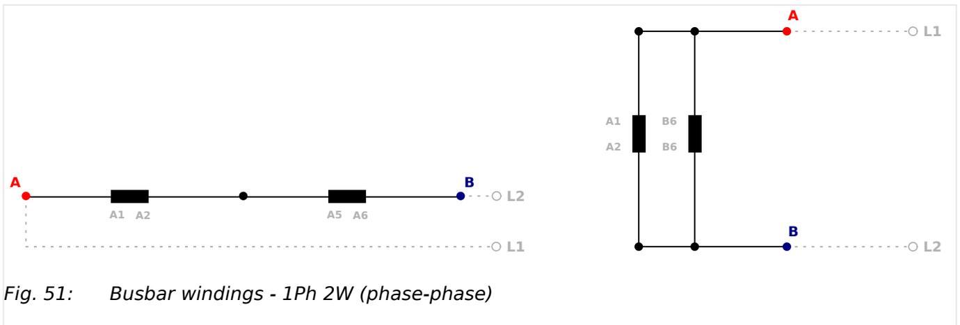
Fig. 51: Busbar windings - 1Ph 2W (phase-phase)
