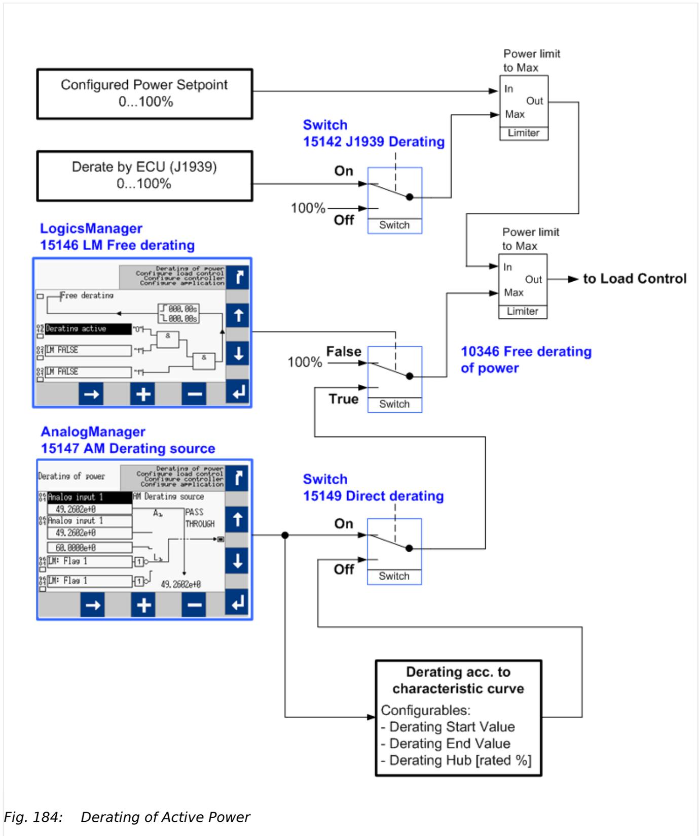
Fig. 184: Derating of Active Power
