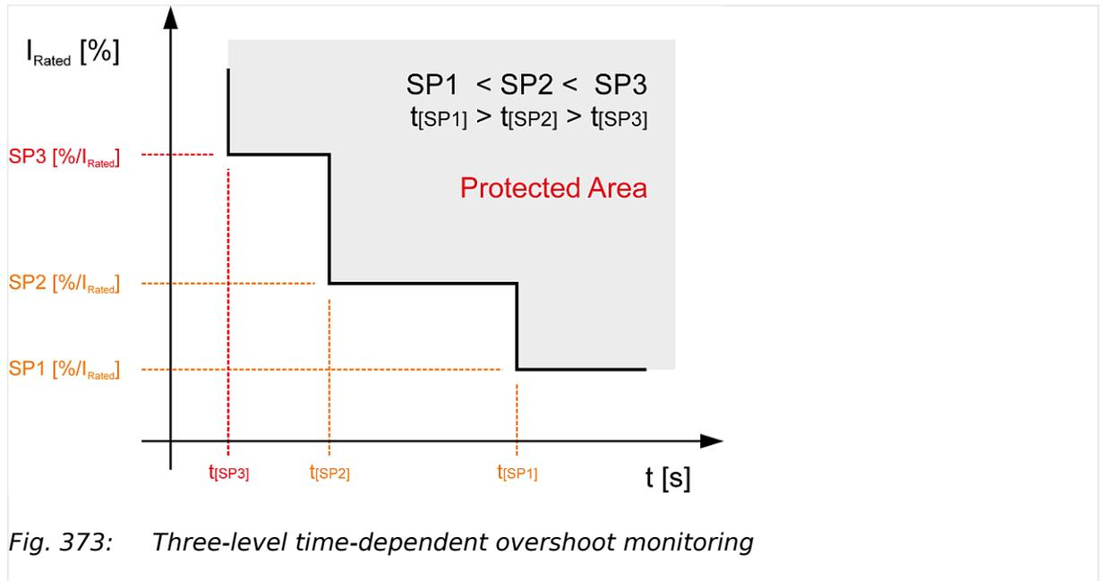
Fig. 373: Three-level time-dependent overshoot monitoring
