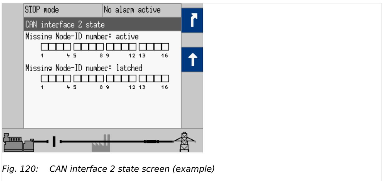
Fig. 120: CAN interface 2 state screen (example)
