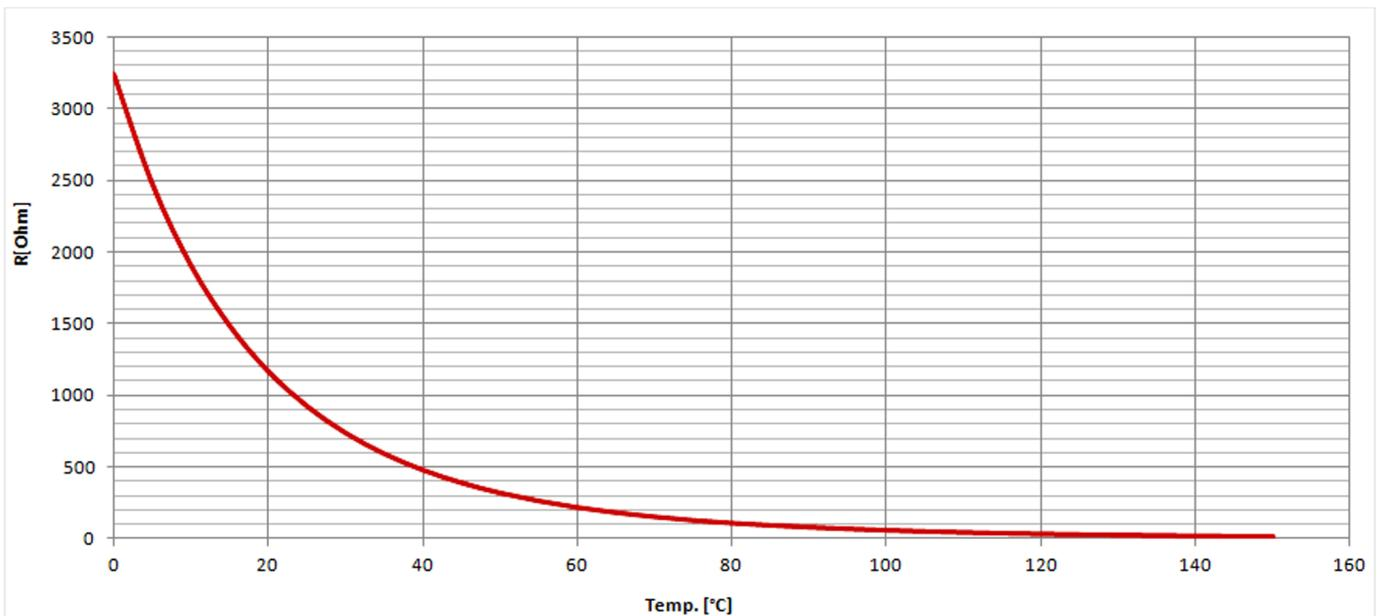
Fig. 384: Characteristics diagram VDO 0 to 120 °C - full range, Index "92-027-006"
