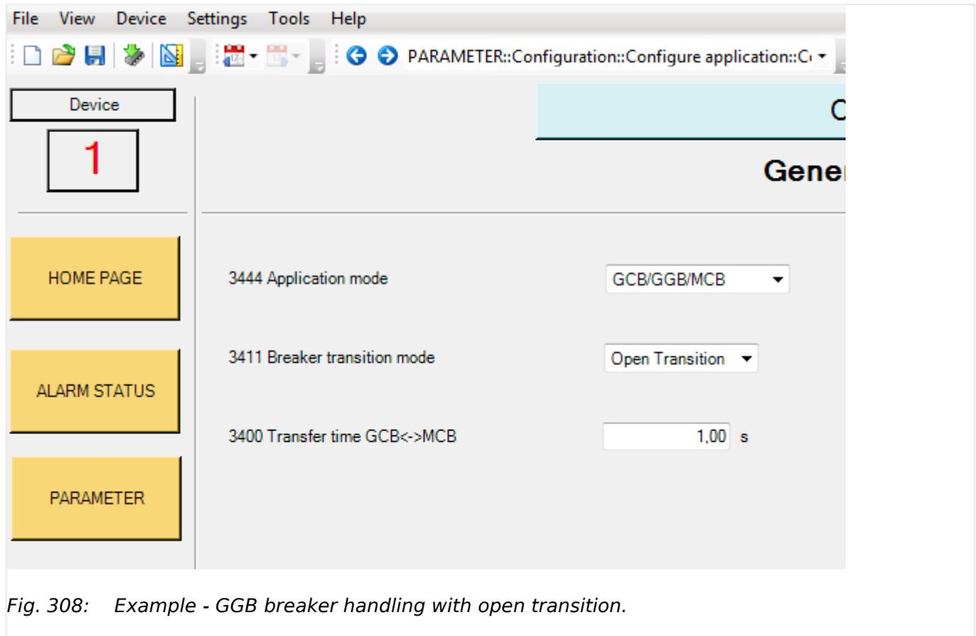
Fig. 308: Example - GGB breaker handling with open transition.
