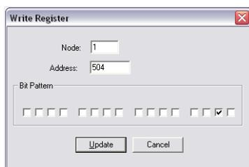
Fig. 317: Modbus - write register - stop request
