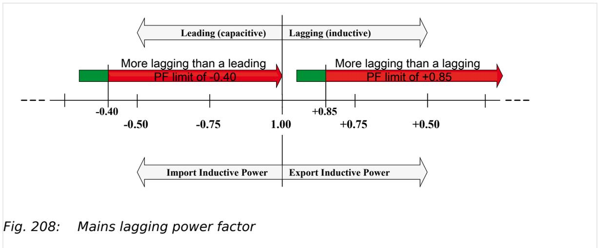
Fig. 208: Mains lagging power factor
