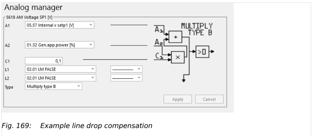
Fig. 169: Example line drop compensation
