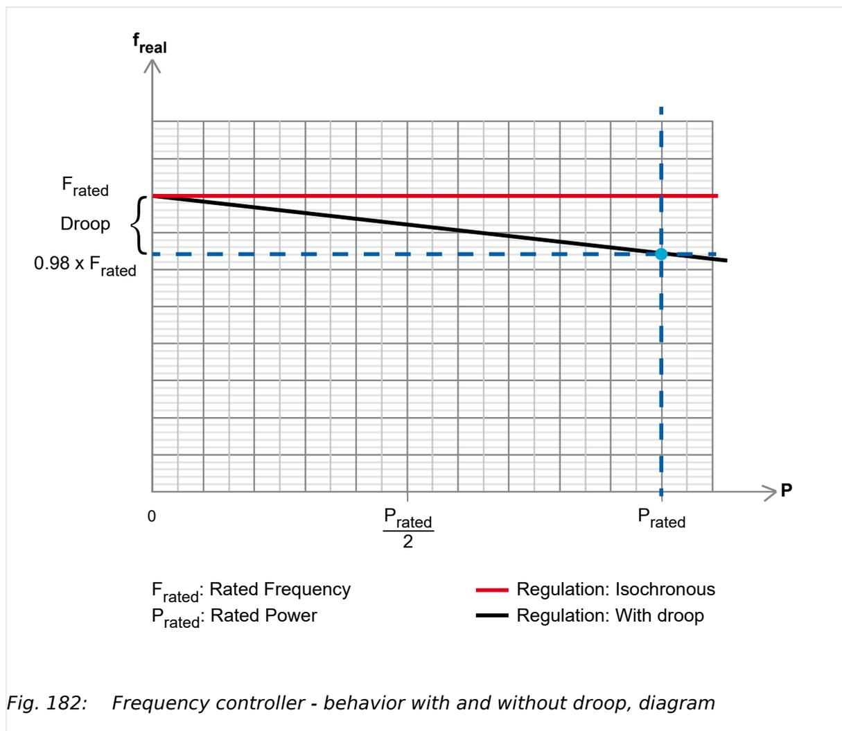
Fig. 182: Frequency controller - behavior with and without droop, diagram
