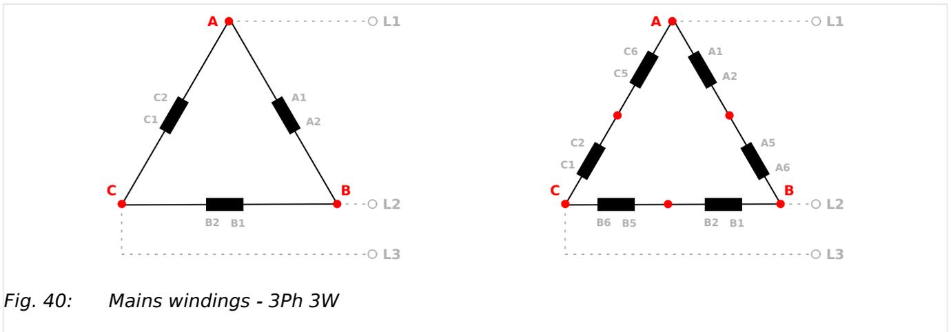
Fig. 40: Mains windings - 3Ph 3W
