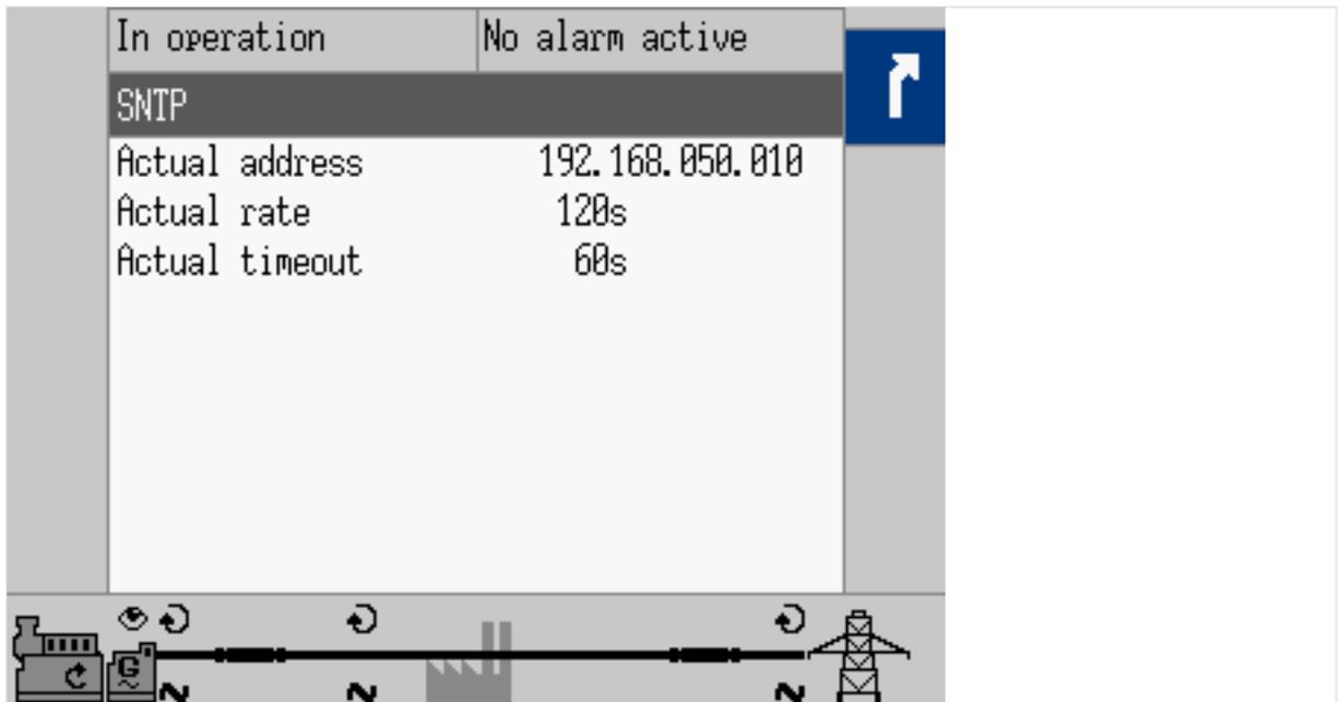
Fig. 127: Ethernet SNTP (example)
