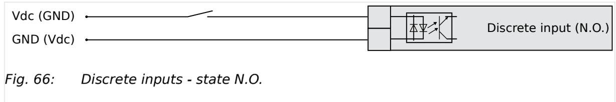
Fig. 66: Discrete inputs - state N.O.
