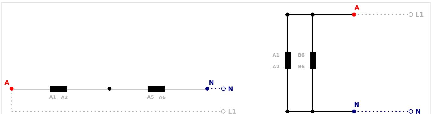
Fig. 44: Mains windings - 1Ph 2W (phase neutral)
