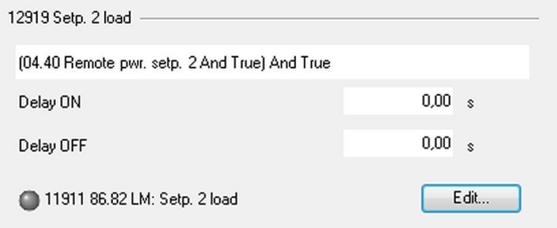
Fig. 331: Remotely switch Setp. 2 load
