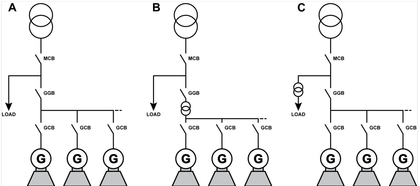
Fig. 298: Run-up synchronization examples
