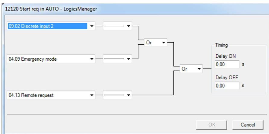
Fig. 307: Including the emergency mode as starting argue.
