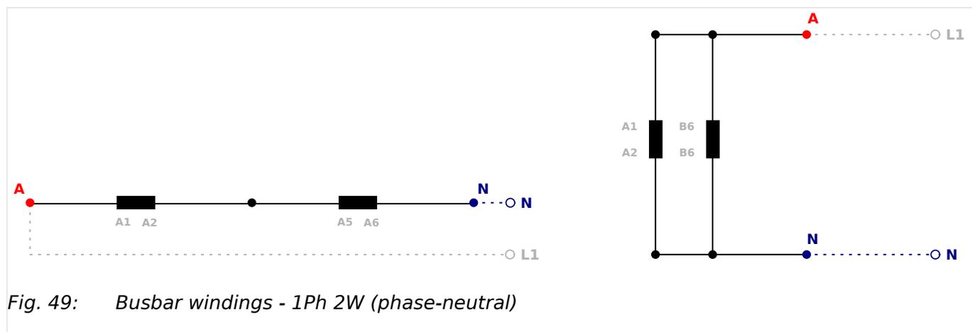
Fig. 49: Busbar windings - 1Ph 2W (phase-neutral)
