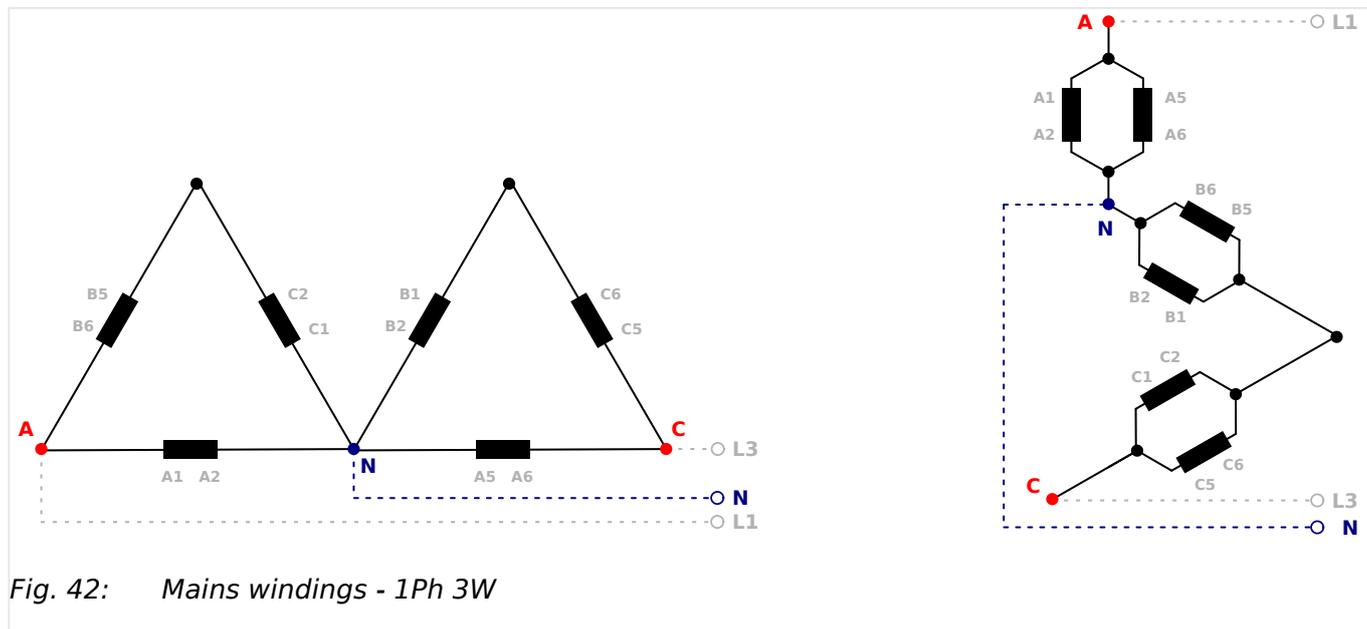
Fig. 42: Mains windings - 1Ph 3W
