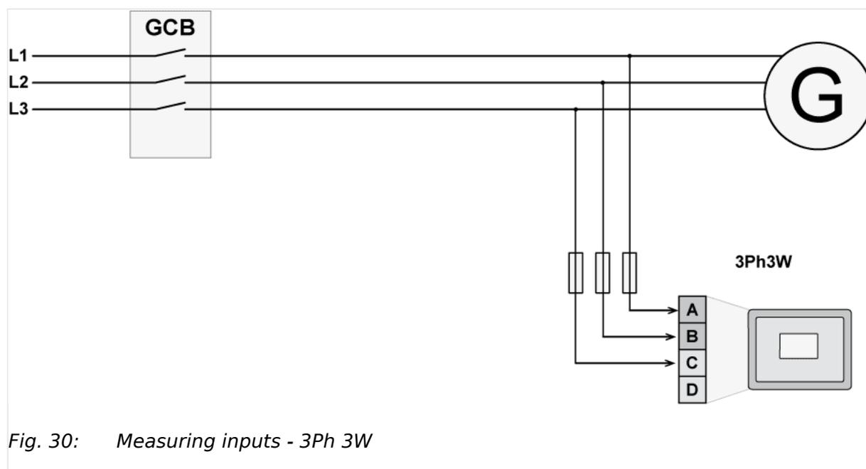
Fig. 30: Measuring inputs - 3Ph 3W
