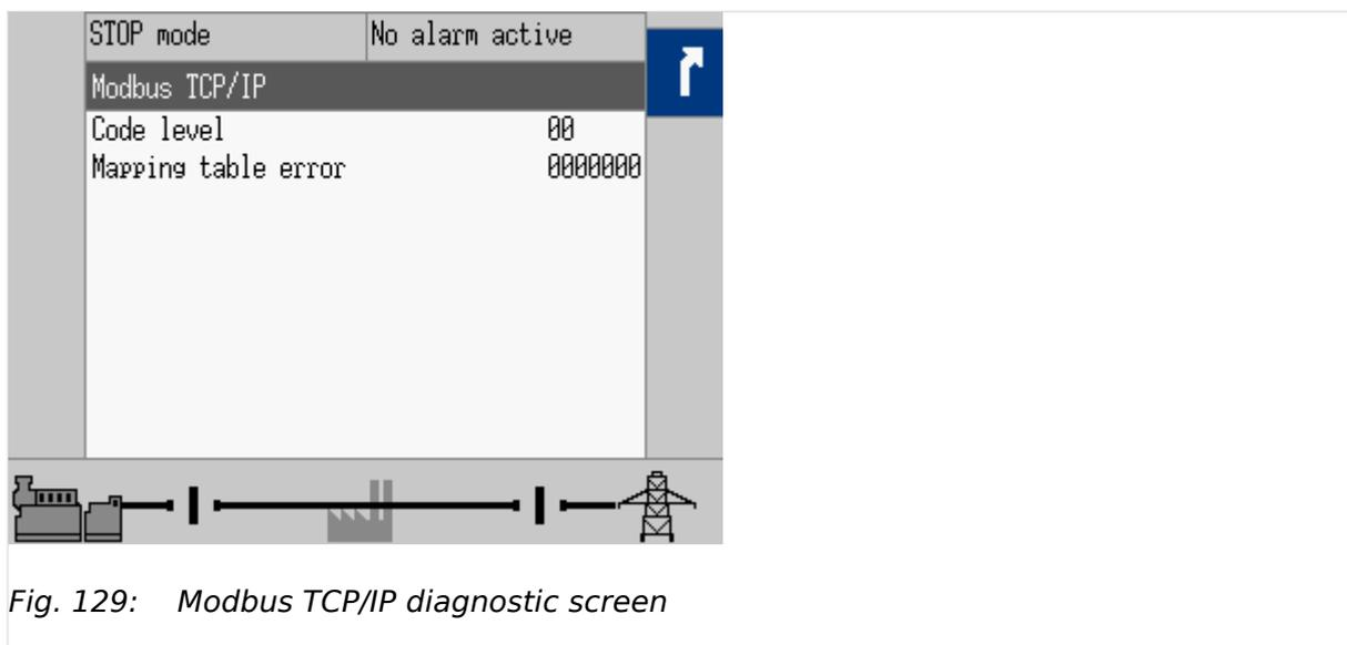
Fig. 129: Modbus TCP/IP diagnostic screen
