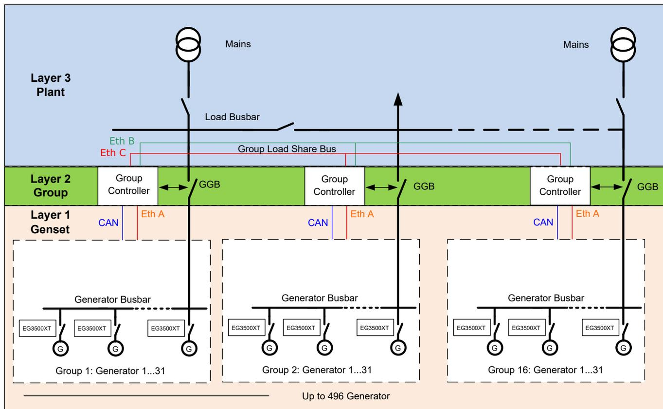
Fig. 241: Example application mode A13 with GC-application mode GGB/MCB
