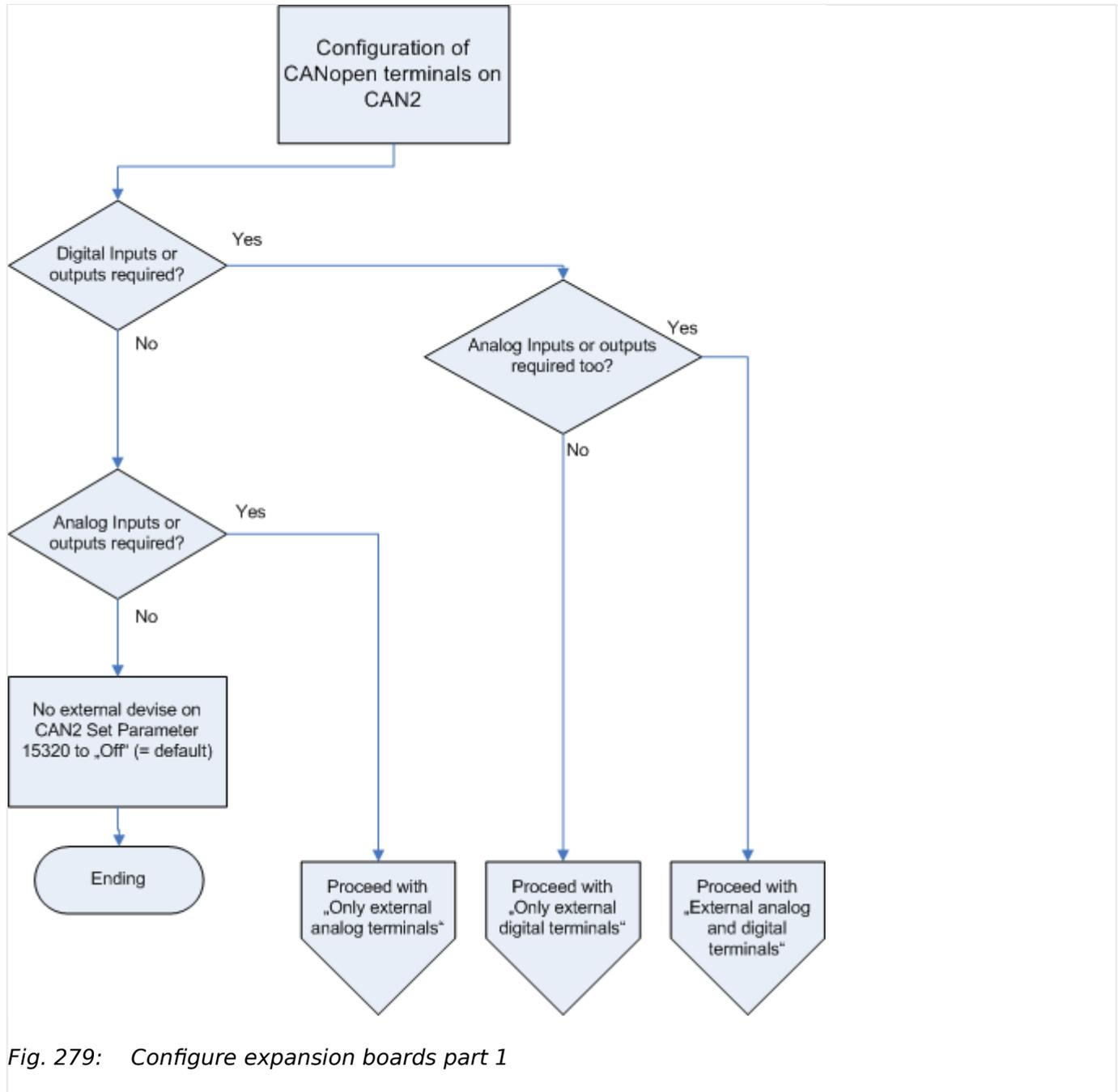
Fig. 279: Configure expansion boards part 1
