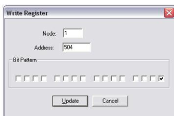
Fig. 316: Modbus - write register - start request
