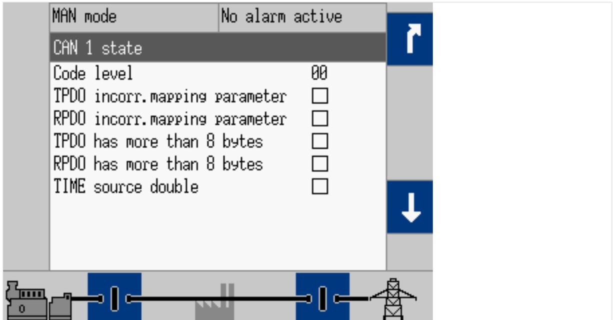
Fig. 117: CAN 1 state screen (example)
