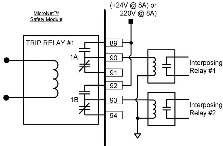
Figure 2-16d. Example Trip Relay Wiring (Voted Trip Relay Models)
