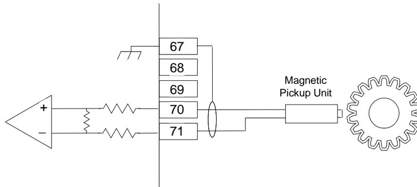
Figure 2-11a. Example MPU (Passive Magnetic Pickup Unit) Wiring
