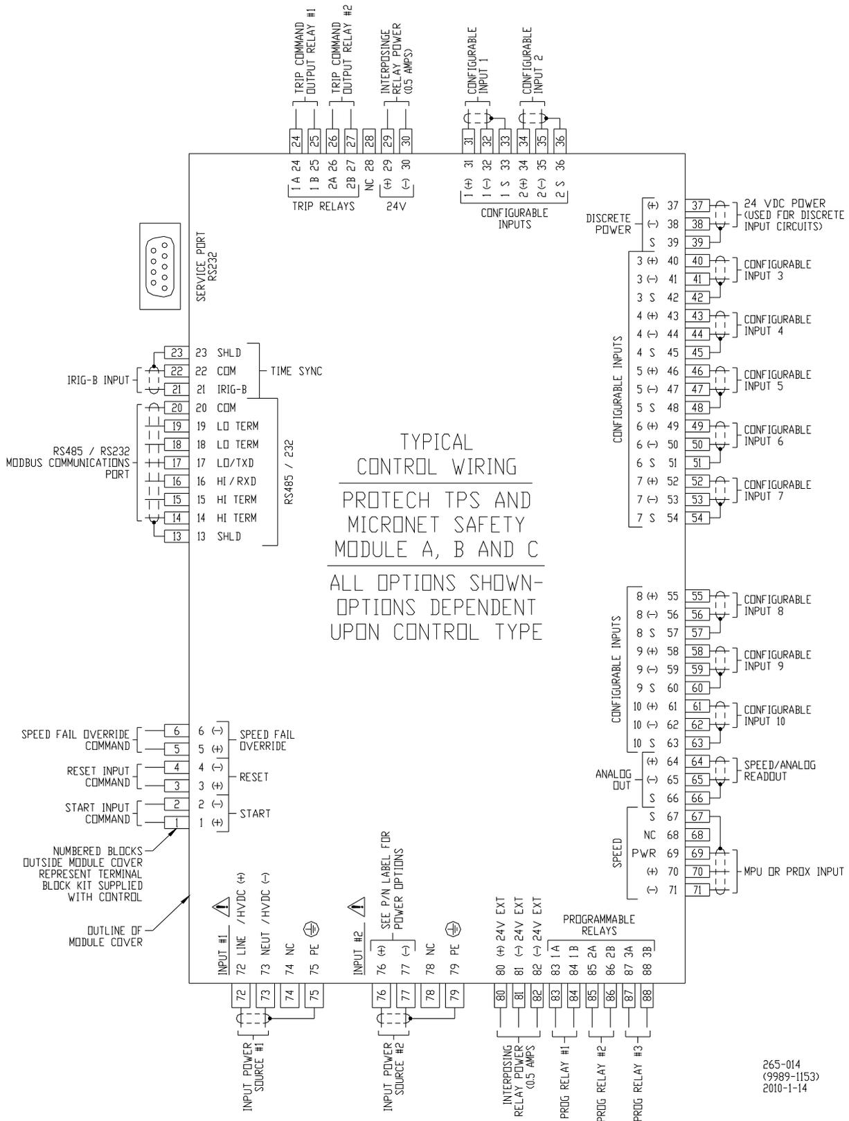
Figure 2-8. MicroNet Safety Module Control Wiring Diagram
