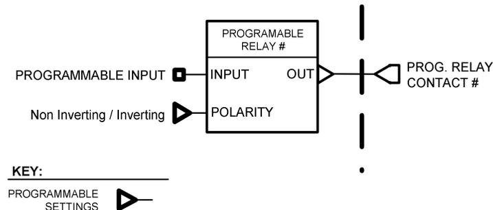
Figure 3-10. Programmable Relay Output Diagram
