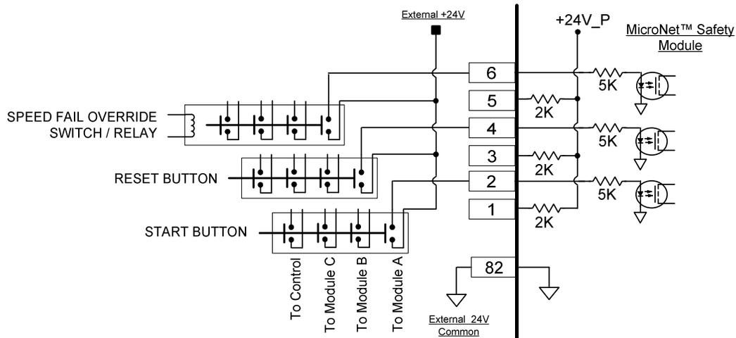
Figure 2-12b. Example Standard Discrete Input Wiring (External Power Option)
