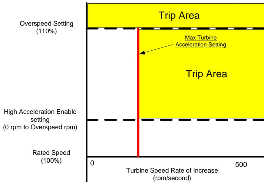
Figure 3-11. Over-Acceleration Enabling Diagram
