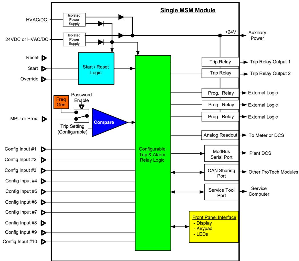
Figure 3-2. Functional Diagram of single MicroNet Safety Module with Independent Trip Relay Outputs
