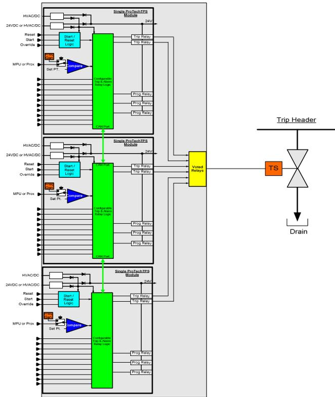
Figure 3-6. Simplex Trip Block Assembly
