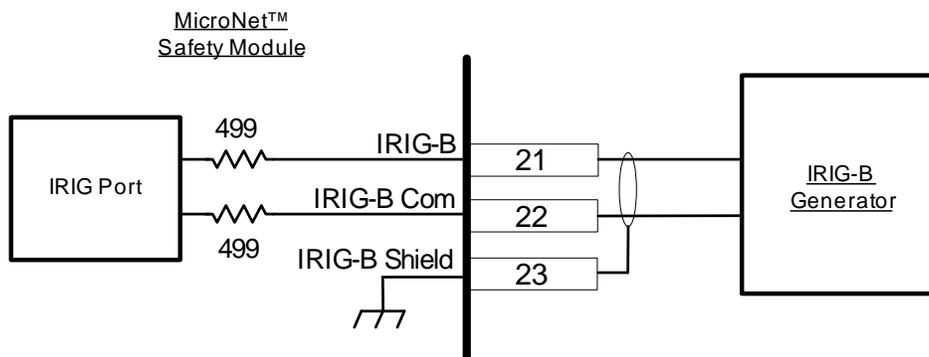
Figure 2-20. IRIG-B Interface Diagram
