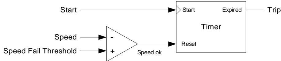
Figure 3-13. Speed Fail Timeout Trip Diagram
