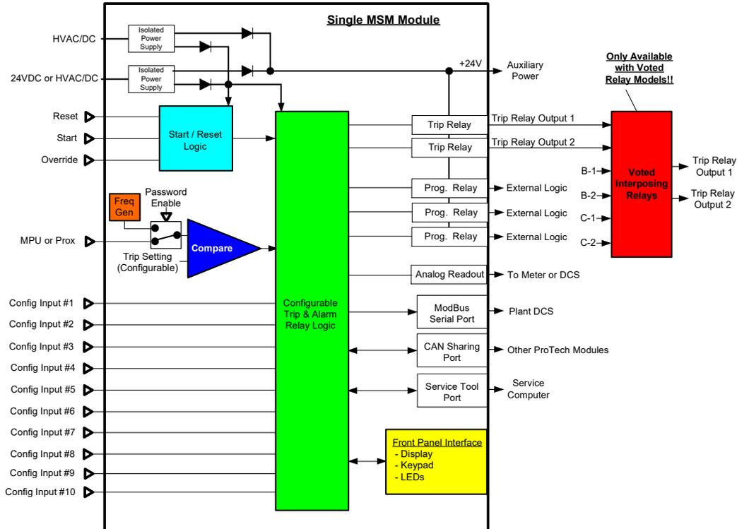
Figure 3-5. Functional Diagram of Single MicroNet Safety Module with Voted Trip Relay Outputs
