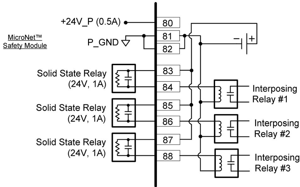
Figure 2-16f. Example Programmable Relay Wiring (External Supply)
