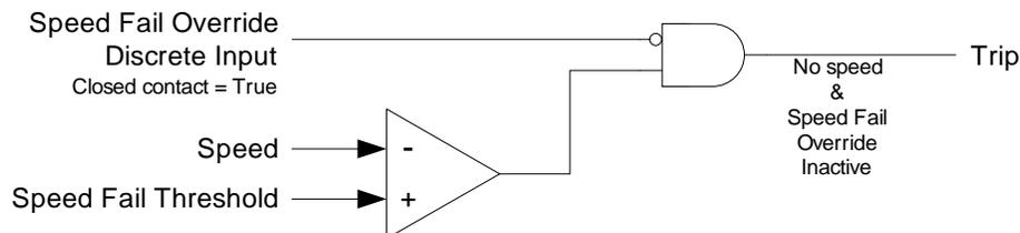
Figure 3-12. Speed Fail Trip Diagram
