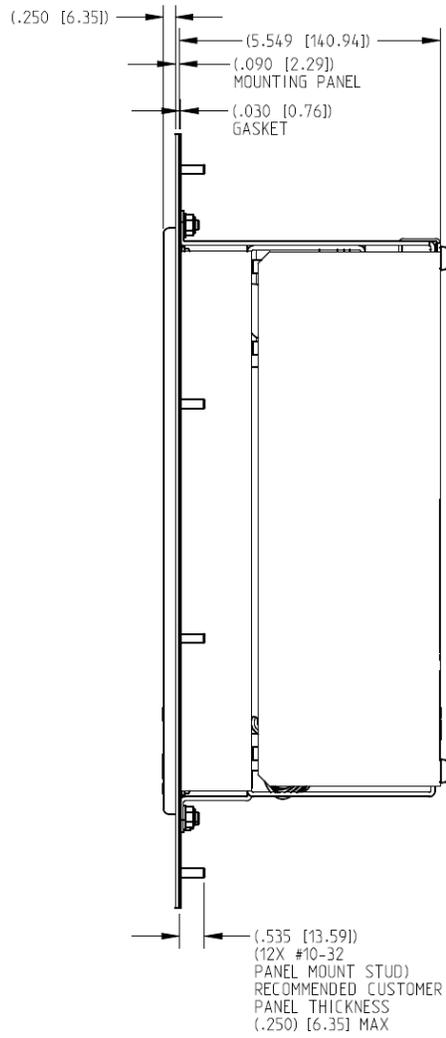
Figure 2-5b. Mounting Outline Diagram for Panel-Mount Models
