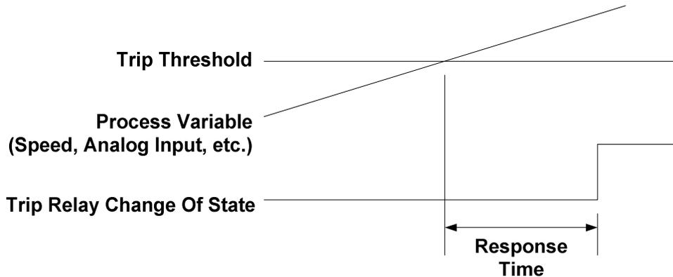
Figure 6-1. MicroNet Safety Module Response Time
