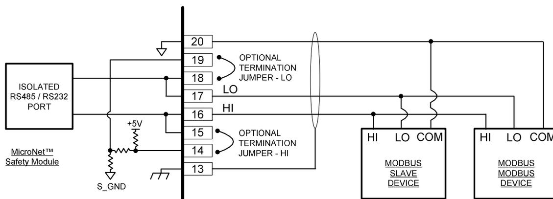
Figure 2-18b. Serial Com Port Interface Diagram —RS-485
