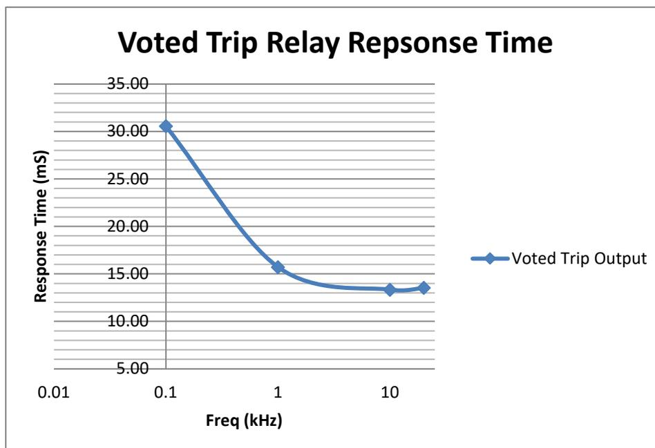
Figure 3-16. Voted Trip Relay Response Time (Typical) Graph
