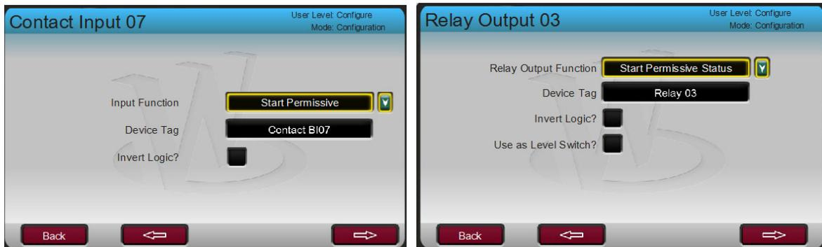
Figure I-11: Menu selections for DI and Relay Output
