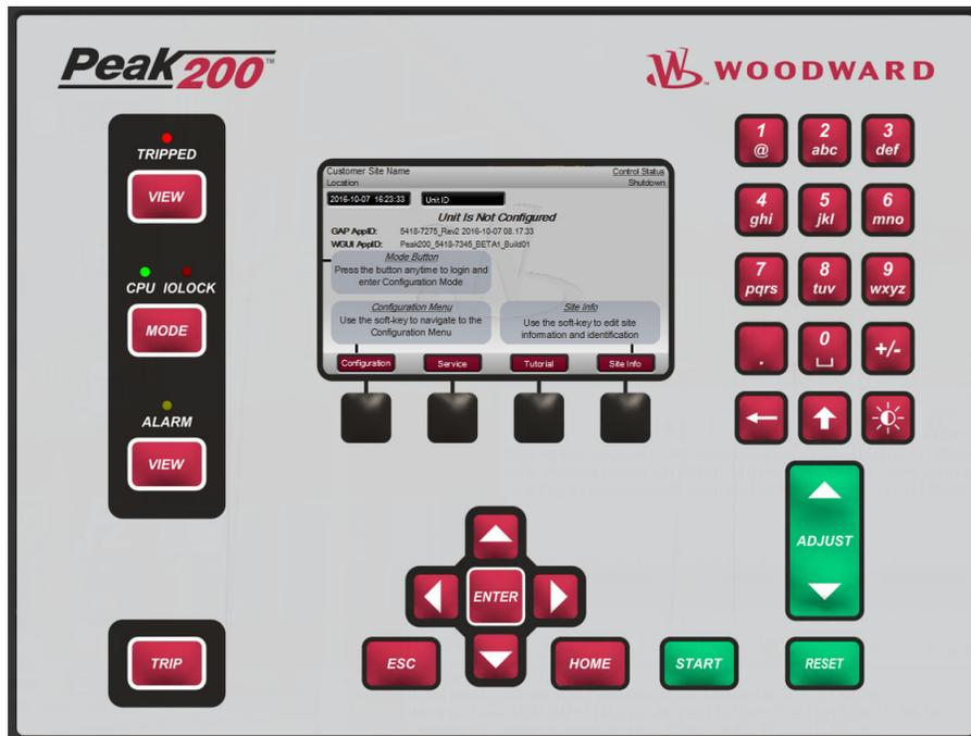
Figure 4-1. Initial HOME Screen (unit not configured)
