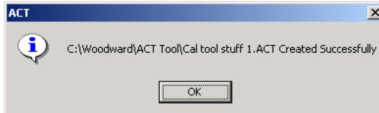
The file name in this message is the file selected in Step 2. ACT will save the calibration data to the designated file and display “Calibration Data Saved in File: ABCD.ACT” message (where ABCD is the name you entered in Step 2).
