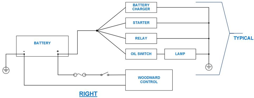
Figure 3-4. Correct Wiring to Power Supply Input
