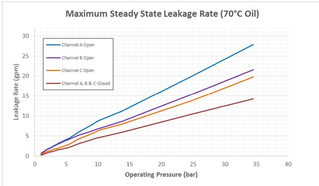
Figure 2-3. QuickTrip Steady State Leakage (70 °C hydraulic oil)
