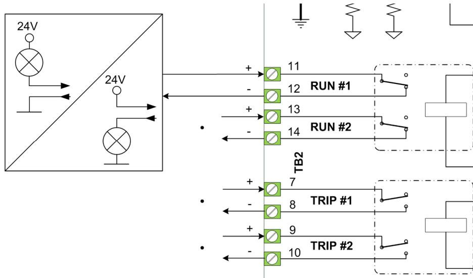
Figure 3-8. Feedback Output Connections
