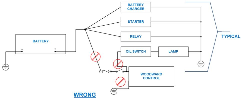
Figure 3-5. Example of Incorrect Wiring to Power Supply Input
