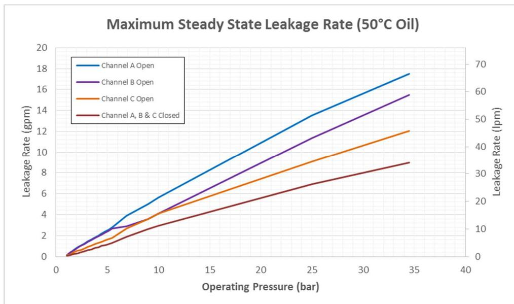
Figure 2-2. QuickTrip Steady State Leakage (50 °C hydraulic oil)
