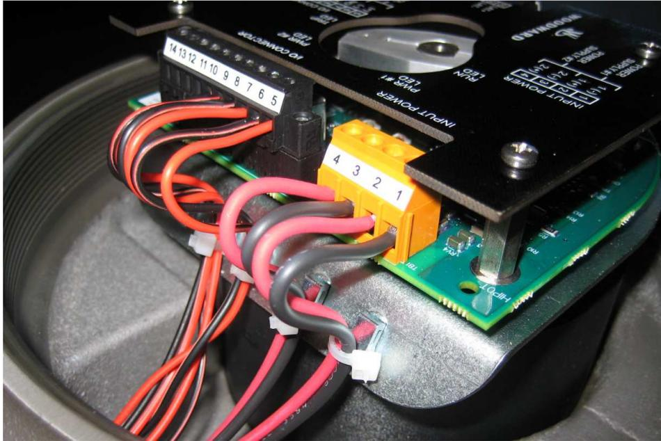
Figure 3-6. Recommended Wiring Strain Relief
