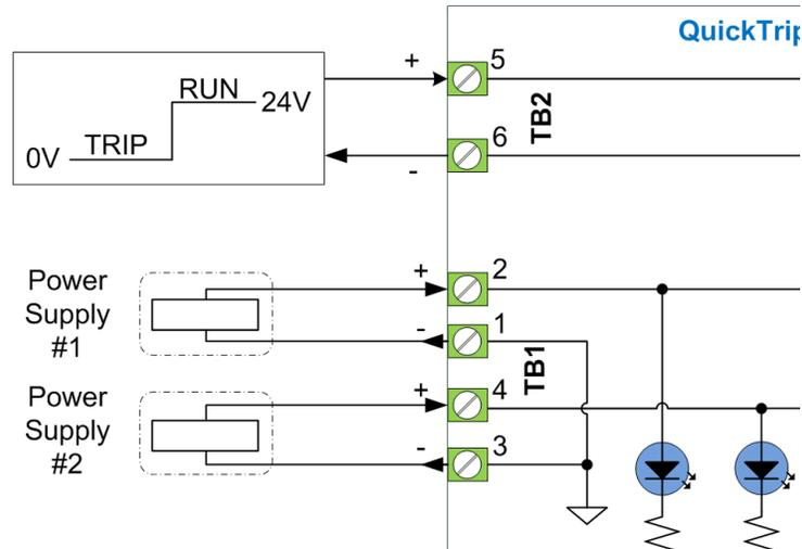
Figure 3-7. Control Input Connections
