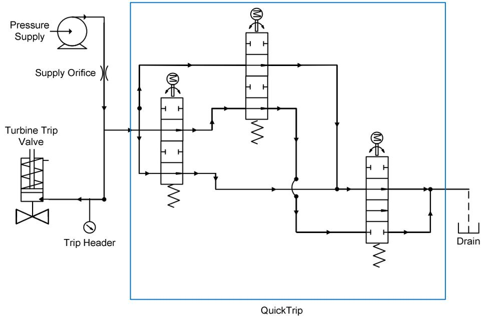
Figure 2-5. Hydraulic Schematic
