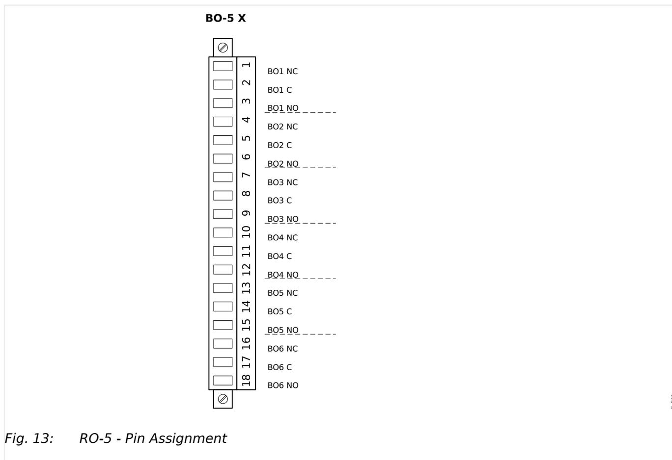
Fig. 13: RO-5 - Pin Assignment
