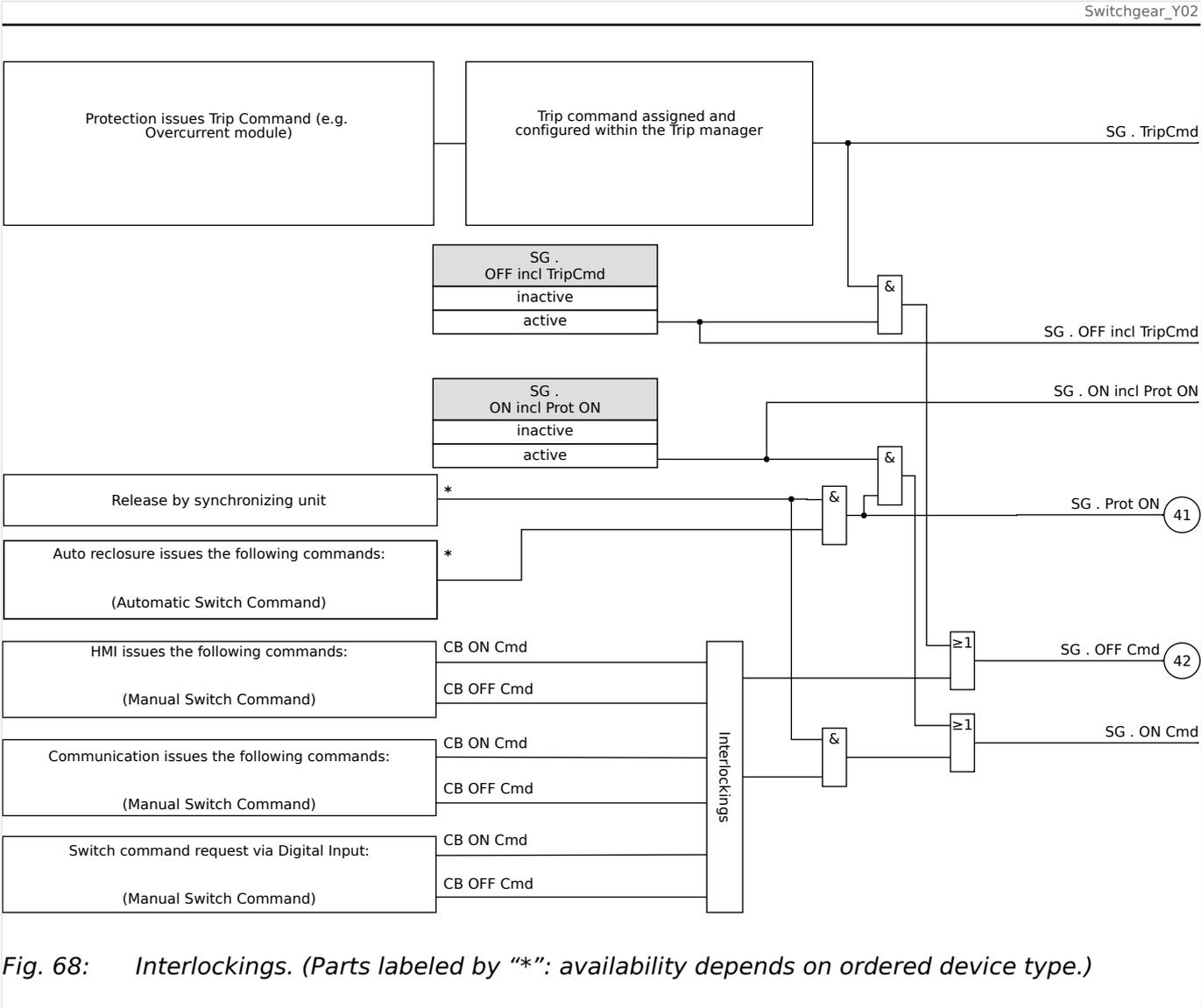
Fig. 68: Interlockings. (Parts labeled by “\*”: availability depends on ordered device type.)
