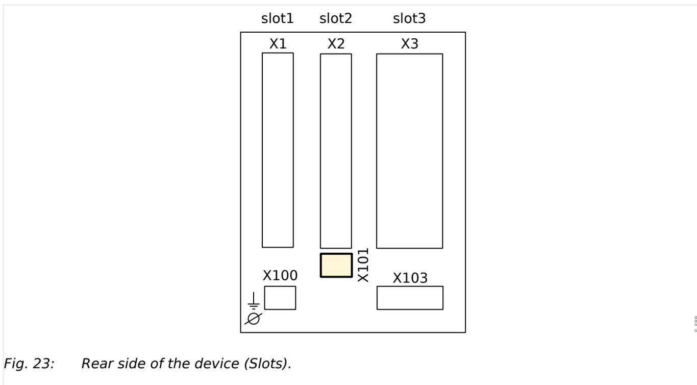
Fig. 23: Rear side of the device (Slots).
