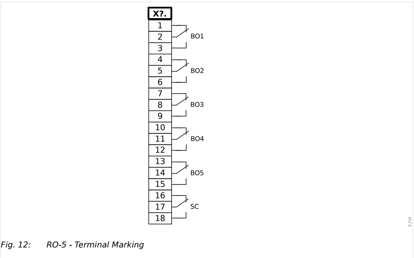
Fig. 12: RO-5 - Terminal Marking
