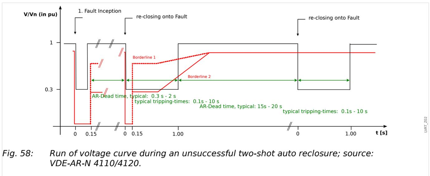
Fig. 58: Run of voltage curve during an unsuccessful two-shot auto reclosure; source: VDE-AR-N 4110/4120.
