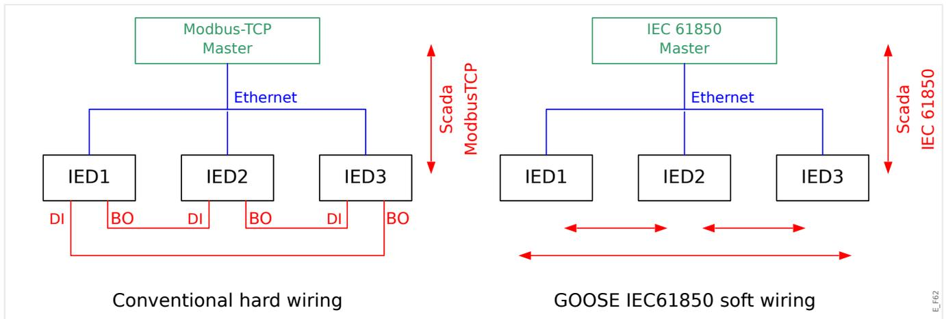
Commissioning steps for a conventional substation with modbus TCP environment:
