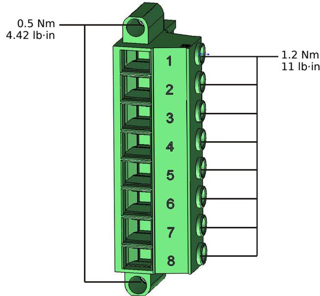
Fig. 81: Voltage measurement terminals of measuring card “TU” (➡ “2.5.1 TU - Voltage Measuring Inputs”).
