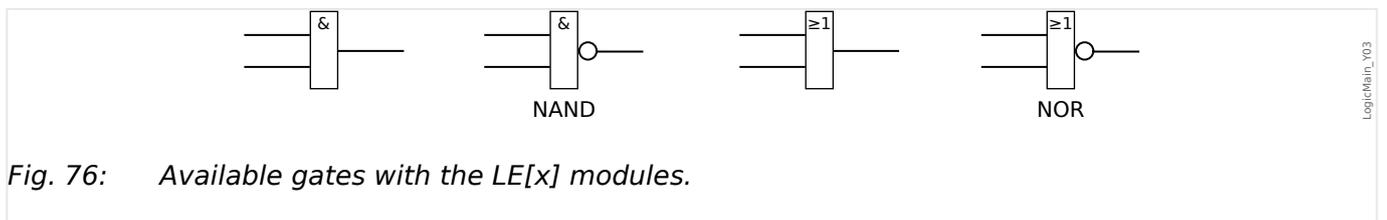
Fig. 76: Available gates with the LE[x] modules.
