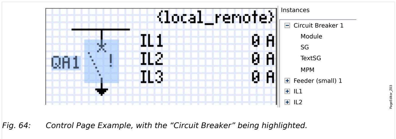
Fig. 64: Control Page Example, with the “Circuit Breaker” being highlighted.
