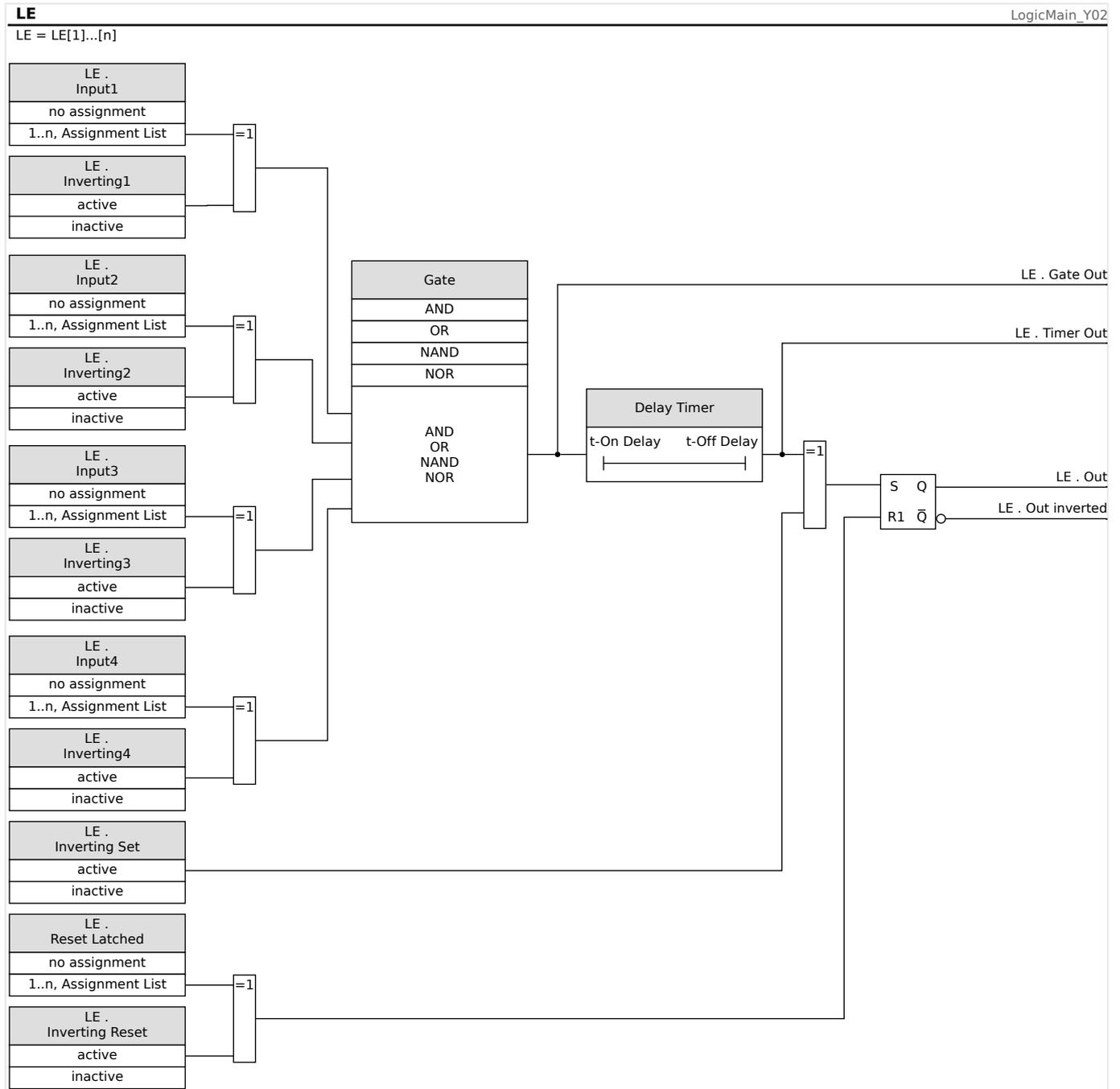
Fig. 75: Detailed Overview - Overall Logic Diagram.
