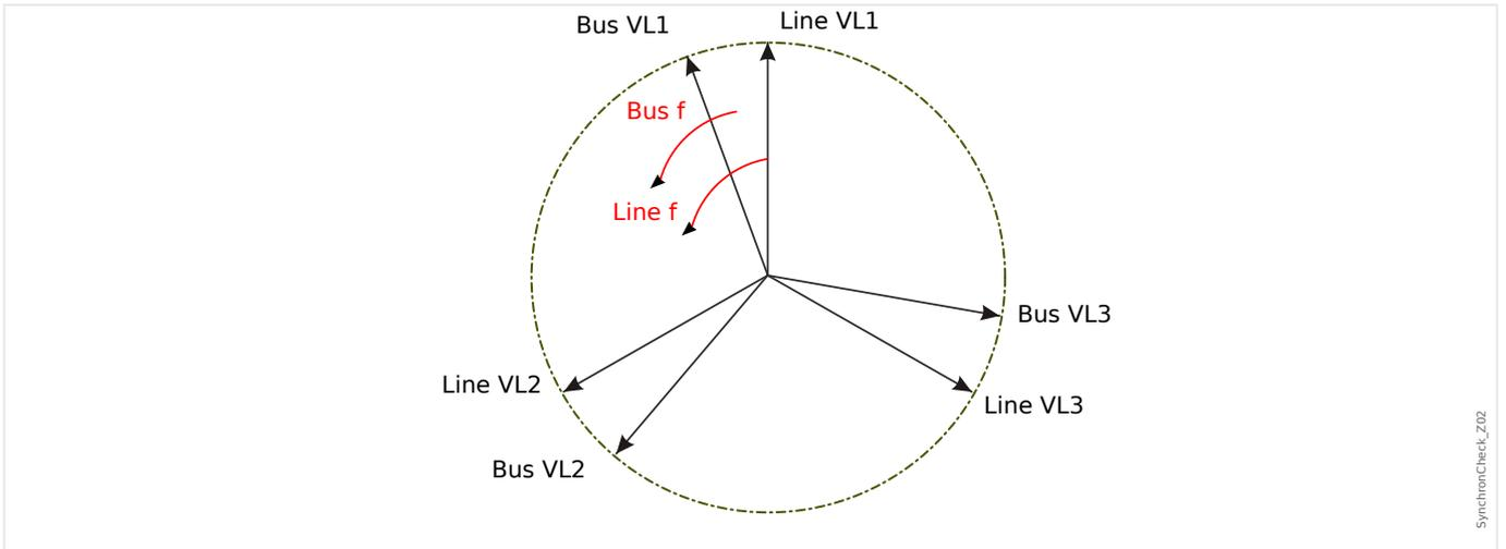
If the generator frequency  $f_{Bus}$  is not equal to the mains frequency  $f_{Line}$ , it results in a slip frequency  $\Delta F = |f_{Bus} - f_{Line}|$  between the two system frequencies.
