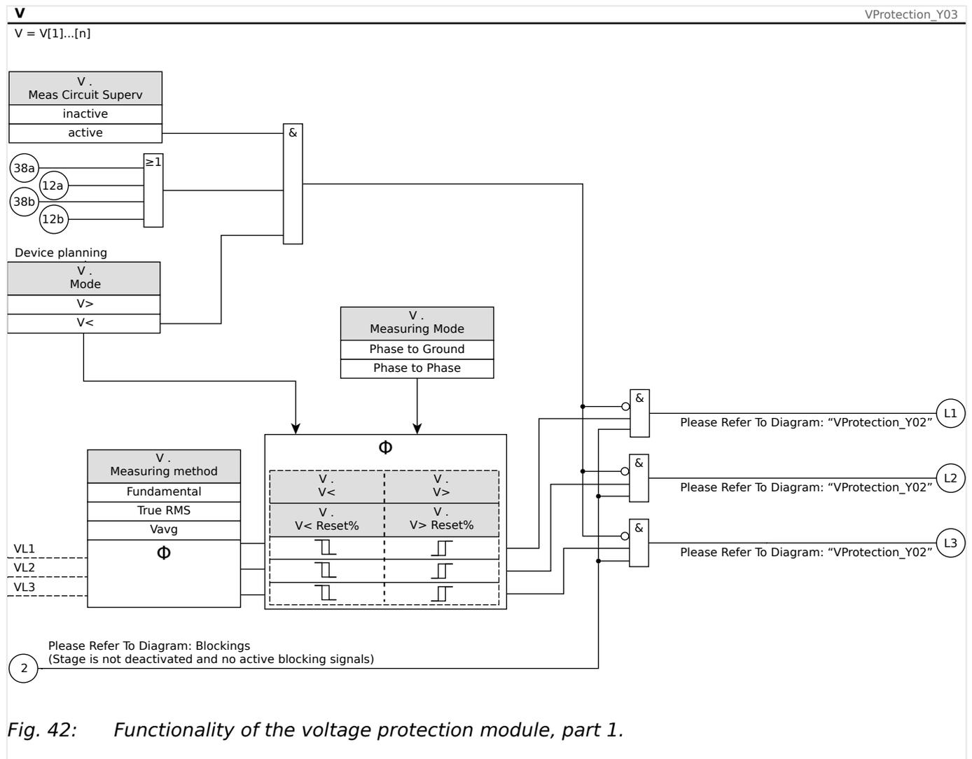
Fig. 42: Functionality of the voltage protection module, part 1.
