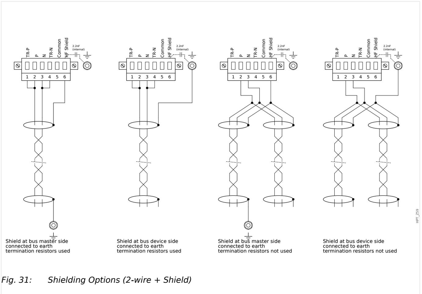
Fig. 31: Shielding Options (2-wire + Shield)
