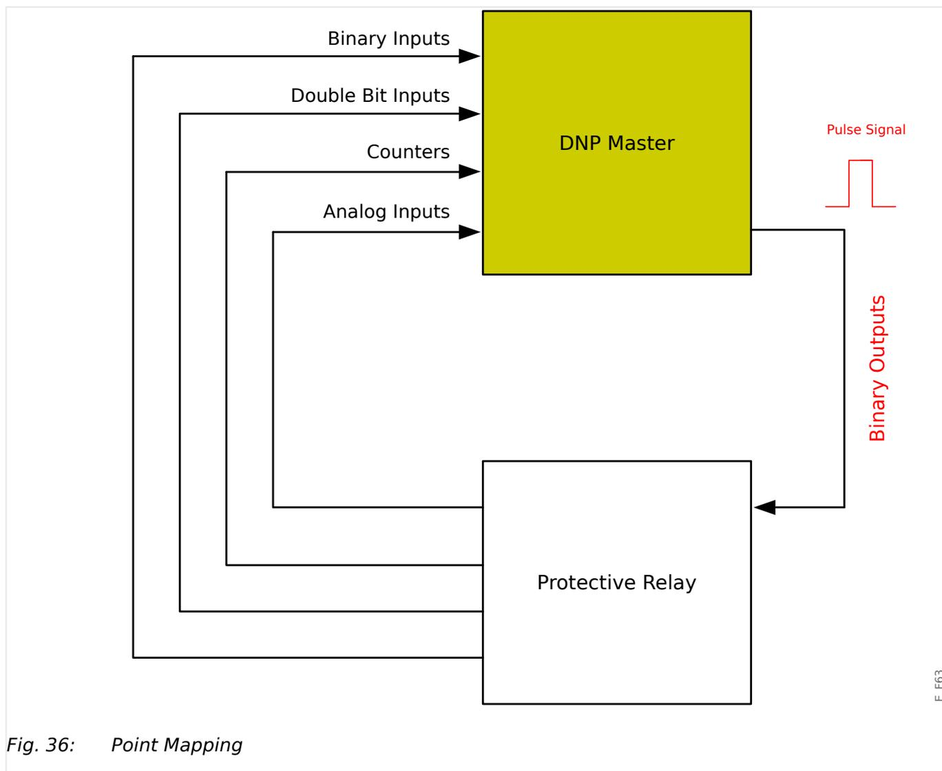
Fig. 36: Point Mapping
