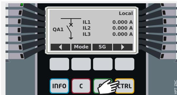
By pressing the »CTRL« key you enter a screen showing the single line, and you have direct access to related measuring values and control functions.
