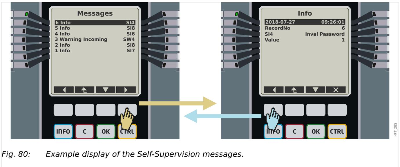
Fig. 80: Example display of the Self-Supervision messages.
