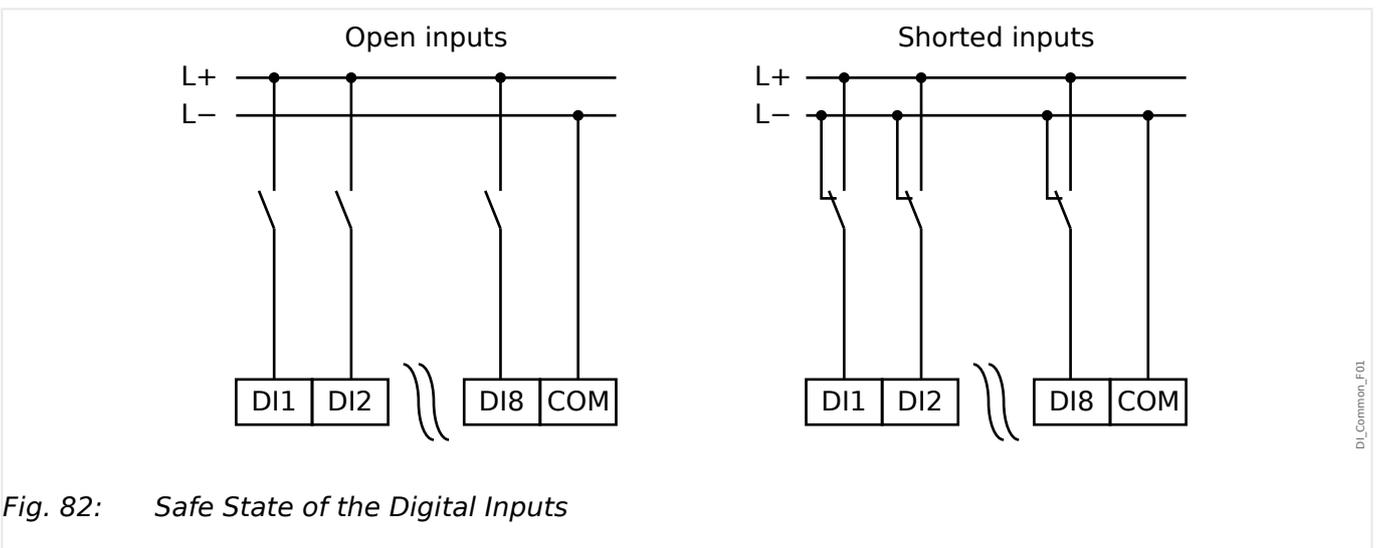
Fig. 82: Safe State of the Digital Inputs
