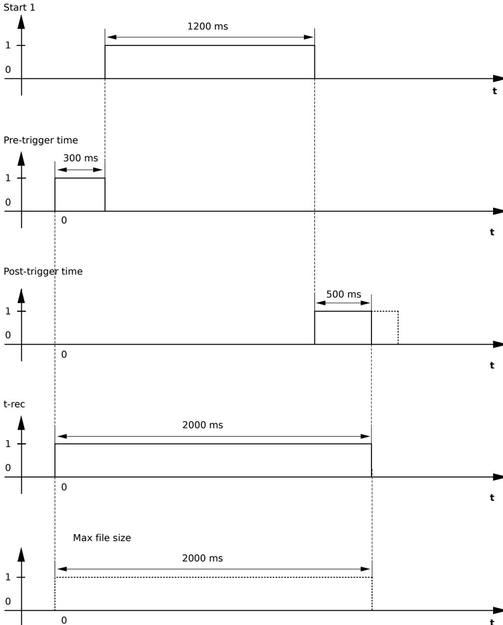
Fig. 71: Example Disturbance Recorder Timing Chart I
